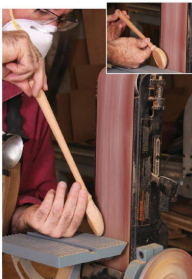
Sanding spin. Press the bowl against the sanding belt as you spin the handle with your fingers. Spinning the handle shapes the bowl from side to side, while varying the handle angle shapes it end to end. To shape the part of the bowl nearest the handle, rotate the spoon downward toward a more horizontal orientation (inset).
