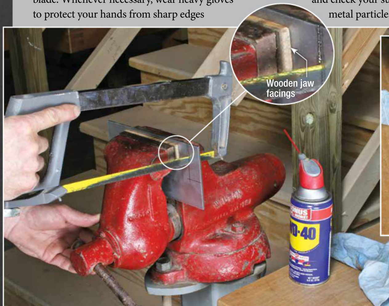
Magnets hold wooden facings to metalworking vise jaws.
