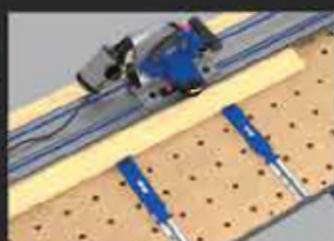
RIP BOARDS TO SIZE
