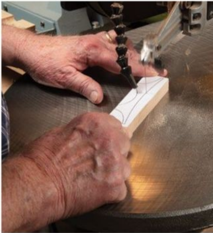
Scrollsaw the handle. With the pattern affixed to long stock for safe control, shape the handle, and then sand it.
