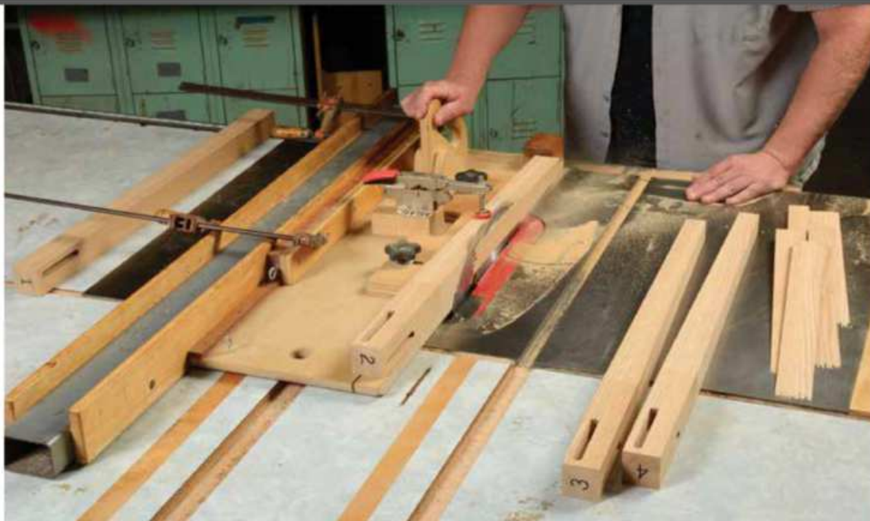
A jig for the job. A table saw tapering jig provides the best way to shape the legs. This version (see onlineExtras) was designed by woodworker and teacher Steve Latta.
