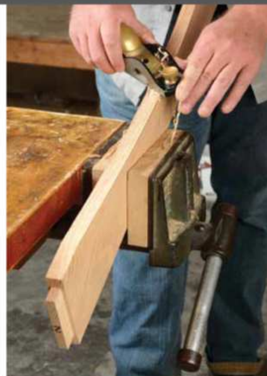
Just plane fair. A block plane does a great job of fairing the apron curve, as long as you skew it, which effectively shortens the sole enough for the blade to contact the concave edge.
