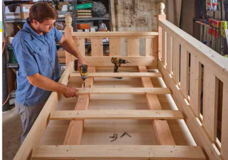
Screw in the seat slats. Evenly space out 5 or 6 slats across both beams, and then attach them with 1½" screws.
