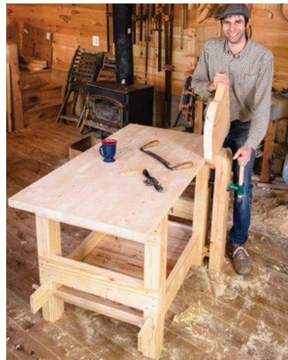
Weekend workbench. Make the leg vise from inexpensive hardware and the base from framing lumber.
