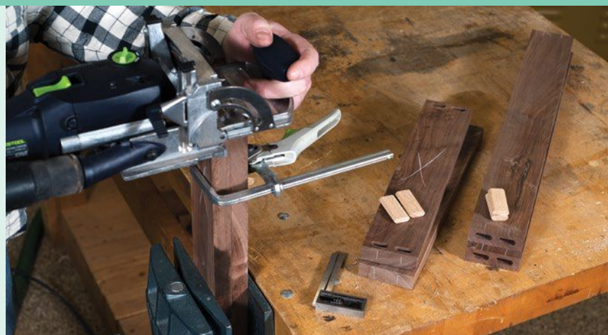
Domino the legs and rails. Clamping two legs together, inside faces out, simplifies layout and offers a wider base for the machine's fence.
