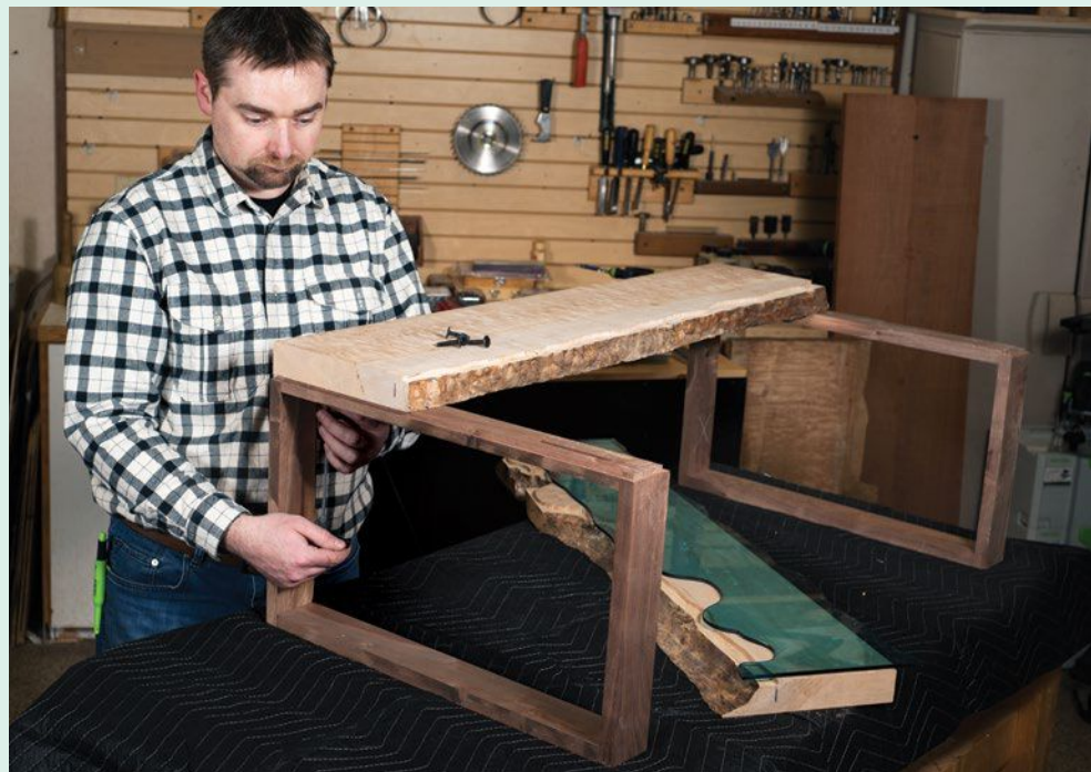
Making a final connection. Loosely bolt both top sections to the leg assemblies, set the glass in the rabbet, squeeze the top together, and then tighten the bolts.
