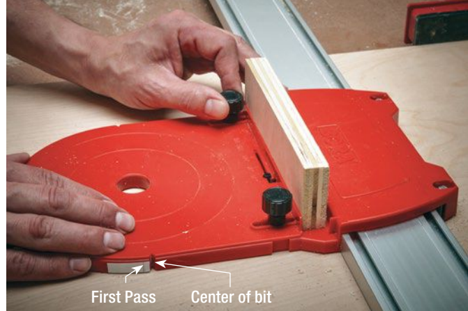
STEP 1: Set jig and rout the first pass.
