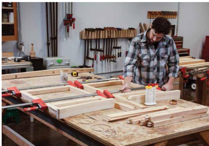
Side-by-side setup. Assembling the chairs in sections takes the pressure off you so that you can put more pressure on the joints that need it most. Have a few extra clamps and cauls at the ready in case you need to draw the armrests tight to the legs.
