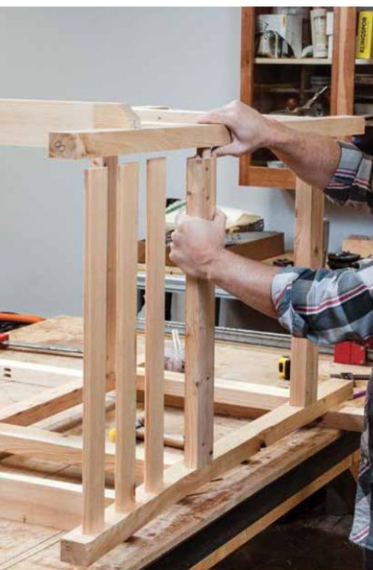
Gravity-assisted assembly. Fitting a multitude of tenons into their mating mortises is the trickiest part of the process. An extra pair of hands can help guide the top half into place.
