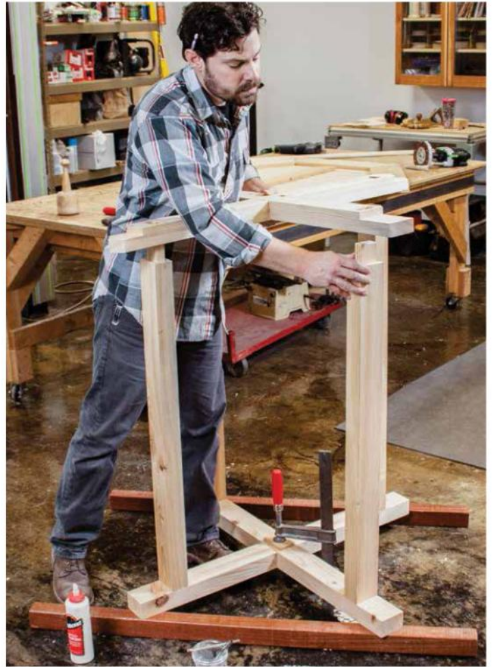
Stack, and then put the squeeze on. Insert the legs in the lower rails, and then attach the upper rails. The riser blocks provide necessary clearance for clamps.
