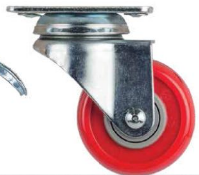
Swiveling caster with 2 \frac{1}{2} " wheel. 3 \frac{3}{8} " height, 2 \frac{3}{8} " x 2 \frac{1}{8} " mounting plate.
