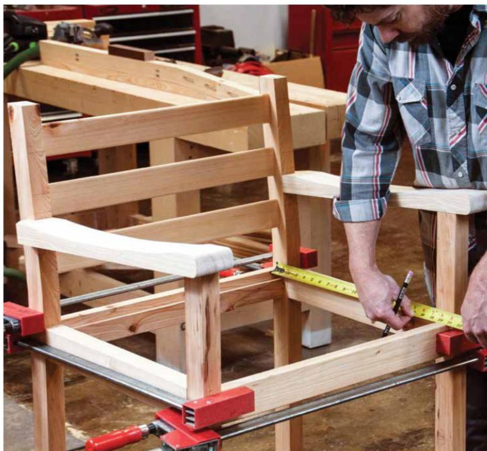
Make (and then take) a seat. I measure for the seat slats when the chair frame is together. Install the slats on top of the front and back cleats.
