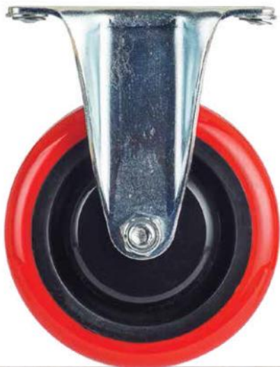
Fixed caster with 4" polyurethane wheel. 5" height, 2 \frac{3}{8} " x 3 \frac{3}{4} " mounting plate.
