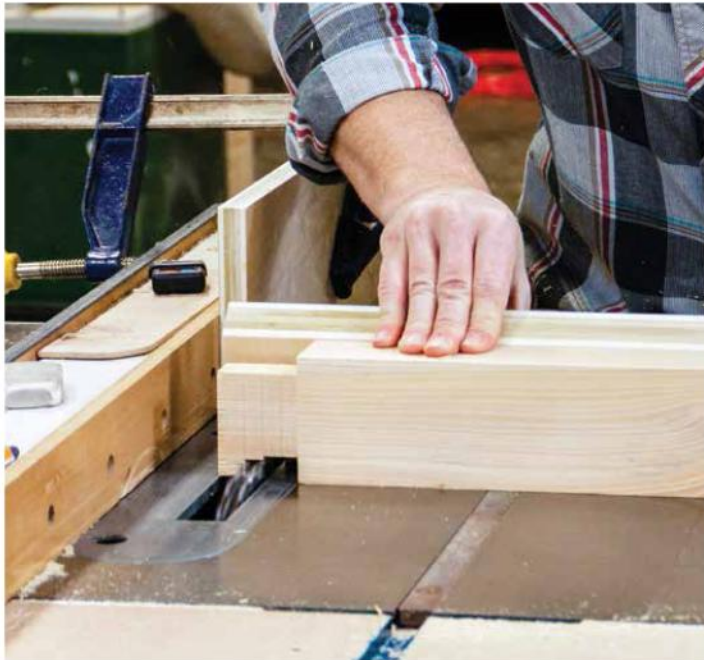
Tenon tamers. When cutting the leg tenons, use a stopblock and outfit your miter gauge with an auxiliary fence.
