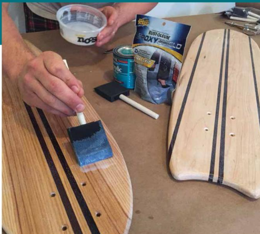
Pretty and gritty. A mixture of silicone grit and varnish creates a lovely, protective, non-skid finish that dries clear.
