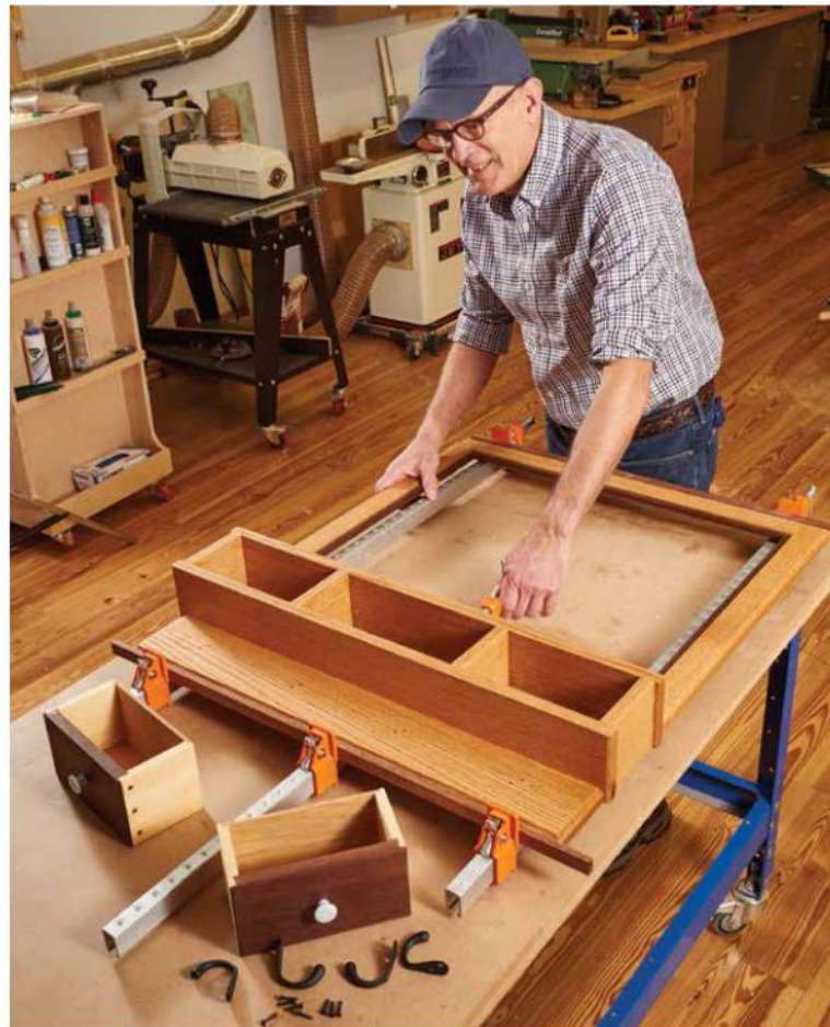
3 into 1. I used biscuit joints for strength and alignment when gluing the three subassemblies together.
