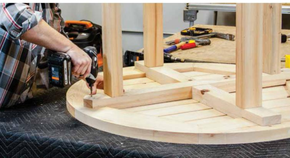
Attach the base to the top. Position the base assembly on the top and join the two with 2"-long stainless steel screws.
