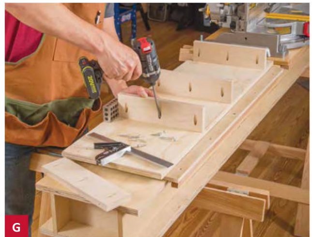
Pocket-screwing the risers to the underside of the saw table top ensures a smooth, seamless work surface.
