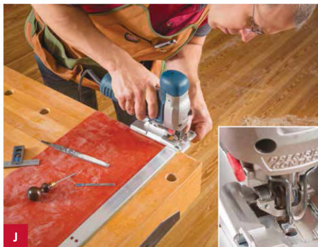
J To be safe, saw on the inside of your line and finish up with a file.
