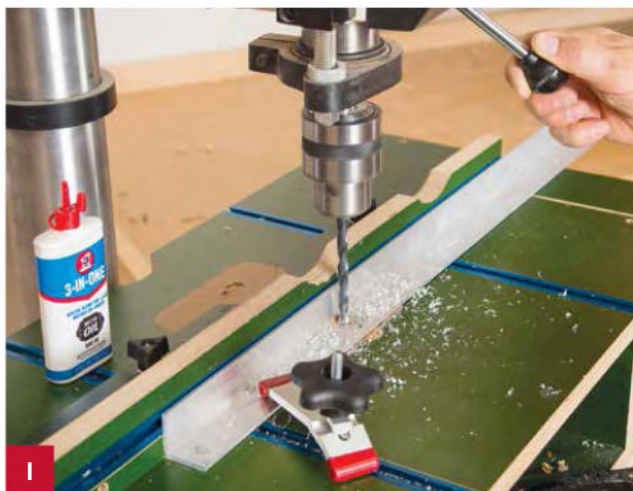
I Clamp the aluminum angle securely to your drill press table, and lubricate the bit for clean, straight holes.
