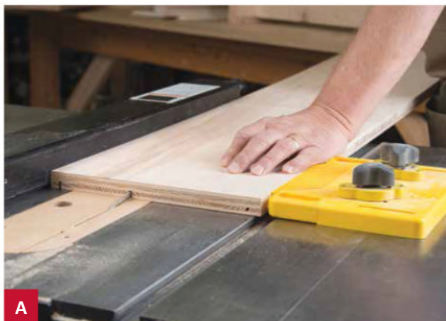
A Cut the runner grooves on the tablesaw with fence and featherboard.
