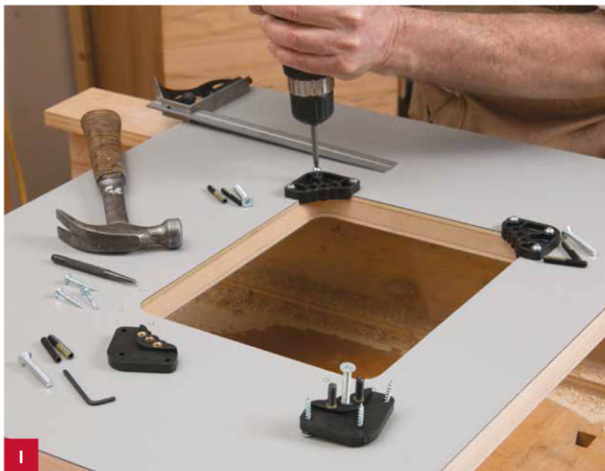
I Screw the insert plate levelers to the underside of the table top. Each is outfitted with two set screws for leveling the plate and one flathead screw for securing it down.
