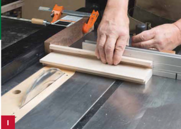
I After gluing the pull blank to the drawer front blank, crosscut the drawer fronts to final length at the tablesaw.
