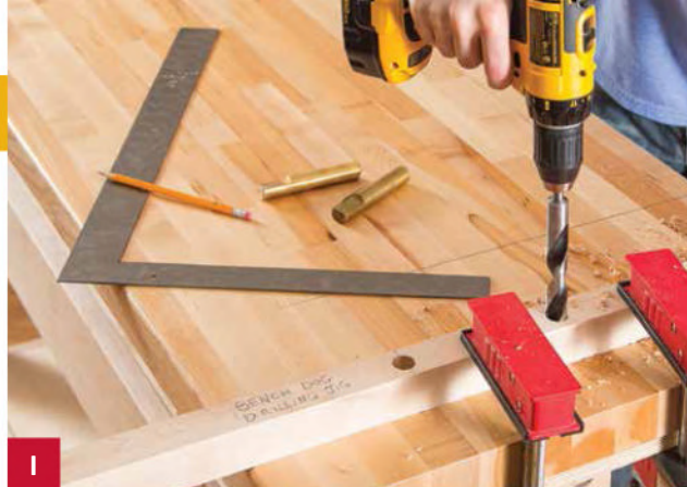
I Using your drilling jig and backer board to prevent tear-out, drill dog holes in your benchtop.
