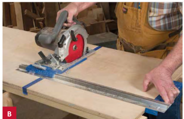
B Employ a circular saw guide or clamped-in-place straightedge to accurately crosscut the case parts to length.
