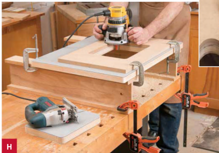
H Having roughed out the opening with a jigsaw, clamp the insert installation template in place, and rout to the template edges using a pattern-routing bit.
