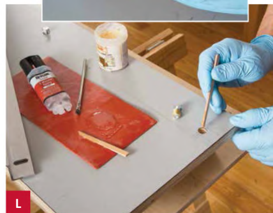
L Sinking threaded inserts into epoxy-filled holes is an easy way to ensure a tight fit without the risk of messing up the top of the insert.
