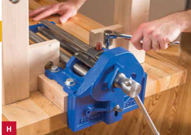
H Ratchet down the lag screws to firmly secure the vises in place.
