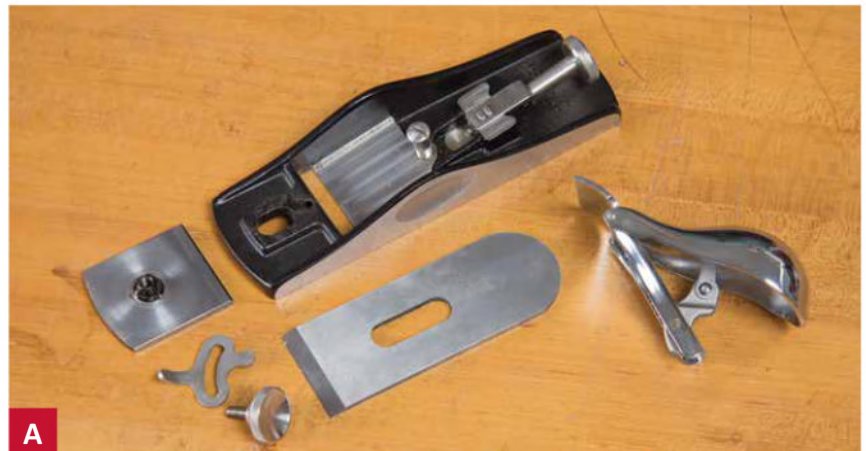
Figure 2c: Low Angle Block Plane with 38° blade. Good for planing difficult stock.
