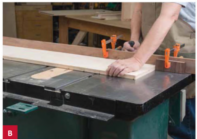
B Cut the dados for the drawer dividers using an auxiliary miter-gauge fence and stop.
