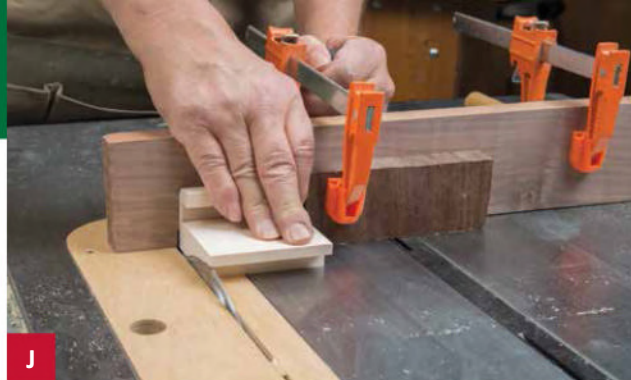
J Use a standard saw blade and a stop clamped to the auxiliary miter gauge fence to cut the rabbets in the ends of the drawer fronts. (Note: Half of the cuts are made with the miter gauge in the left-hand table slot, and the other half in the right-hand slot.)
