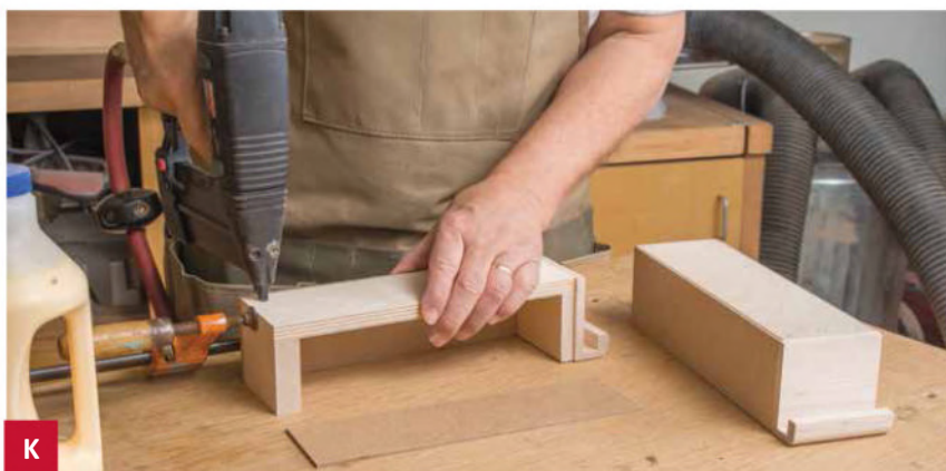
K Using a drawer side as a spacer to flush the drawer back, bottom, and front rabbeted edges, glue and pin-nail the parts together. Then permanently add the sides.
