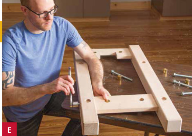
E Using the bench bolts, attach the rails and stretchers to the legs.
