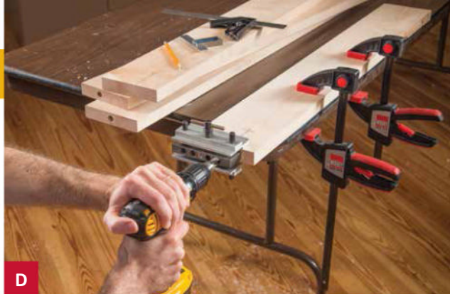
D Secure the doweling jig on the end of a stretcher or rail, aligned with the layout line. Bore a \frac{1}{2} " hole, 3" deep.
