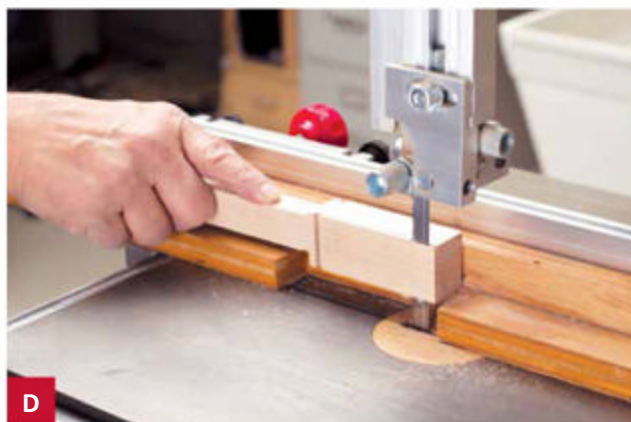
D Cut shoulders on the handle bottom, guiding off the fence and marked cutlines. Stop at the kerfs.
