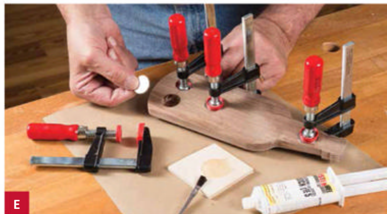
E Spread epoxy in the hole bottom, insert a magnet, and clamp it in place before moving to the next hole.
