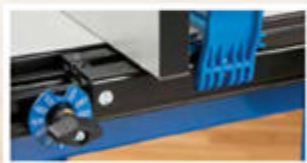
Fence Moved 0.015-Inches To "015" Setting
