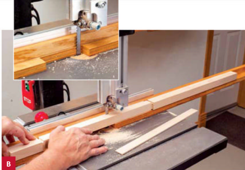
B Bandsaw between the radii on each handle edge by moving the jig and handle along the saw's fence to remove the waste.
