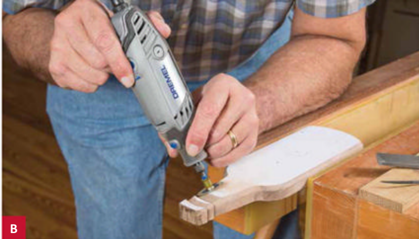
B Carefully disc-sand or file the neck to round over the edges leading into the collar. Round over the edges of the collar and cap.
