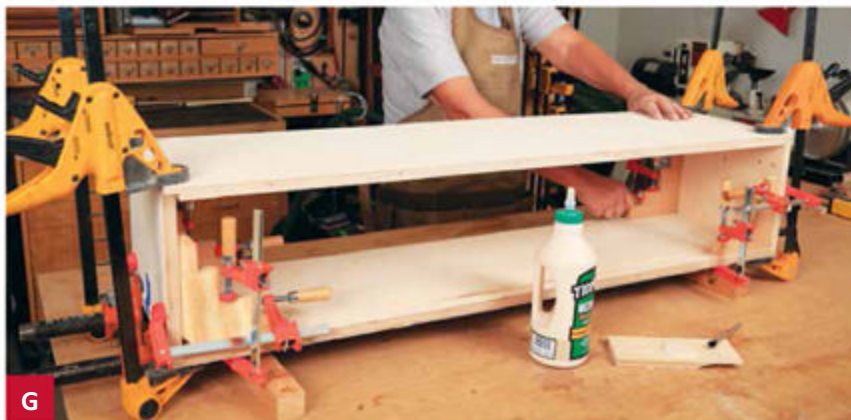
G Clamp square angle braces in the box corners when gluing and assembling the box ends and sides.
