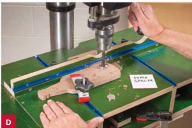
D Clamp the bottle in place to prevent it from moving during the drilling operation.
