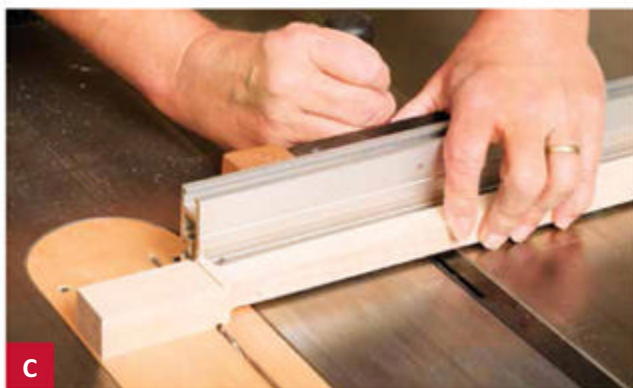
C Use a miter gauge for support when cutting the kerfs on opposite surfaces of the bottom ends of the handles for the mallet heads to seat against.
