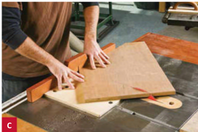
C Clamp or nail the deck to a crosscut sled, and saw the second deck edge 90° to the first.
