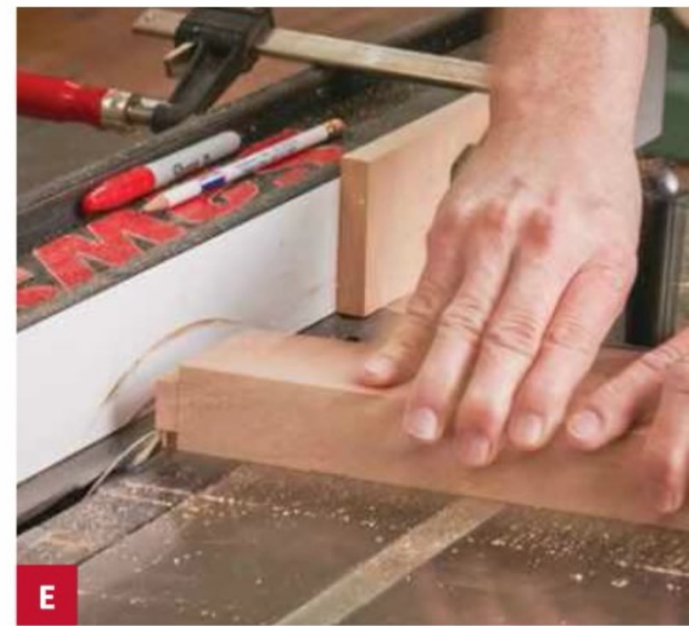
E Set the miter gauge to 10°, and cut the angled tenons on the armrest ends.
