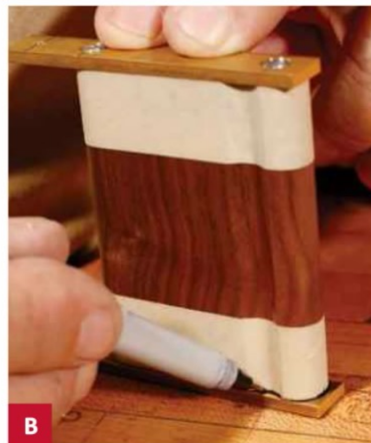
B With the side blanks temporarily screwed to the handle, use a fine-tipped marker to trace the handle's shape onto the blanks.
