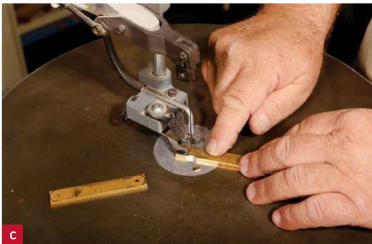
C Hold the brass side blank firmly to cut the coves and rounded ends while following the cutlines.
