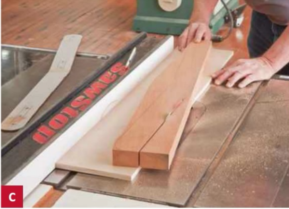
C Using a plywood sled to trim the front edges of the rear legs ensures a straight, square edge.
