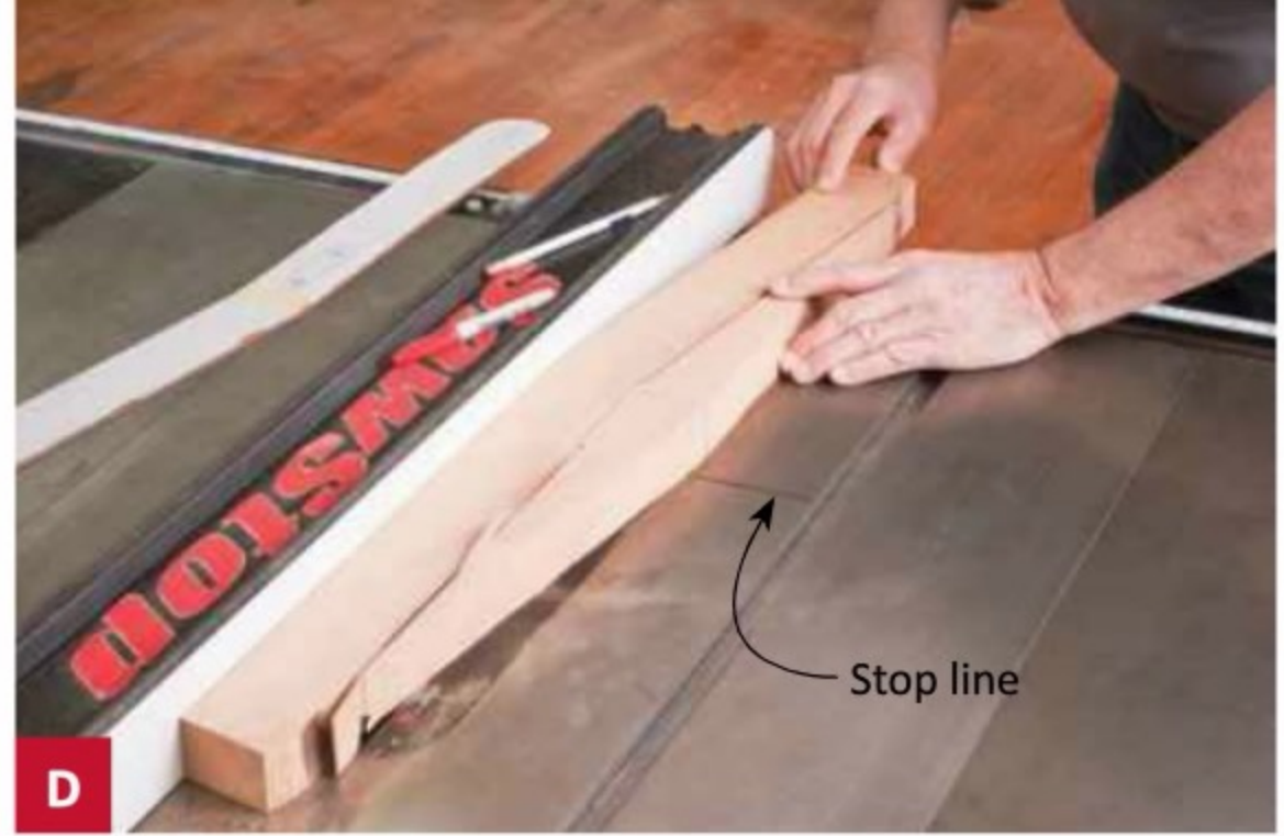
D Keep the leg's front edge against the fence when ripping the outside edges. Pay attention to the stop line to avoid overcutting.
