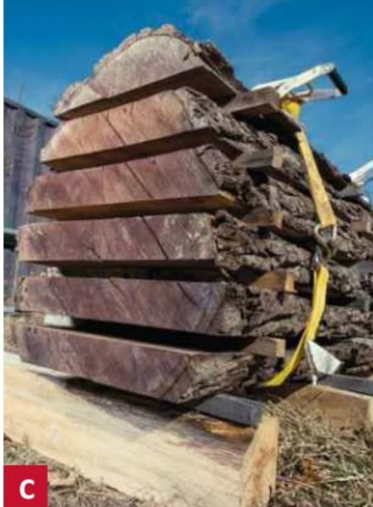
C Strap pressure and properly placed stickers can restrain boards in a stack from warping.
