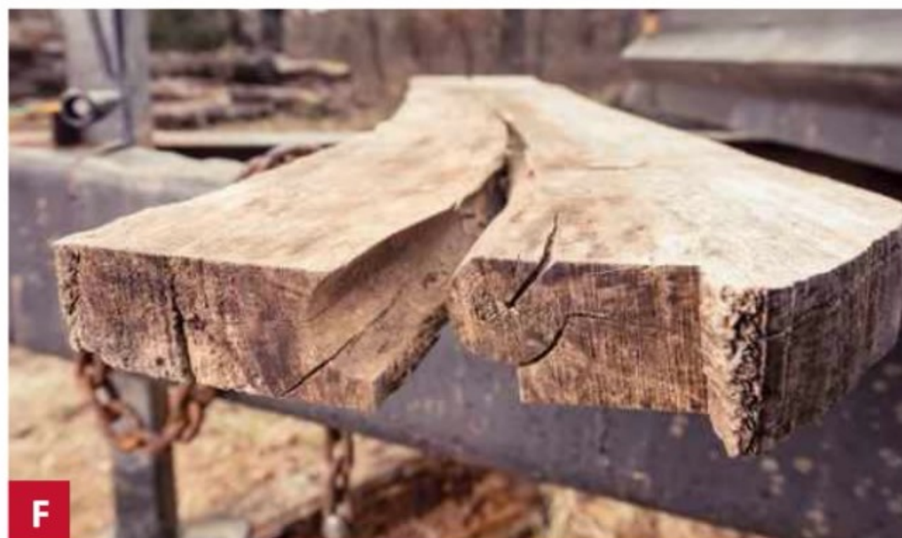
F The off-centered pith in this board caused it to both crook and crack.
