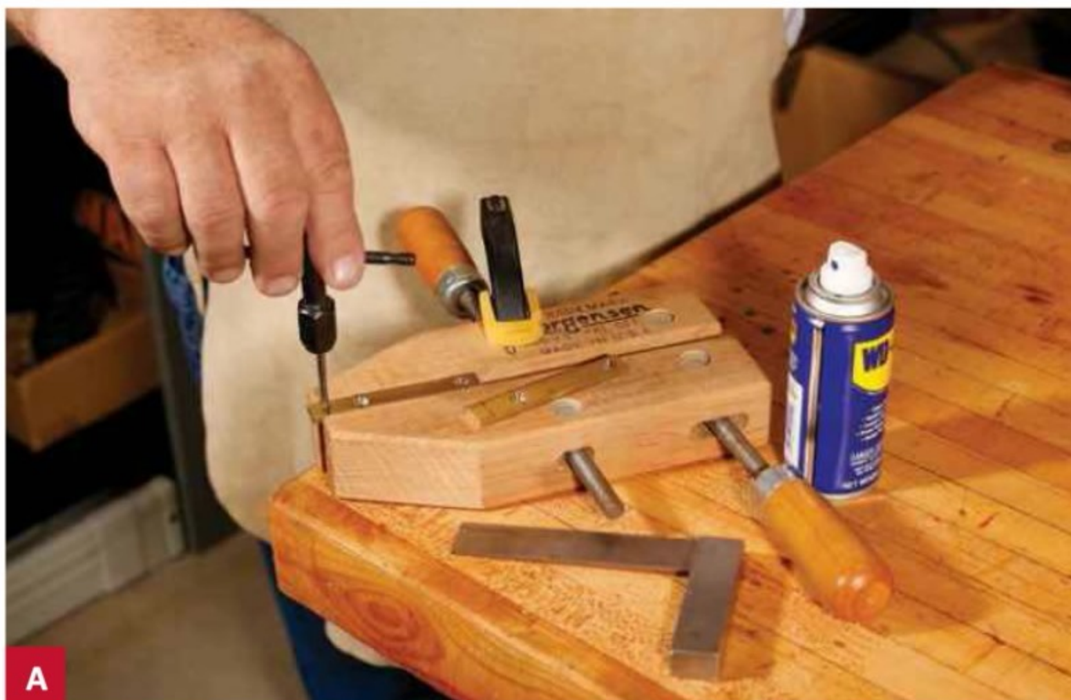
A With the side held in the bench vise and the tap square to its face, cut the hole threads, lubricating as needed with cutting oil.
