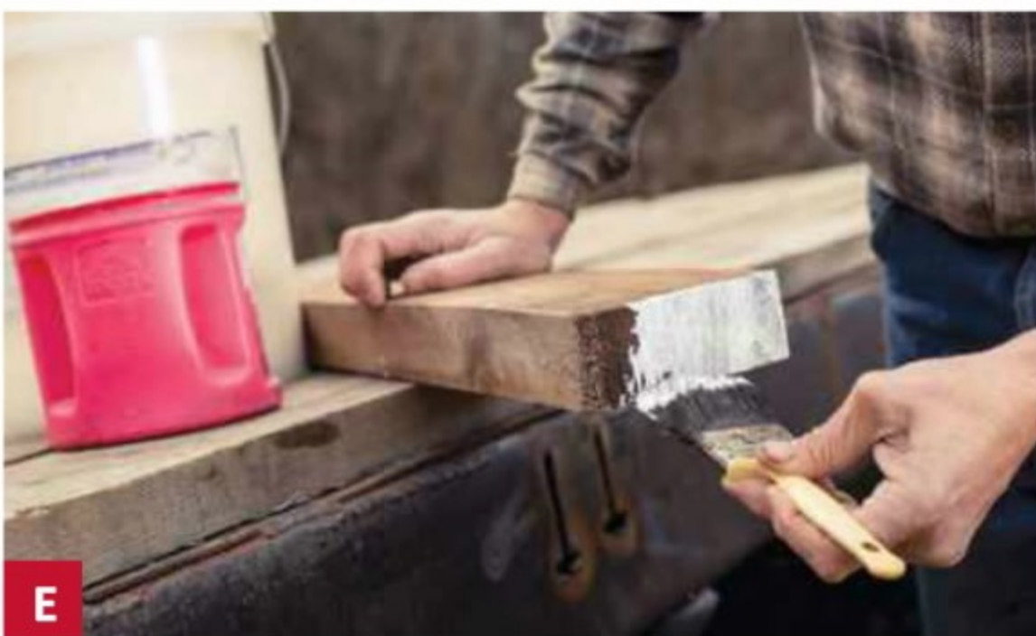
E Apply several coats of latex paint or “Anchorseal” on board ends soon after the tree has been cut to reduce end checking.
