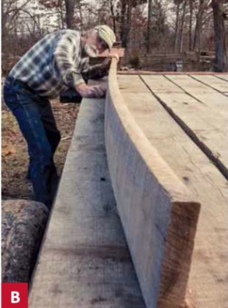
B Drying boards can bow from one end to the other if left unrestrained.
