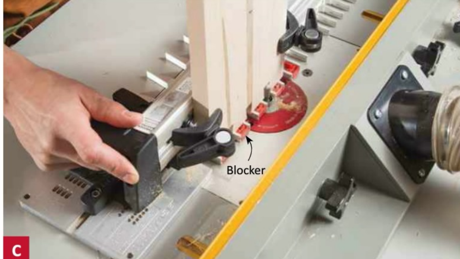
The snap-in plastic blockers prevent routing between the wrong set of template fingers. Locating a router table fence dust port nearby extracts most of the dust.
