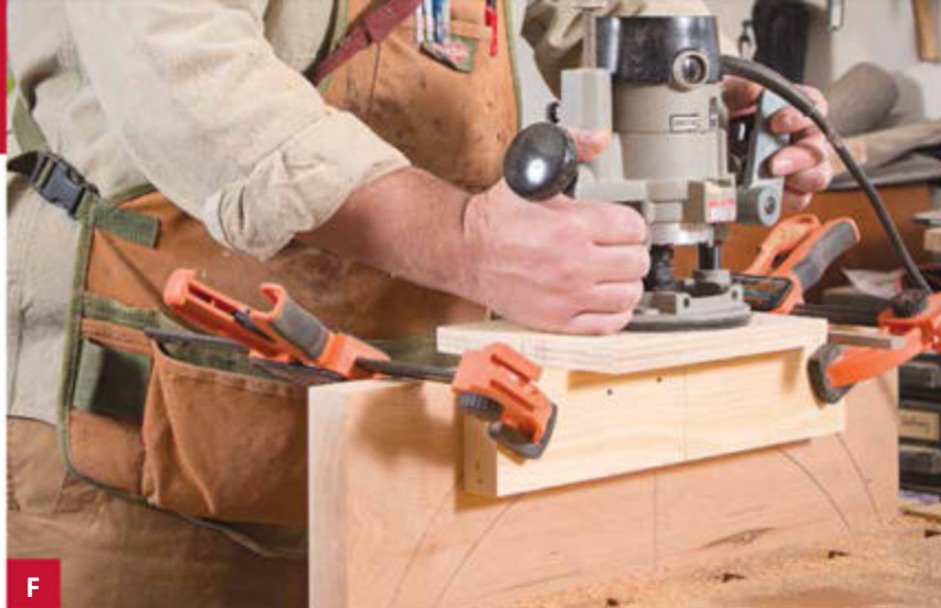
Register the mortising jig on the upper edge of the foot blank and rout the mortise.
