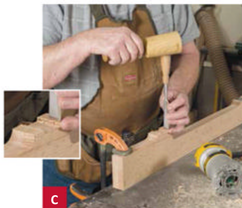
Rout the mortise to the thickness of the table leaf hardware; trim to the layout lines with a sharp chisel.
