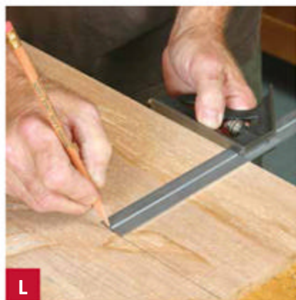
L A combo square has a longer reach than most marking gauges, allowing layout of parallel lines at a greater distance from the board edge.
