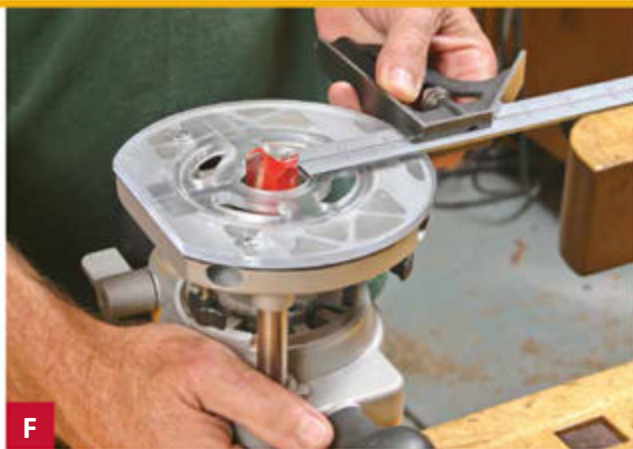
F A combo square can take a measurement of a router base-to-bit distance as reference for setting fences and jigs for dado and groove work.
