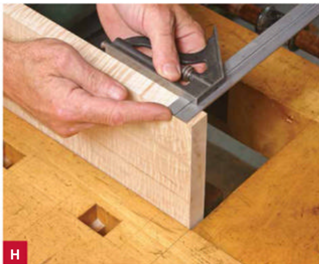
H To check a board for consistent thickness, extend the blade to one corner, and then compare at the other corners, feeling for flush with your finger.
