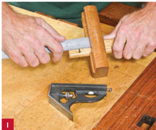
I Set up a marking gauge by butting the rule against the gauge's fence and aligning the knife or pin to the desired increment.
