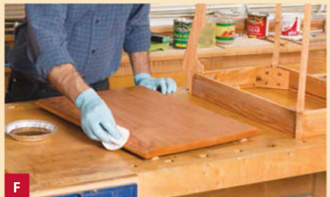
F Apply finish to edges first, using light pressure, and wiping on just enough varnish to coat them without causing dripping on the underside.
