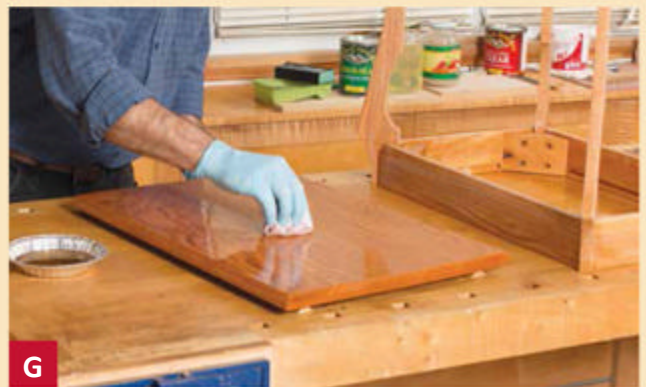
G Cover the surface thoroughly, using light pressure to transfer the varnish to the work, slightly overlapping previous swaths.
