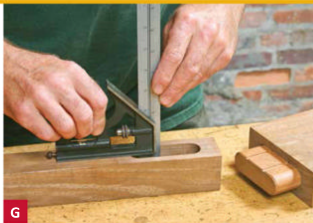
G Check a mortise's depth by holding the head on the work while sliding the rule into the recess until it bottoms out. Lock the rule, and then read the distance.
