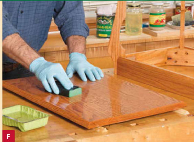
E Wet-sand the dried second coat using 600-grit paper. Notice here the second-coat sheen already starting to build on the unsanded right-hand side.
