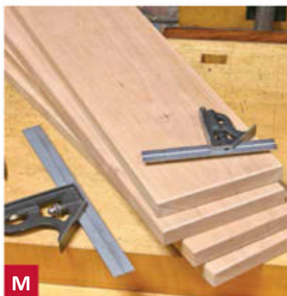
M Set two squares to key dimensions for locating hardware on a series of identically sized drawer fronts or other parts.
