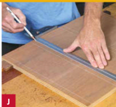
J A 24" accessory ruler makes laying out and squaring dadoes and other long joints easy and accurate.
