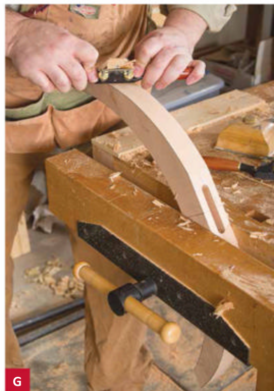
A spokeshave will quickly remove saw marks on the feet, although you could use a power sander to do the job instead.
