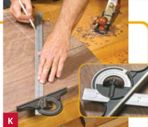
K Precise angles are a snap to lay out with a protractor head. The easy-to-read scale on this Starrett model is marked in 1° increments (inset).
