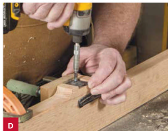
Use a block to flush the hardware with the edge of the oval support; drive the mounting screws.
