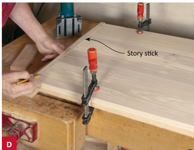
D Use a story stick to mark the biscuit locations on mating pieces and to establish consistent biscuit spacing from part to part.
