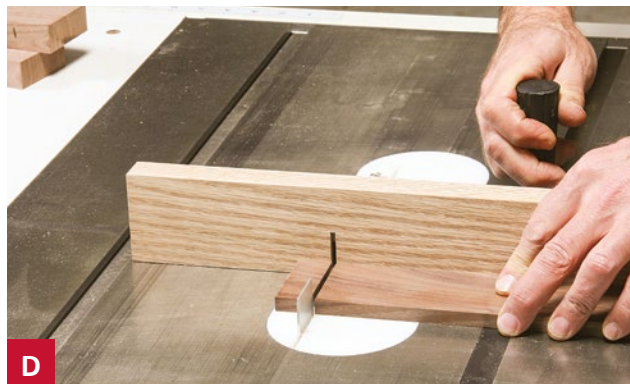
D An auxiliary miter gauge fence that extends past the blade will safely carry small offcuts completely past the blade.
