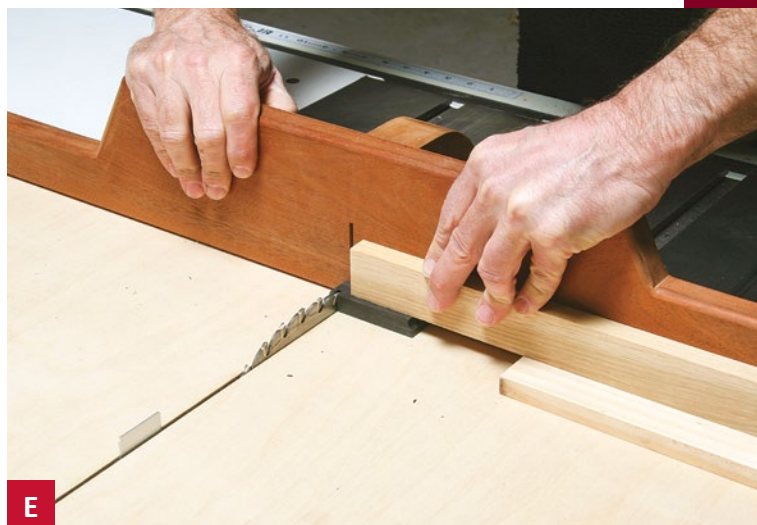
E This small ebony workpiece is held down on a crosscut sled using a stick that bridges over from a scrap riser.
