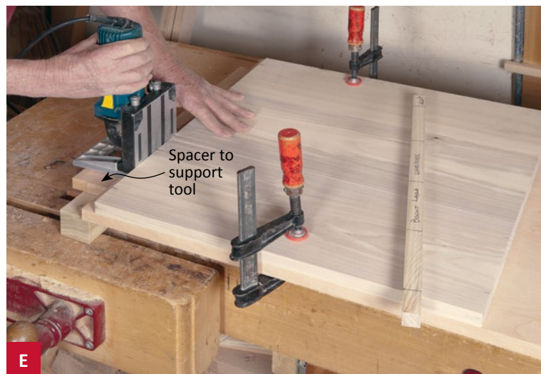
E With the biscuit cutter aligned with the marks, cut slots on the mating parts.
