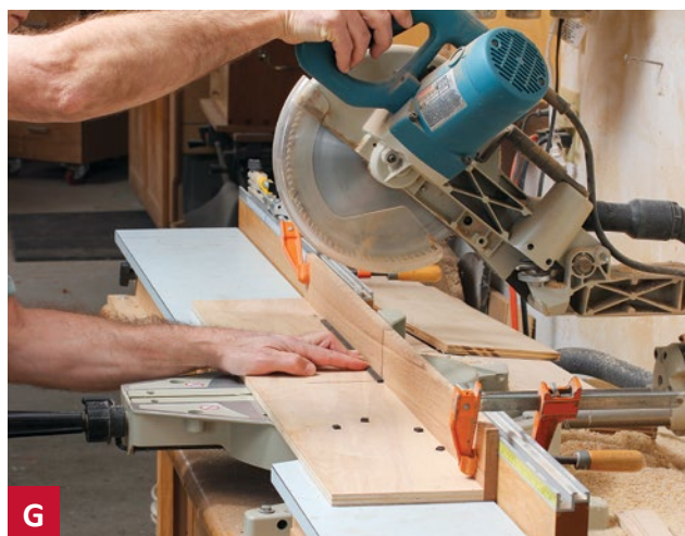
G An auxiliary deck on a power mitersaw makes for cleaner cuts and prevents "keeper" offcuts from being thrown backwards by the blade.
