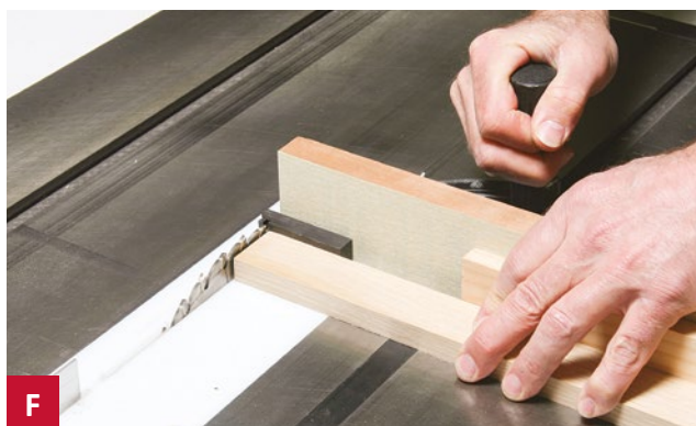
F Bridge-clamping can also be done against an auxiliary miter gauge fence that extends all the way to the blade.
