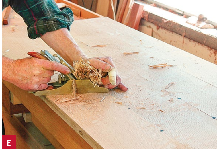
E Working diagonally across the panel, use a #4 bench plane to quickly level the boards, or go with a belt-sander for similar results.
