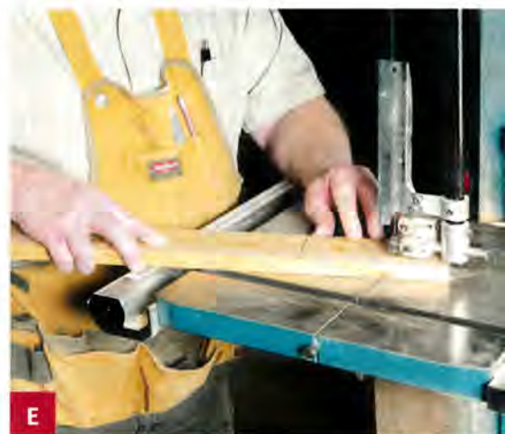
Keep fingers out of harm's way by laying out the corbels on a longer workpiece to safely cut the curves.
