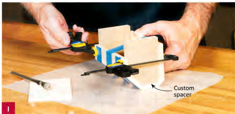
Clamp the taped and glued bucket parts to the custom spacers to create the bucket shape.
