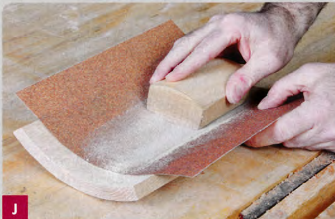
J To refine the shape of a complementary sanding block, line the workpiece curve with sandpaper and rub the block against it.
