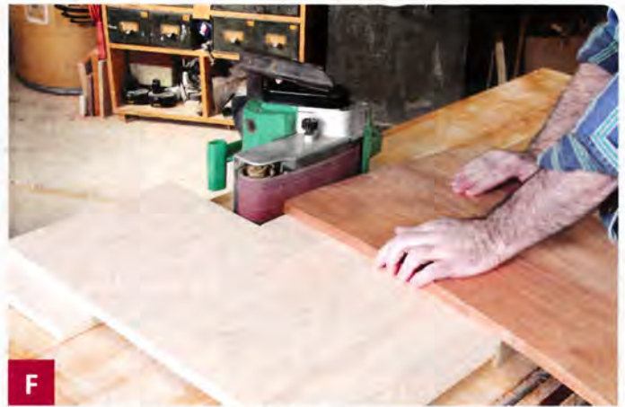
F A portable belt sander clamped sideways next to a raised platform on a bench becomes a stationary sander for smoothing both concave and convex curves.
