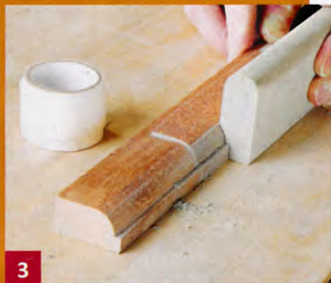
Line a profile sample with sandpaper, and then rub a block against it to create a complementary sanding block.
