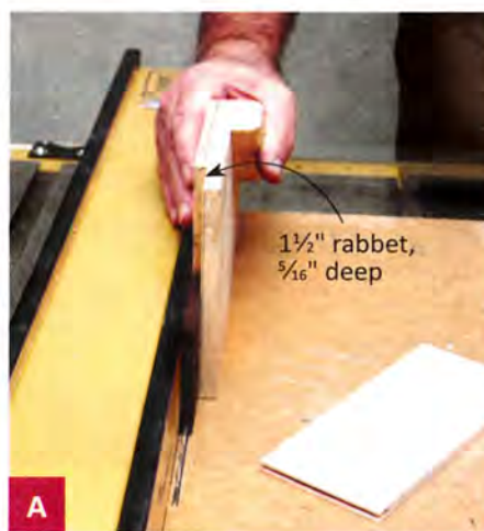
Use a rabbeted pushblock to safely trap the blank against the fence when making the kerf cuts.
