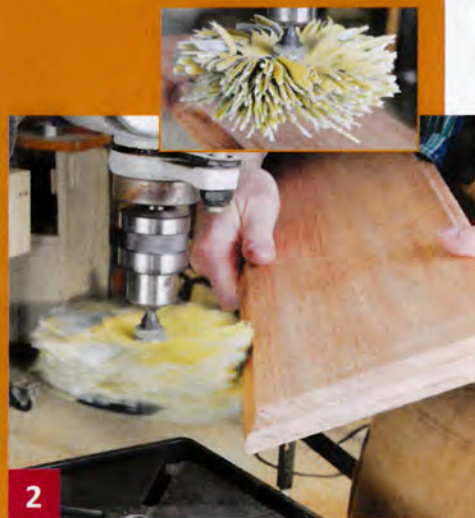
A sanding mop smooths molding profiles in much the same way brushes in an automatic car wash clean your vehicle.
