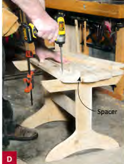
After installing the center slat, use a pair of spacers to locate remaining slats, securing them with screws.
