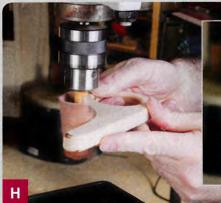
H Insert a scrap of sandpaper into a slotted dowel to turn your drill press into a sort of mini drum sander.
