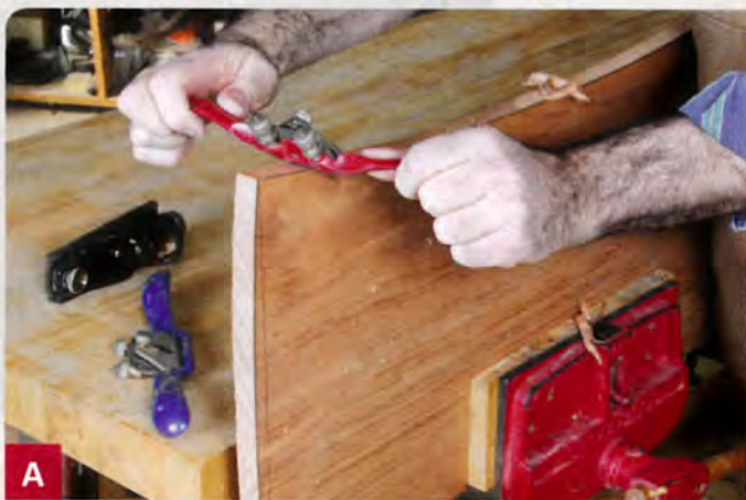
A Flat-sole spokeshaves work well for convex curves, while curved-sole models are better suited to concave shapes.
