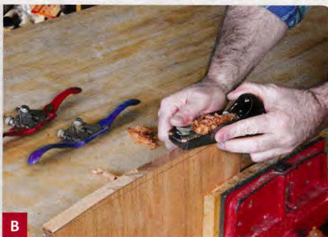
B On convex curves, a block plane will serve to remove saw marks while fairing away lumps and valleys.
