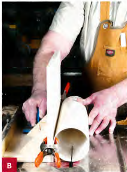
B Clamp each shutter pipe to a right-angle jig to hold it firmly and then rip along its length.
