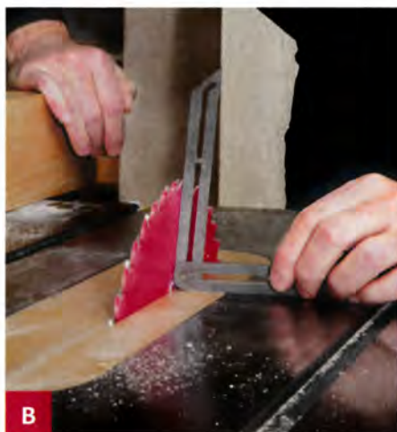
B Place the gauge between the saw teeth, and adjust the bevel angle until both blades touch.
