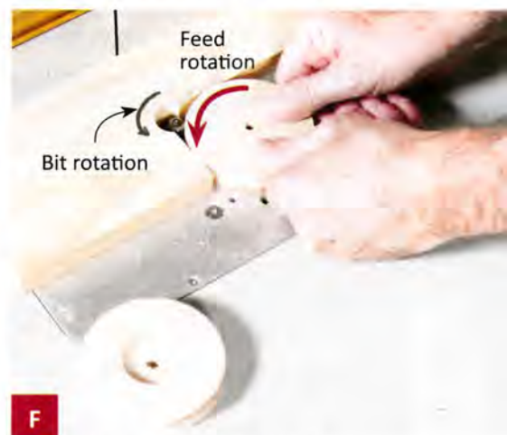
F Fit the tire half—outside face down—in the L-shaped jig and round over the edge as shown.
