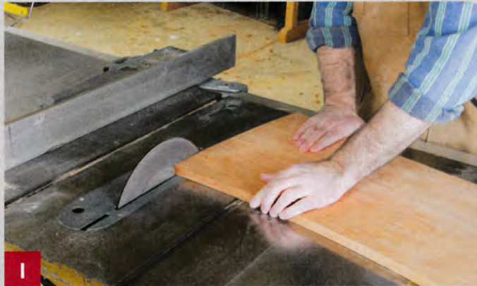
I With a tablesaw-mounted sanding disc, work only off of the forward half of the disc, which is spinning downward into the saw slot.
