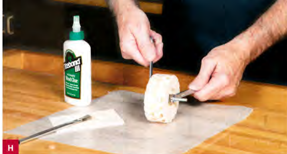
Use a pair of wrenches to tighten the nut and washers on the glued-up tire halves. Make sure the treads create an offset V-pattern.
