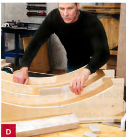
D Position the test slices on the jig to check the stave angle. Adjust your saw as needed for a seamless fit.
