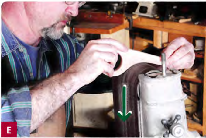
E When shaping curves on the drum of a stationary belt sander, hold the piece perpendicular to the axis of the drum, and check your progress frequently.
