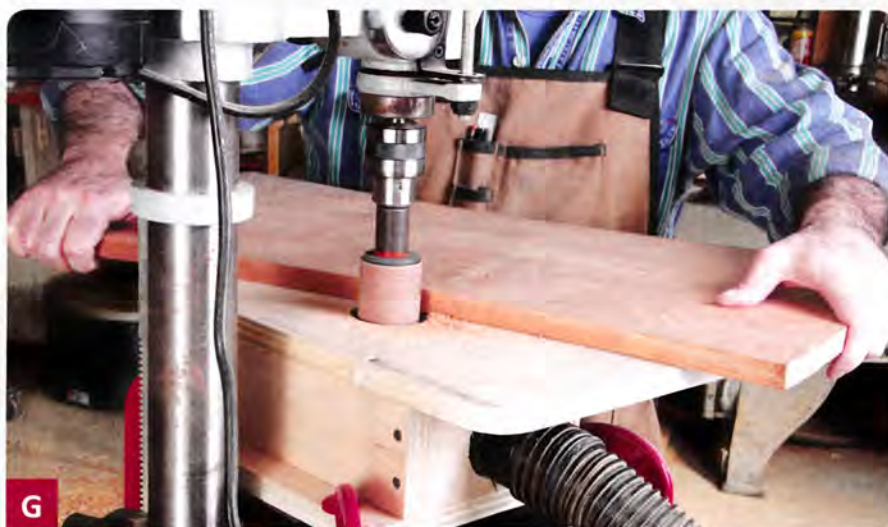
G A boxed platform that accommodates a sanding drum substitutes for a spindle sander. A port in the side allows attachment to a shop vac.
