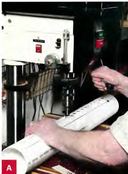
A Hold the pipe to the drill press fence as you bore each suction hole at the marked locations.
