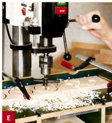
E Cut out the outside tire halves with a circle cutter at the drill press using a low RPM.
