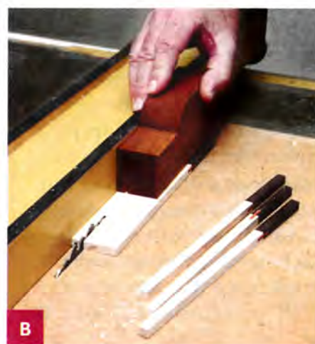
With the blade just above the top surface of the blank, rip the individual chopsticks to width.
