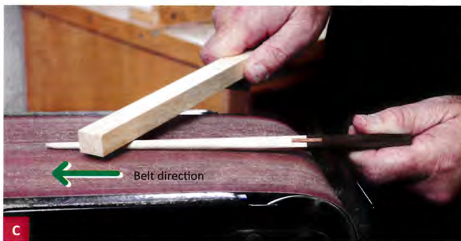
To taper-sand each chopstick to uniform shape, use a strip of wood to safely press the stick onto the sanding belt.
