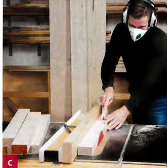
C With the blade tilted away from the fence, bevel both edges of the test stave.
