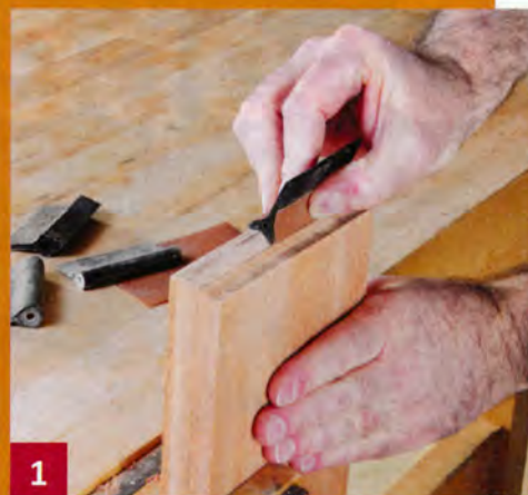
Contour sanding pads allow you to smooth a complex profile by targeting one section at a time.
