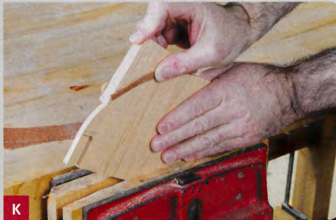
K Even if the curve on an offcut is a bit lumpy, it will serve as a sanding block to fair the curve on the piece from which it was sawn.
