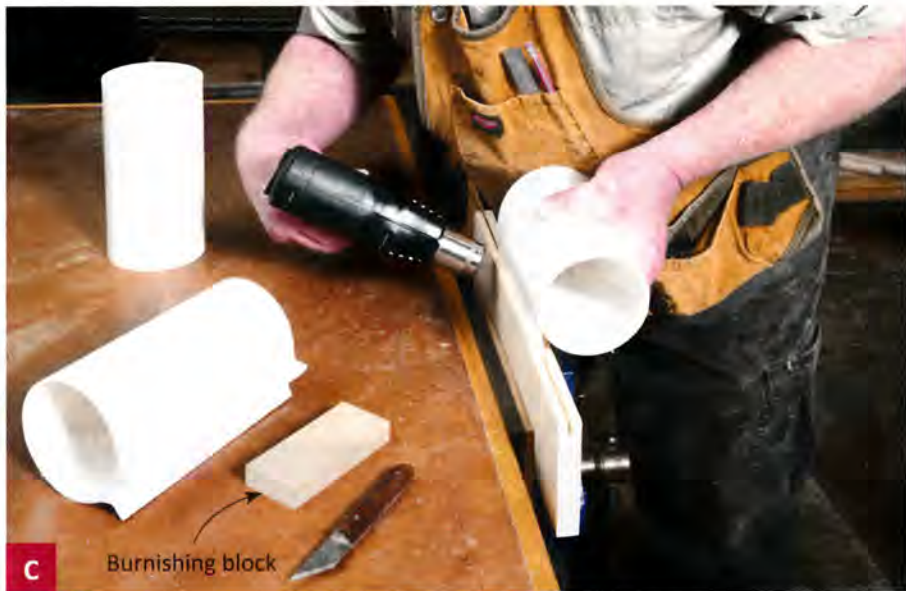
C Move the heat gun along the shutter pipe; when the plastic becomes pliable, bottom out the edge in the kerf and roll the pipe over.
