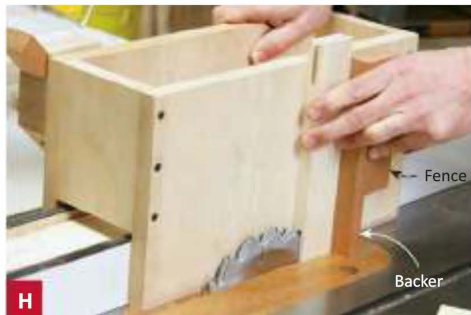
H The easily replaceable backer on this tenoning jig attaches with two screws driven through the rear of the fence.
