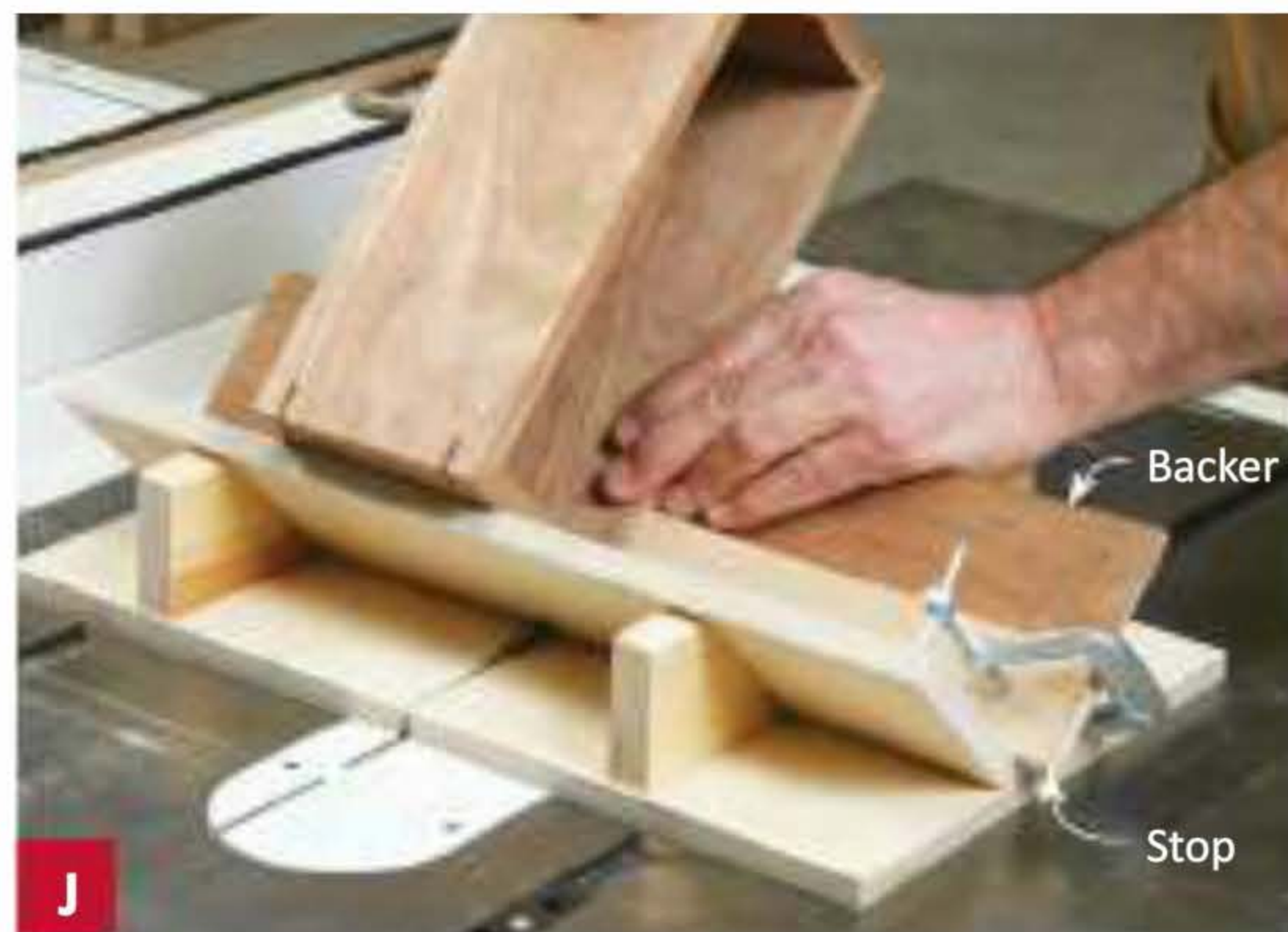
J The rear wall of this splining cradle is covered with a thin plywood backer that can be shifted to a fresh section when necessary.
