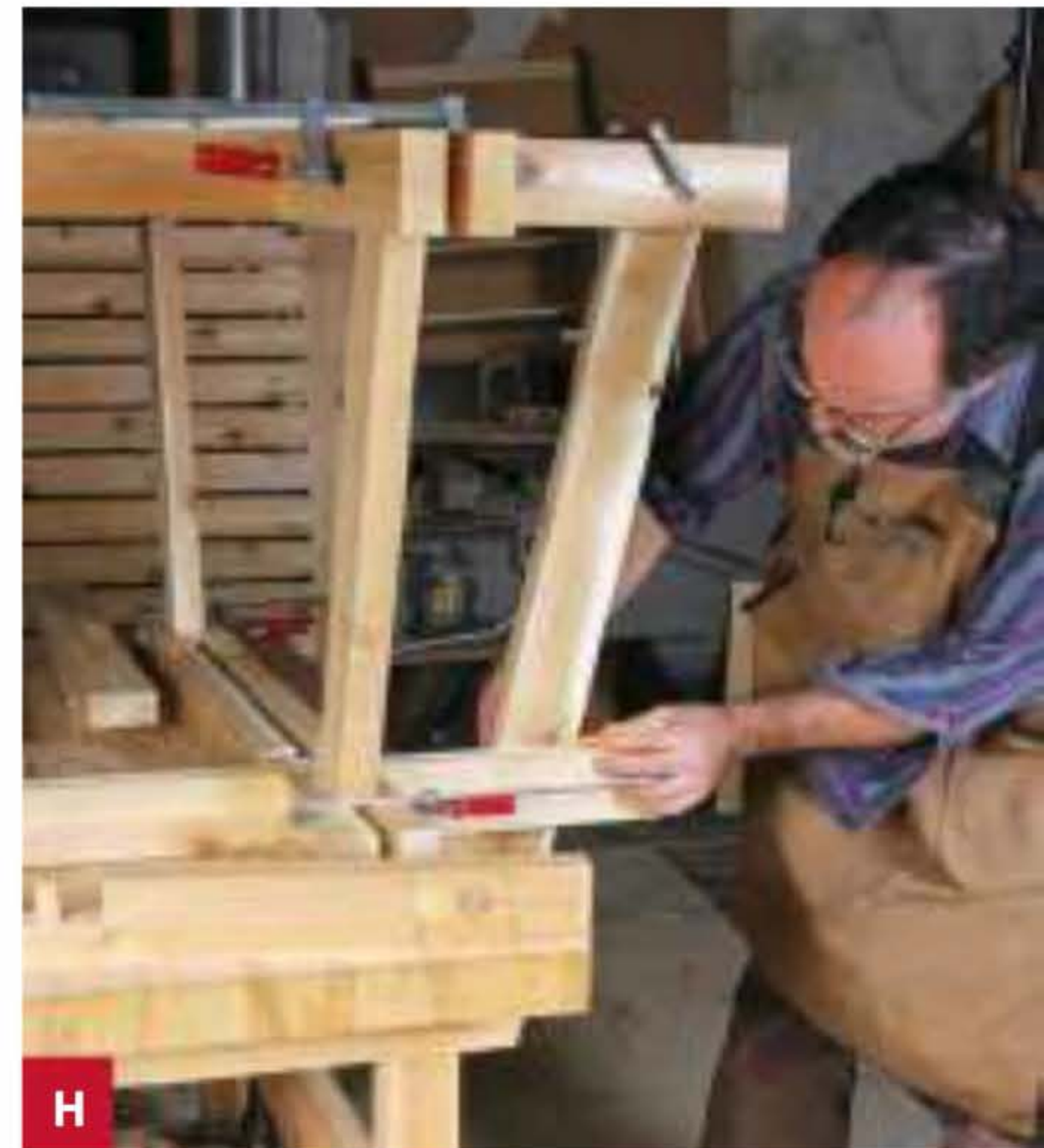
H Clamp the top of each side leg in its upper notch, and mark out where the leg intersects the cross runner.
