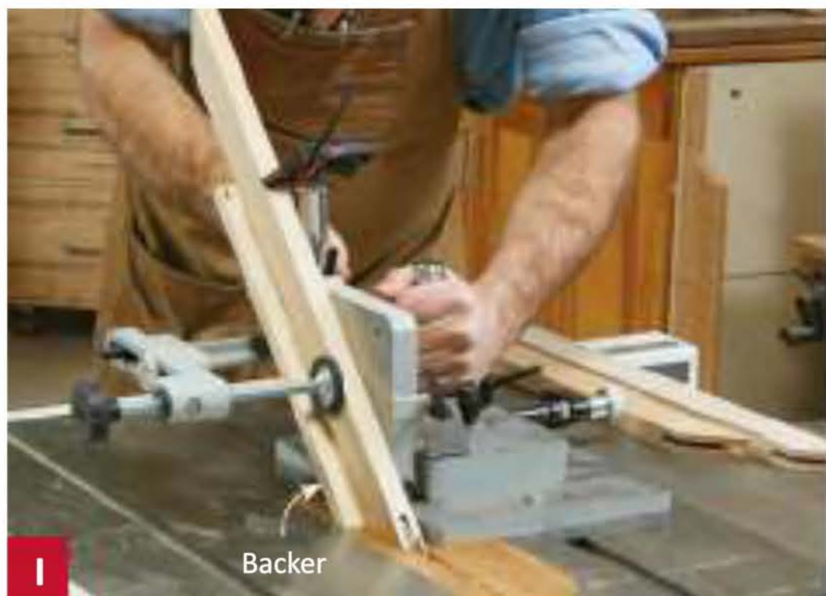
I Suit the backer to the cut and workpiece. For example, miter a backer's end to provide full support for a workpiece's mitered end.
