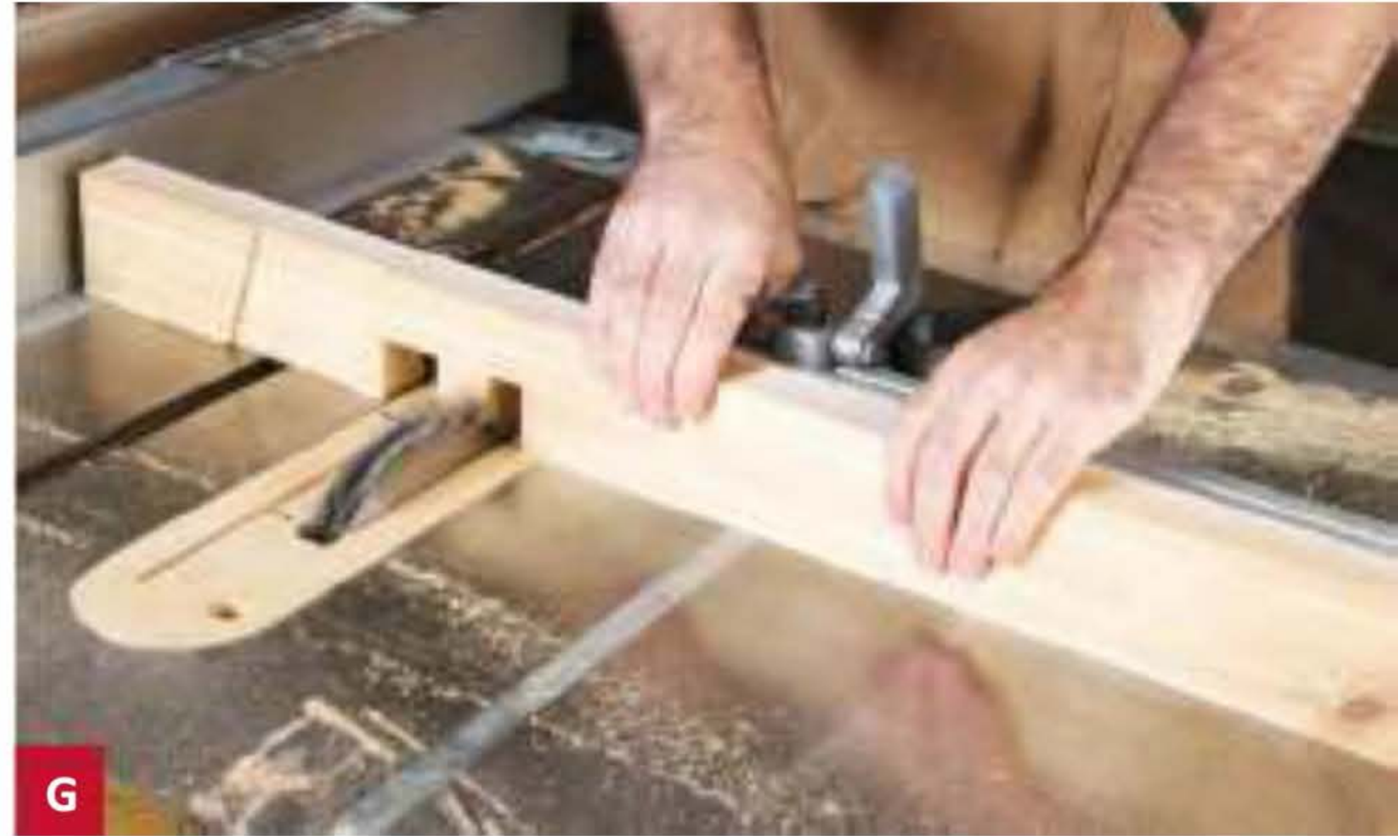
G Position the rip fence as a stop to help you keep the spacing of the notches consistent on the various pieces.
