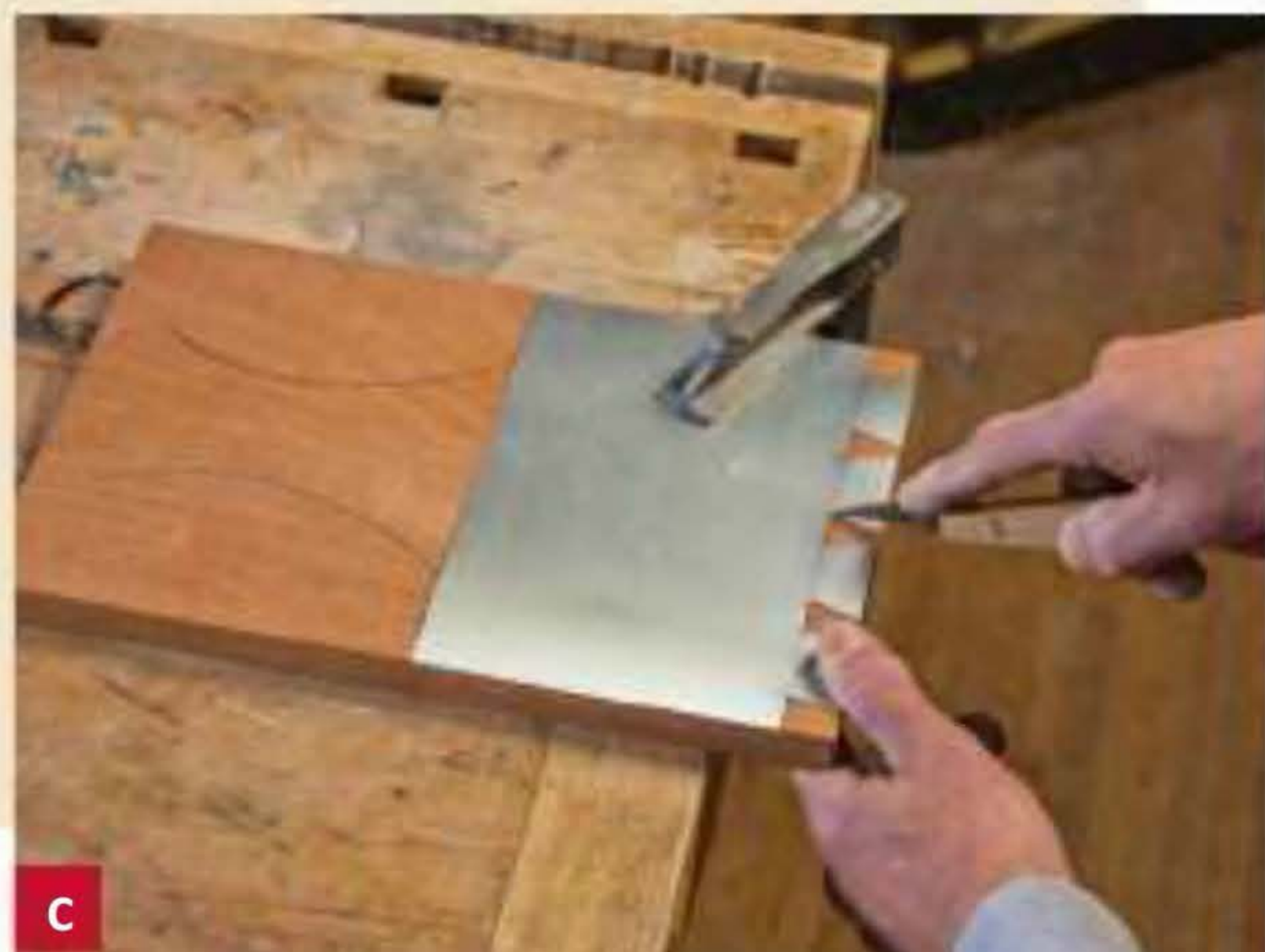
C Trace the tail pattern onto the bottom of both end boards. A marking knife produces a crisp line.
