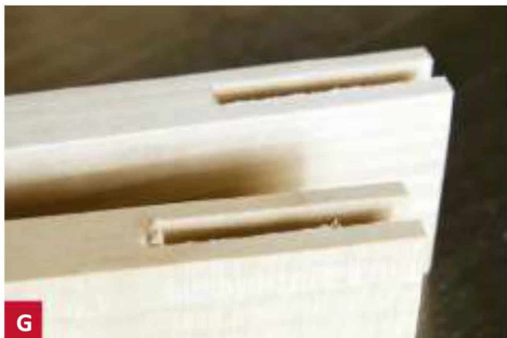
G The unbacked fibers at the end of the open mortise at the bottom tore away. The mortise at the top was backed during the cut.
