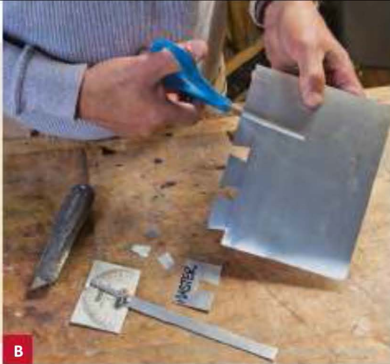
B Score the baseline with a utility knife, and then cut the tail cheeks using heavy-duty scissors. The waste should snap off with a little bending.
