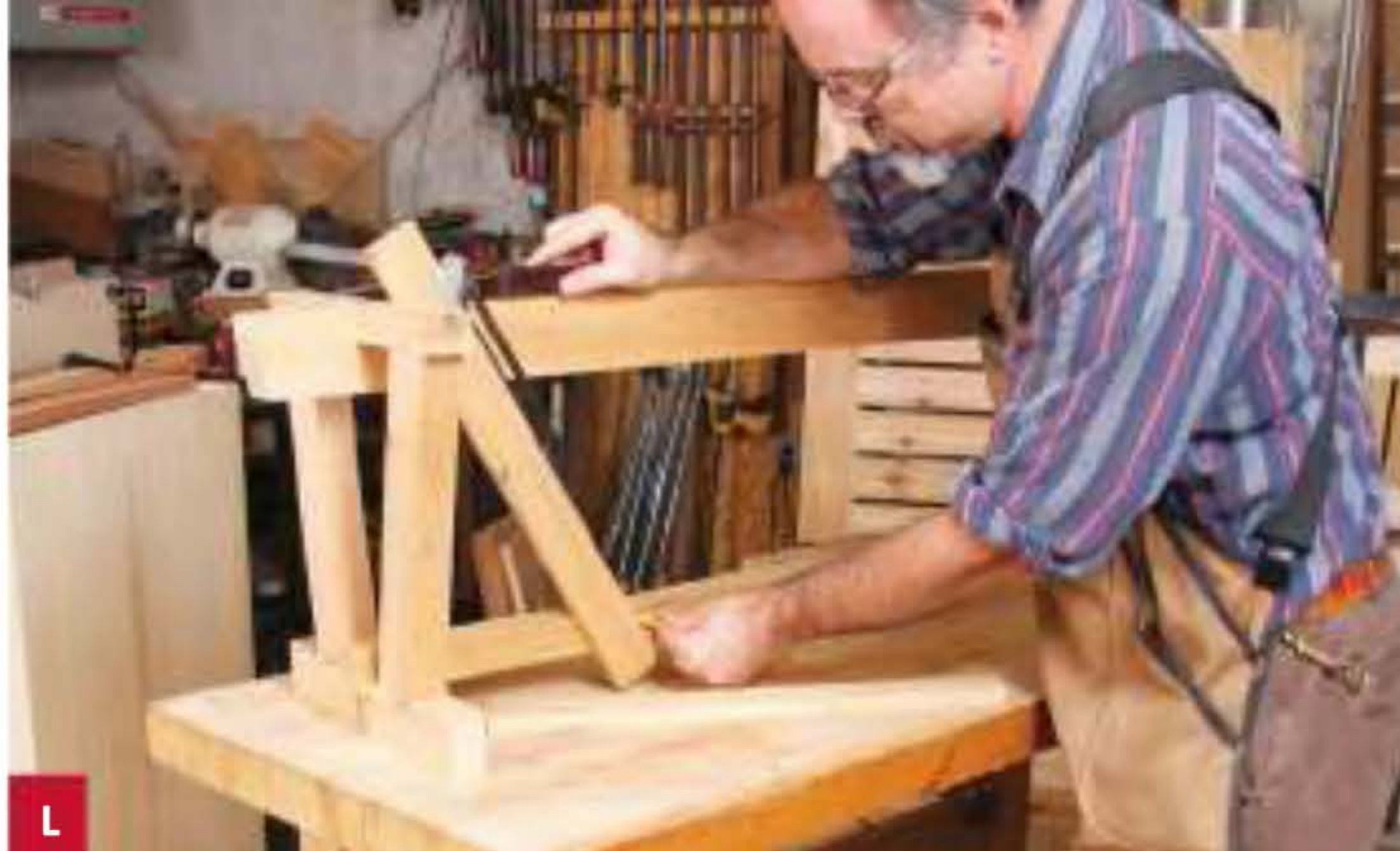
The braces add needed strength to the benches while echoing the table's angled legs.
