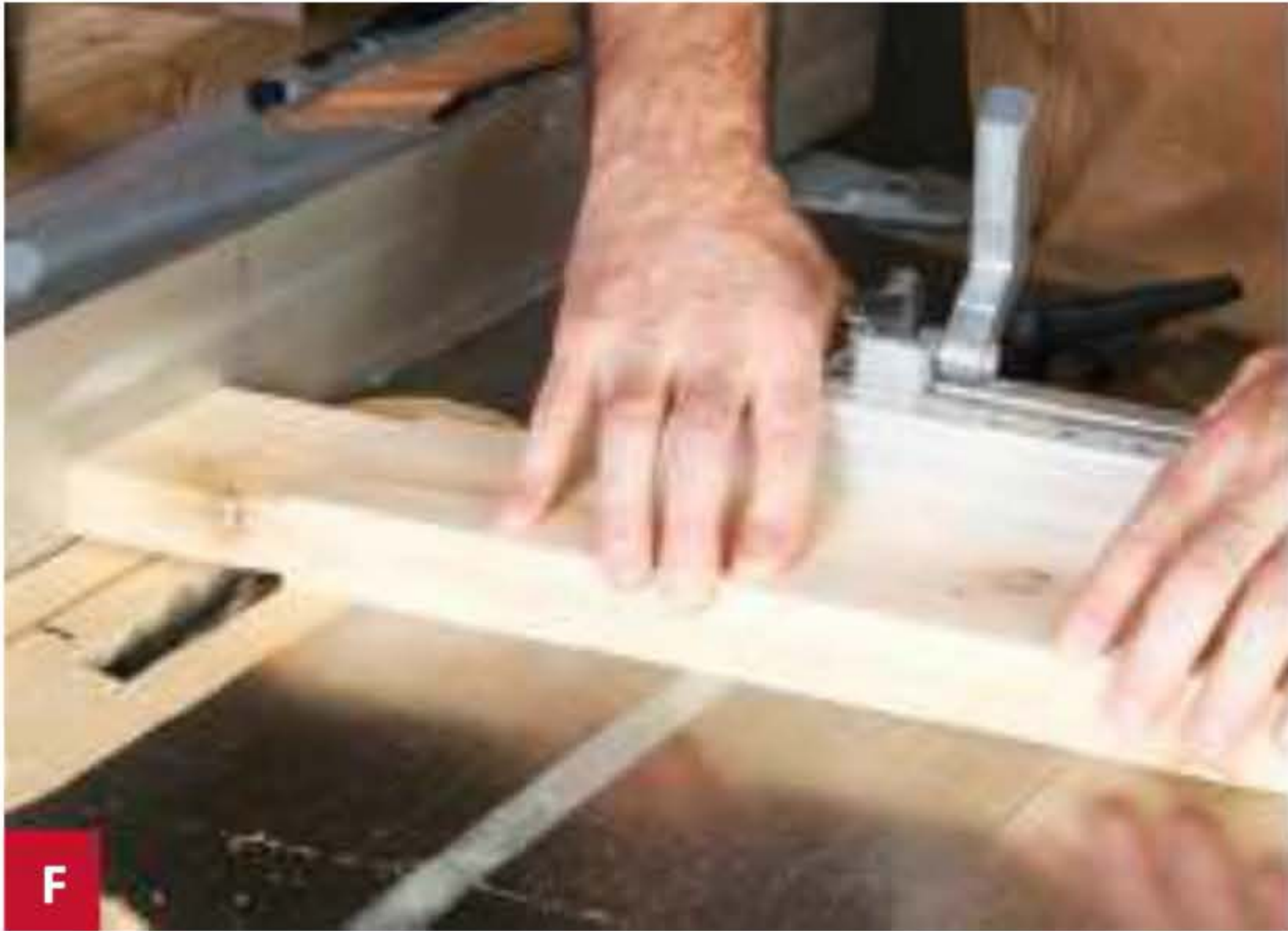
F Make overlapping passes across the dado head to create the wide rabbets at the ends of the legs. Use the rip fence as a stop to ensure consistency.
