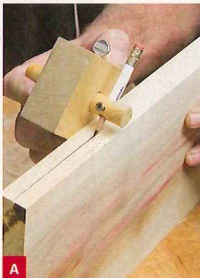
A A shop-made marking gauge outfitted with a pencil scribes a dark, clearly visible line.
