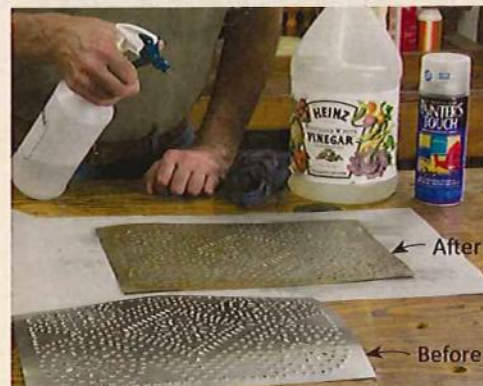
Spray on vinegar to “age” the tin and lacquer to lock in the look.
