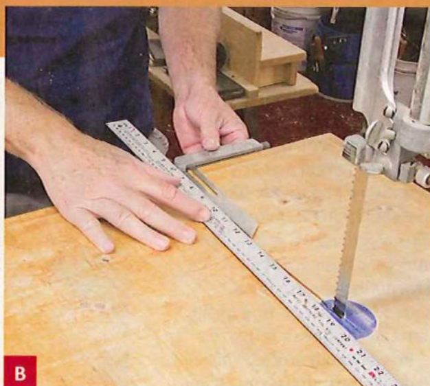
Use a bevel gauge and straightedge to position the primary fence for sawing to the desired veneer thickness with respect to the blade's drift angle.
