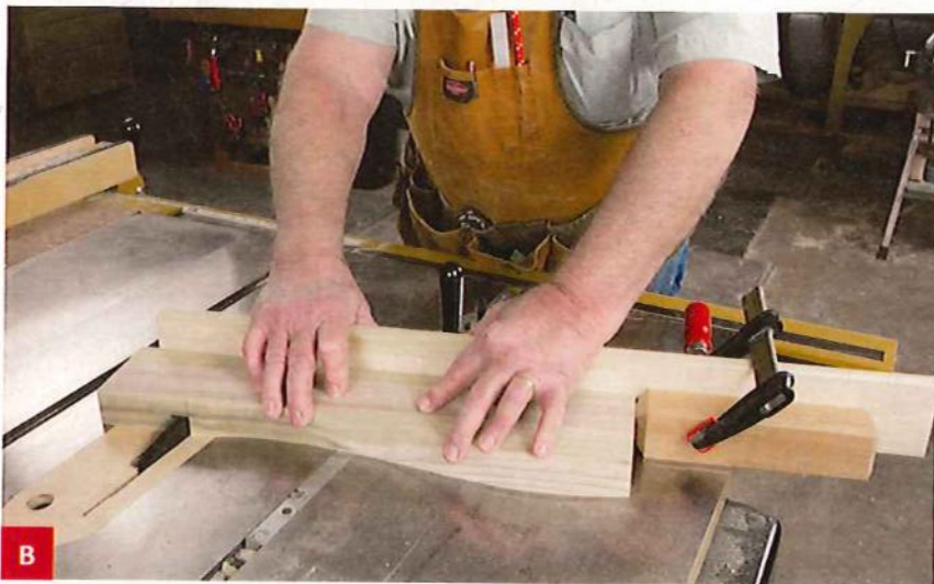
B With the miter gauge fence angled at 15°, cut the half-lap joints with a dado set, starting at the shoulder cutline. A stopblock ensures consistent results.
