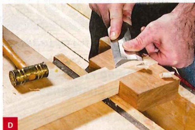
D Use a wide chisel to pare the handle tenon dead-flush with the interior surface of the mallet head.
