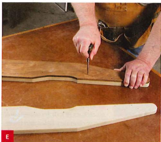
Use a scratch awl to mark the holes in the arms, guiding off the \frac{1}{8} " holes drilled in the plywood template.
