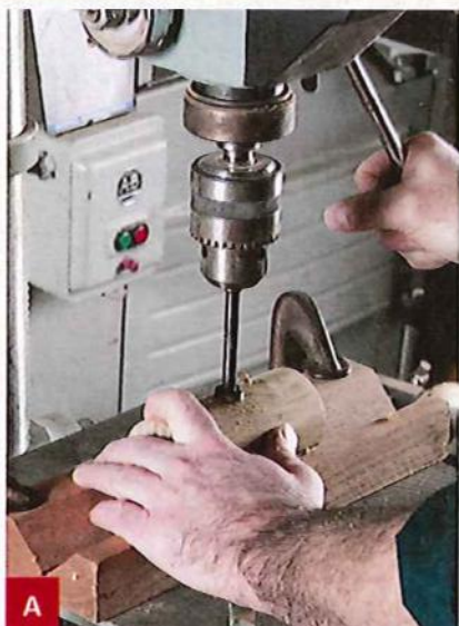
A Drill the handle hole by cradling the mallet head in a V-block that was sawn on the tablesaw.
