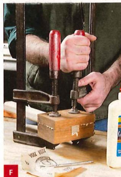
F Two stout clamps should be enough to glue on the third mallet head piece.
