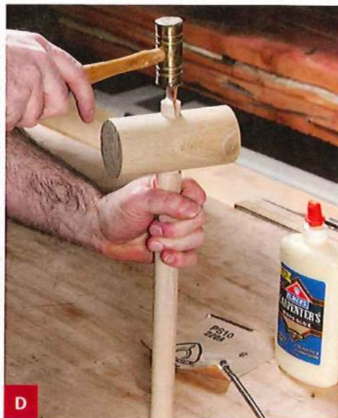
Install the wedge perpendicular to the axis of the head; then trim and sand away the tenon waste.
