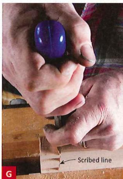
For a shoulder cut, align a chisel with the scribed line at the base of the tails (here) or tenon shoulder.
