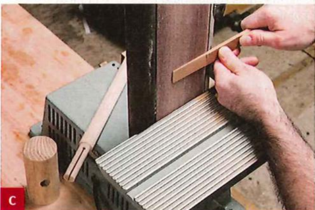
C Start making the wedge with a strip of \frac{3}{16} "-thick scrap that is long enough to provide a good grip. Sand it to shape, making the thin end about \frac{1}{32} " thick.
