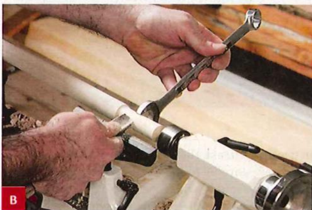
B While turning the handle tenon, you can use a \frac{3}{4} " open-end wrench to gauge the final diameter.
