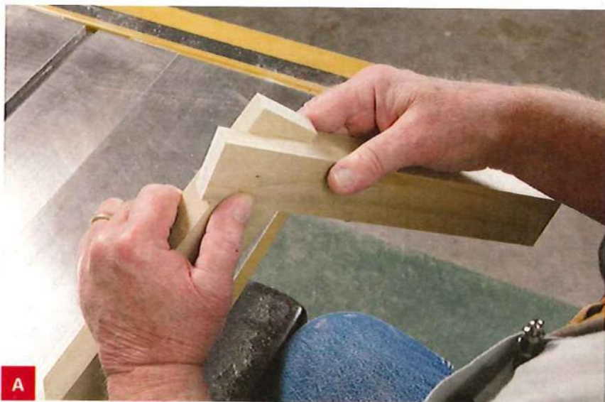
A Test-cut scrap pieces and hold them together to confirm the rabbet depths and angle settings.
