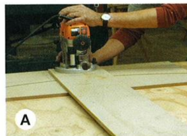
Mounting a router to your trammel is an easy way to cleanly cut the curves for the top rail template.
