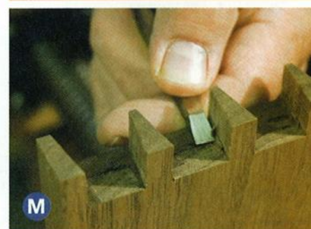
Pare the pin socket with a narrow chisel to maintain good control when cutting. Use a square to make sure the socket is flat.
