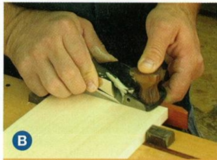
Plane a shallow rabbet along the inside face of the tail board to establish an easily referenced lip for laying out the pin board.
