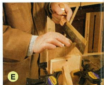
The plywood square works as a convenient drawer clamping jig and raises the stock above the bench so that it's easier to see the saw cuts.
