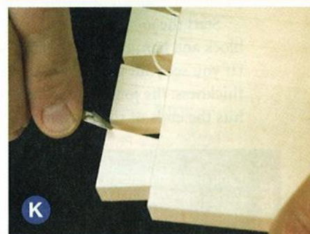
Chamfer the inside edge of the tails to help align the joint during assembly and facilitate gluing.
