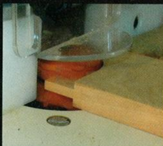
Step 1. Cut the tenon in the rails.
