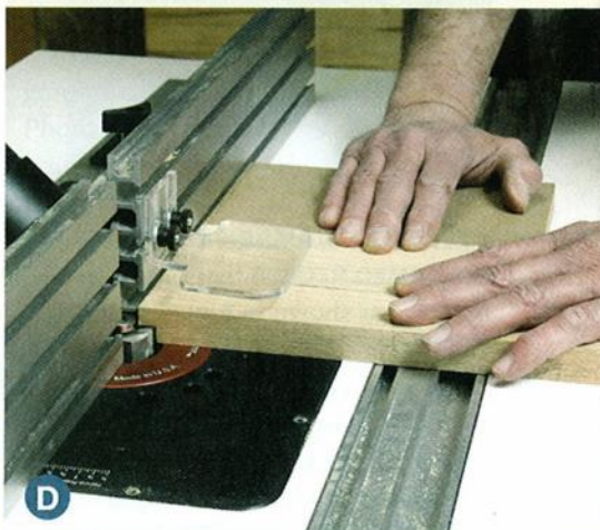
When making end rabbets, a squared cutoff can provide backup and prevent tear-out at the end of the cut.
