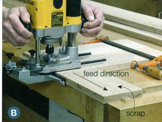
Clamp boards side-by-side to create a longer bearing surface for the edge guide. Scrap placed where the bit exits the wood prevents tear-out.
