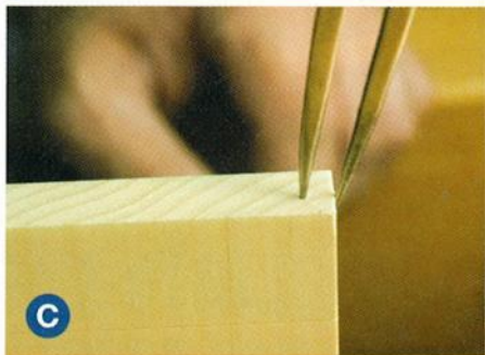
Make a small indent 1/4" in from each edge to mark the location of the half pins.
