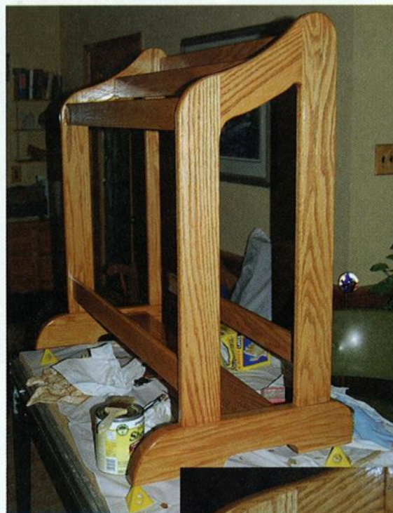
EMLYN JONES USED mortise-and-tenon joinery (see closeup right) for his version of Woodcraft Magazine's Heirloom Quilt Stand.
