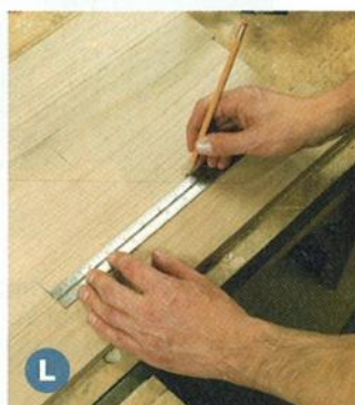
L Position the biscuits every 8" across the joint.
