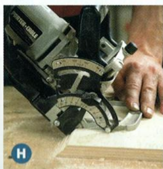
Adjust the fence height or add a shim so that the blade does not cut through the tip of the miter.
