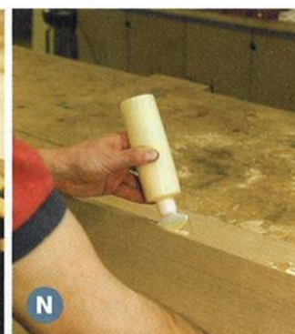
N Use a biscuit-slot bottle to quickly squeeze glue into the slots.
