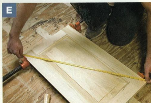
CHECK YOUR DOORS FOR SQUARE before you fully snug up the clamps. Check for flatness using a straightedge after you tighten them.
