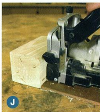
Place a spacer under the joiner to raise the slot and set the height of the offset.
