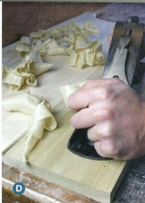
Hand-planing levels edge joints and smooths the side assemblies in a single step. Before planing, scrape away dried glue so it won't chip your blade.
