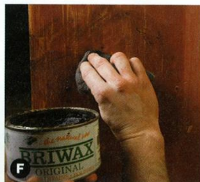
F Apply a dark wax topcoat. Buff off the flat surfaces but leave some wax behind in cracks and crevices.
