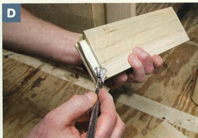
APPLY YOUR GLUE neatly and evenly. Aim for minimal squeeze-out to clean up. You'll also minimize your risks of gluing the panel into the grooves.
