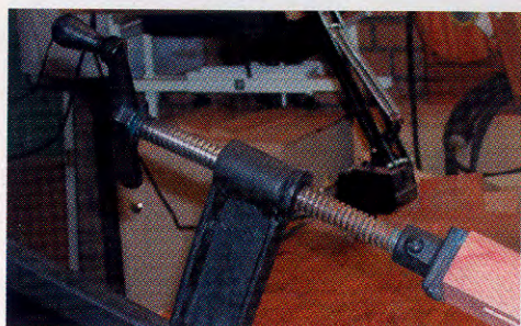
THE ADJUSTABLE HEADSTOCK and tailstock increase the flexibility for positioning a workpiece.
