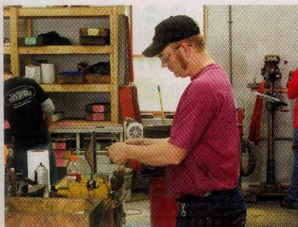
Chris Gamage is one of three LN employees who produce scrub planes. Here, he's filing the mouth on a copy of the LN version of the Stanley 40 1/2.
