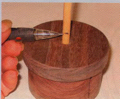
7. Mark the dowel \frac{3}{4} " above the lid before trimming to size.
