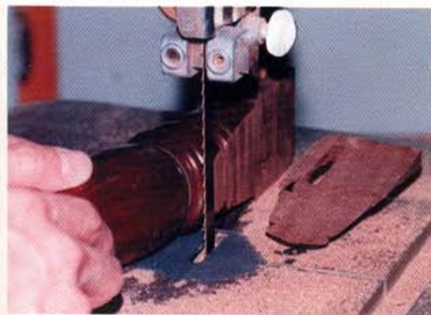
TO MAKE A SCARF REPAIR first cut away the damage at a long angle to the grain using a bandsaw.
