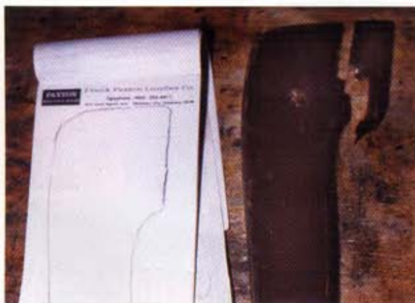
WHEN PATCHING AN EXISTING part, it's very helpful to draw an outline of the part using the original pieces. You can then use this outline to cut the exact shape.
