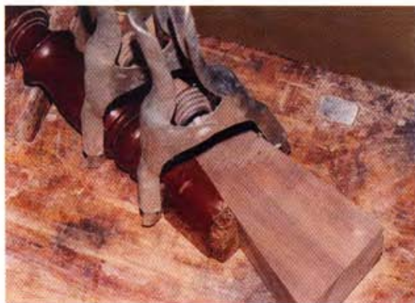
GLUE THE REPLACEMENT patch to the original. Framemaker's spring-miter clamps have built-in teeth for a firm grip and are handy for reducing sliding during glue up.
