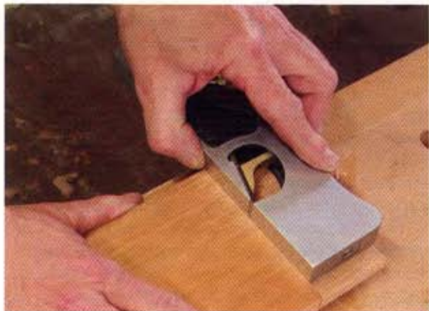
THE MEDIUM SHOULDER PLANE makes clean paring cuts across the end grain surfaces of the shoulders surrounding a tenon.
