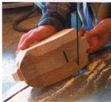
4. When rounding the top and belly, cut to within about \frac{3}{4} " of the glue line.
