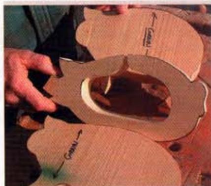
1. Cutting the opening in your center hole in a funnel shape makes coins fall out easily when the finished bank is turned upside down.
