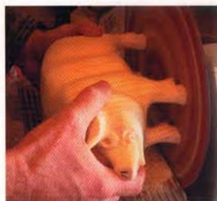
11. Finishing touch: level up the pig's feet with a disc sander.
