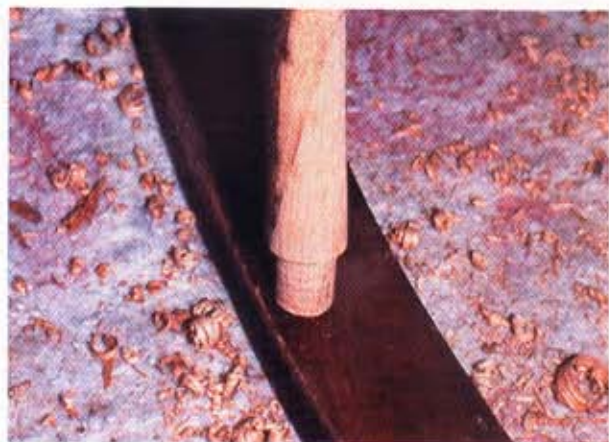
BROKEN TENONS ARE usually best repaired by scarfing on new wood. In this case it was possible to do so without disassembling the rocking chair.
