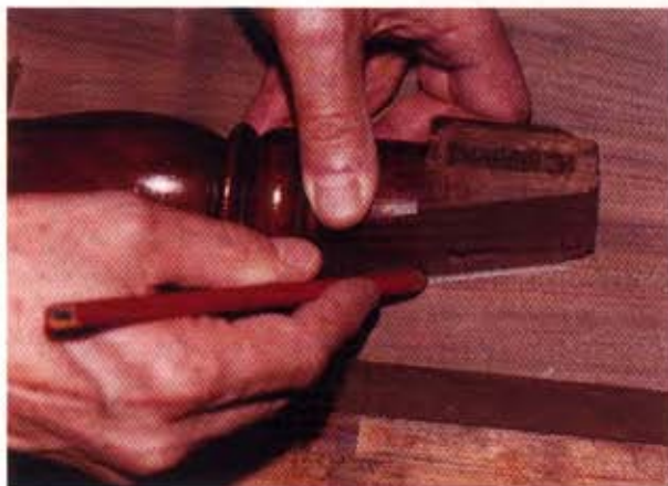
WITH THE LONG ANGLED cut planed perfectly flat, lay out the angle on the replacement wood by holding the original up against it and drawing a line.
