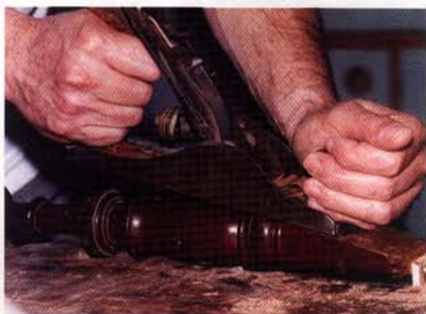
HAND-PLANE THE ROUGH scarf cut perfectly flat. If the part is still attached to the furniture, it can sometimes be a challenge figuring out how to hold the furniture steady.
