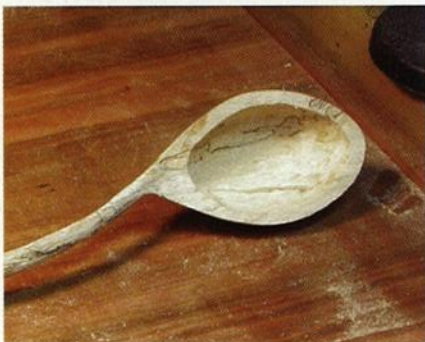
10. Switch to a fine-grit burr and lightly sand the entire piece, taking care not to alter the shape.
