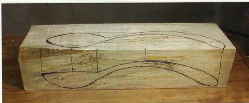
1. Draw the top view on your blank, transfer several points to an adjacent side, and draw the side view.
