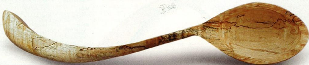
10. Switch to a fine-grit burr and lightly sand the entire piece, taking care not to alter the shape.
