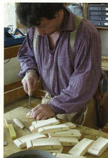
A SWISS ALPINE COOPERAGE STUDENT works on staves that he will join together to form a cylindrical cask.
