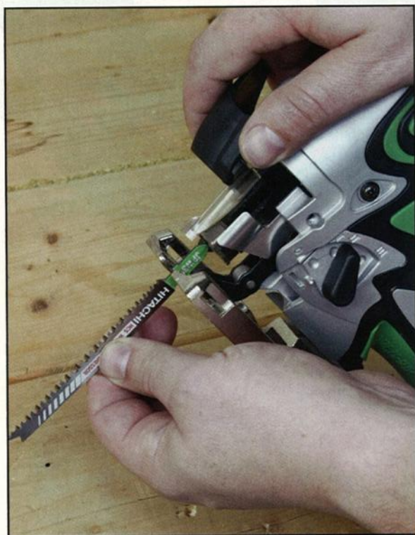
BLADE CHANGES ARE EASY with this jigsaw's built-in, spring-loaded locking lever
