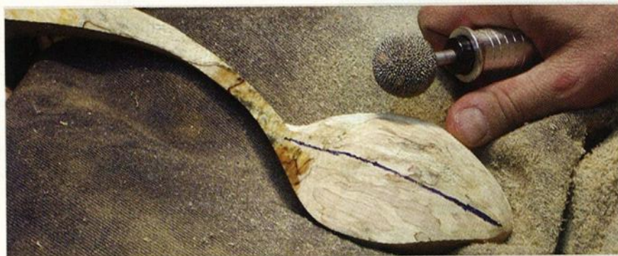
6. Shape the bottom of the spoon's bowl with a coarse round burr.
