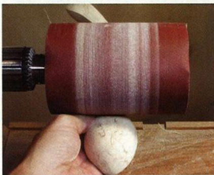
11. Or, remove all traces of the rough burr's cutting action with an inflatable sanding drum mounted in your lathe. Keep the air pressure low.
