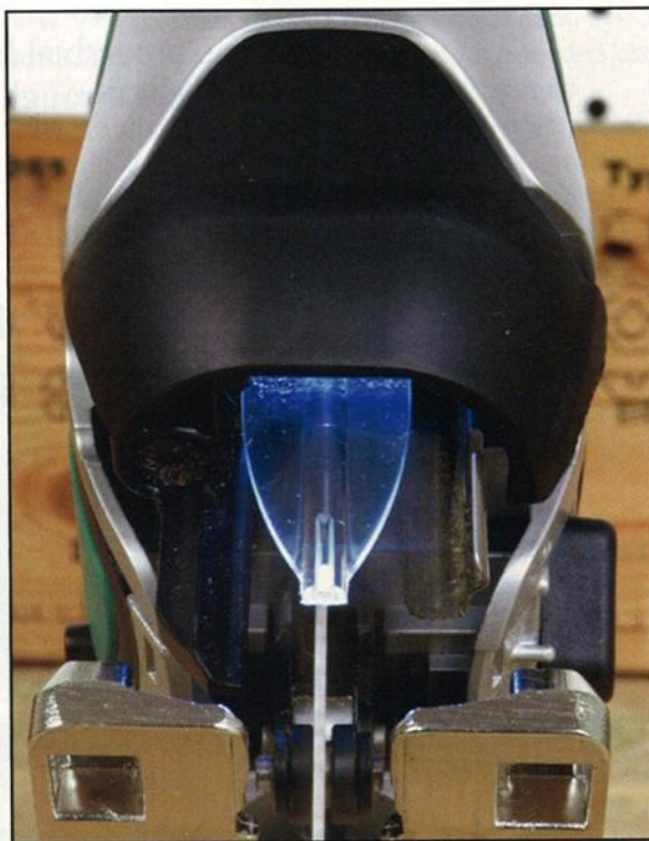
BUILT-IN BLOWER AND BRIGHT LED light the way and keep your cut line clear.
