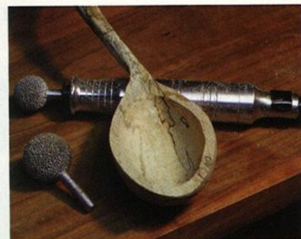
9. Switch to a smaller burr if yours becomes difficult to control. Take light, continuous final passes on the bowl's interior.
