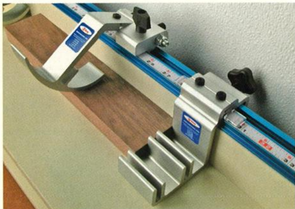
THE KREG SYSTEM ACCOMMODATES the basic Flipstop, left, or the dual-cursor Production Stop, right.
