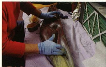
The liming wax, tinted with yellow pigments, is rubbed deep into the grain.
