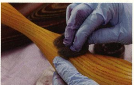
A thorough rubbing with fine steel wool leaves coloration only in the grain.
