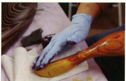
The top form receives a coat of shoe polish on top of yellow stain.
