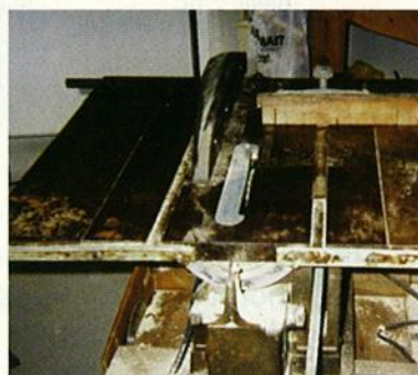
THE CRAFTSMAN MODEL 80 was really a Walker-Turner table saw sold under the Sears brand.
