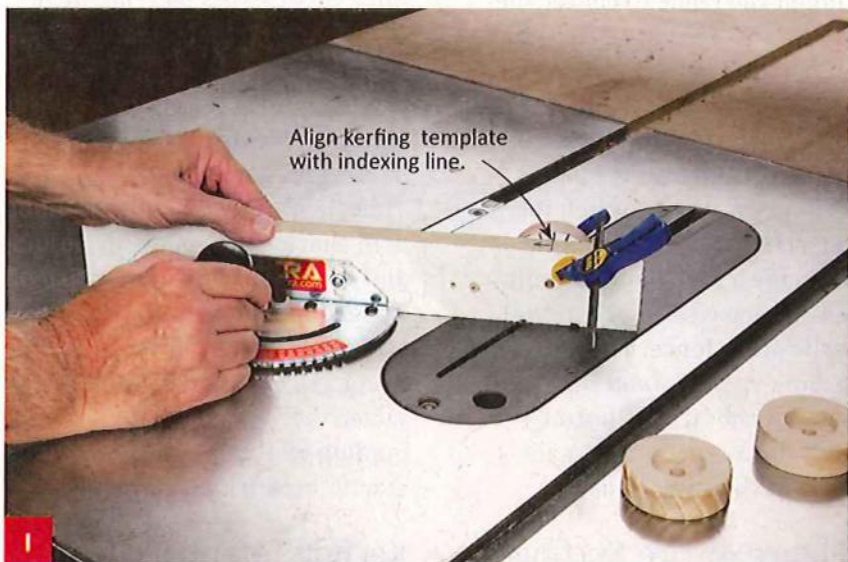
Align the template's start line with the jig line, and then cut, rotate the tire, and cut again, making evenly spaced kerfs. Stop at the stop line.
