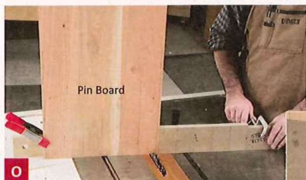
O Set up the first pin cuts by aligning the left-hand half-pin with the left side of the blade. Then locate the spacers and stopblock to the left.
