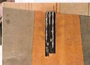
O Set up the first pin cuts by aligning the left-hand half-pin with the left side of the blade. Then locate the spacers and stopblock to the left.
