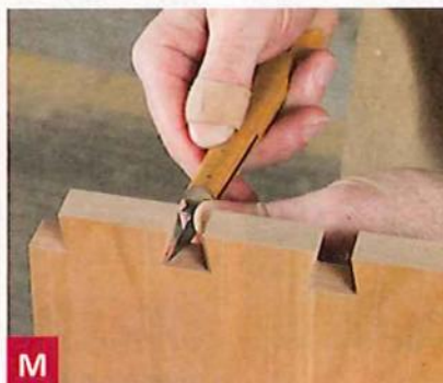
M Once you have trimmed the shoulders, clean out the corners with a knife.
