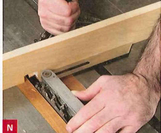
N Use your pre-set T-bevel to adjust your miter gauge before cutting the pin board.
