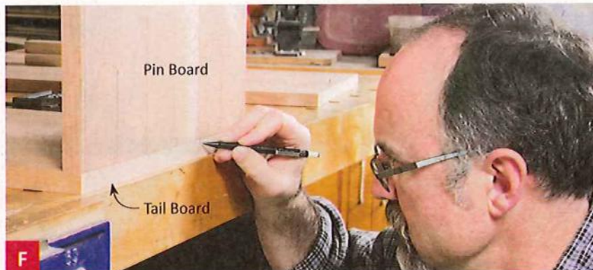
F Stand the pin board on the tail board, and transfer the marks indicating the pin cheeks onto the end of the tail board.
