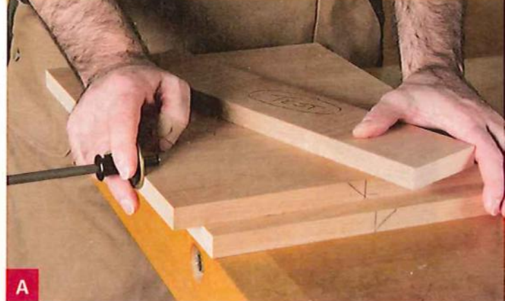
Scribing shoulders with a marking gauge helps prevent tear out and serves to register a chisel when paring.
