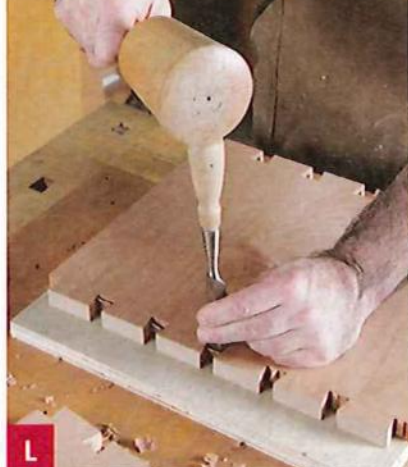
L Pare or chop to the scribe line to clean up the saw cuts.
