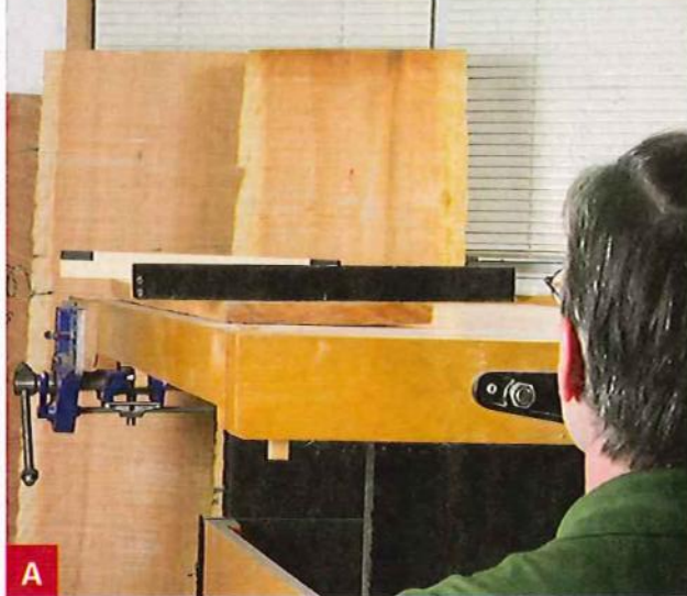
A Using a pair of metal or wooden winding sticks, sight across the top of the sticks to reveal any twist.
