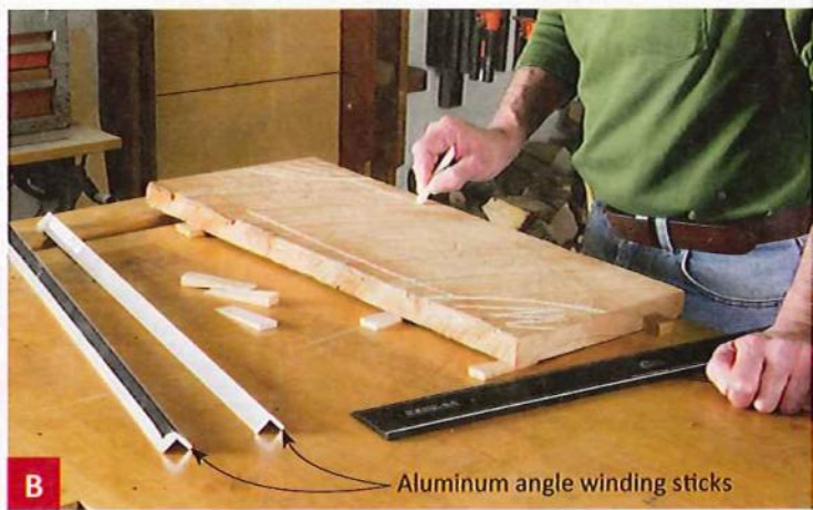
B Mark the high spots with chalk. Insert wedges to keep the board from rocking or deflecting when planing.
