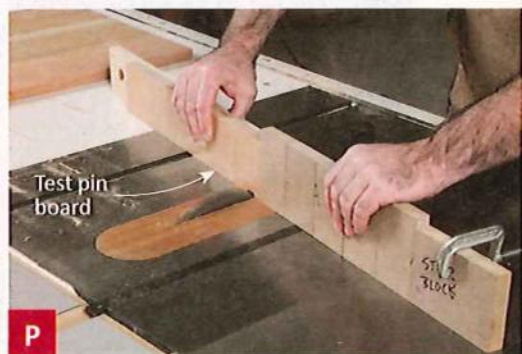
P Cut the left-hand half pin with all the spacers in place against the stopblock.
