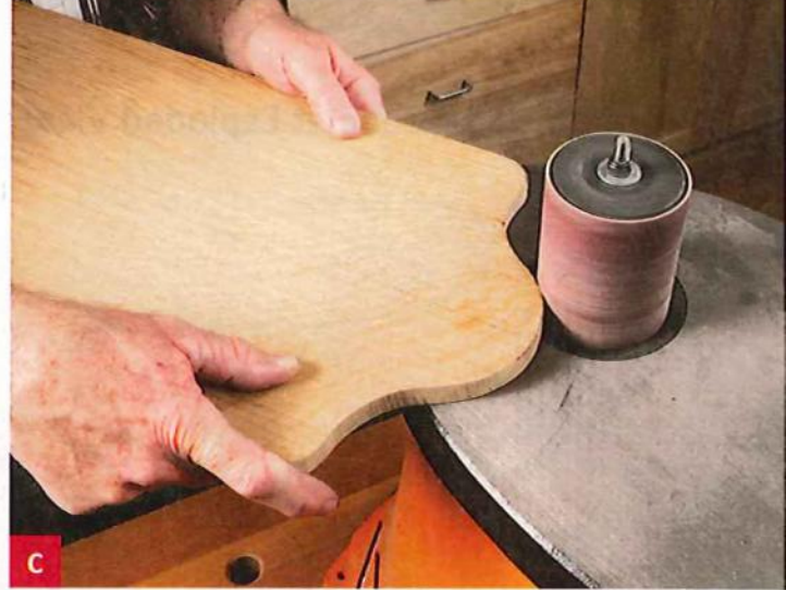
C Use an oscillating spindle sander to sand off waste, moving the workpiece against the counterclockwise motion of an appropriately sized drum.
