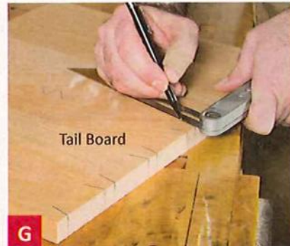
G Use the pre-set T-bevel to extend the tail lines onto both faces of your tail board.
