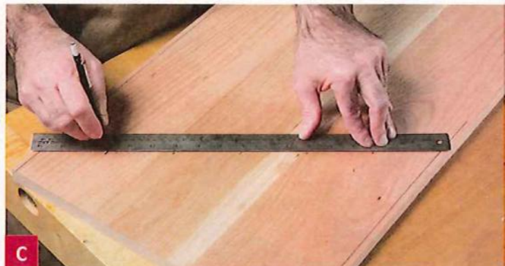
Angle the rule to find an easily divisible number. Then mark and extend the center lines for the full pins.
