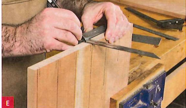
E When laying out pins, orient the T-bevel so that the pin's narrow face is on the outer face of your board.
