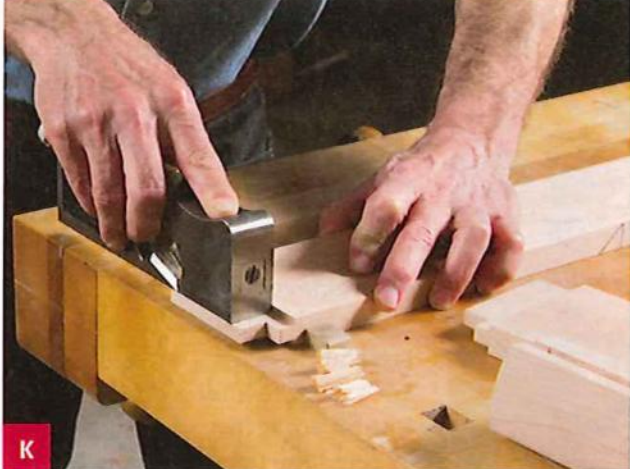
K Use a shoulder plane set for a very fine cut to trim each tenon for a snug fit in its specific mortise.
