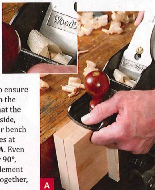
A Planing both edges at once ensures complementary edges. Use the shavings to check your progress.
