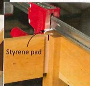
M Glue the legs to the short aprons after attaching soft pads to your clamp faces. Partially insert the long-rail tenons to keep the legs from cocking.
