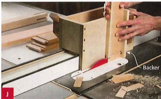
J Use a tenoning jig to cut the tenon cheeks. A backer on the jig prevents exit tear-out.
