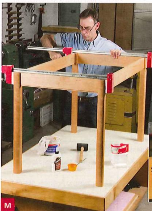
M Glue the legs to the short aprons after attaching soft pads to your clamp faces. Partially insert the long-rail tenons to keep the legs from cocking.
