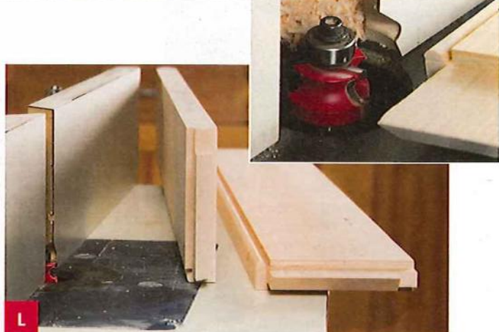
L Use the router table to cut a bead on the outside bottom edges of the aprons.
