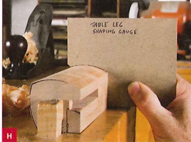
H Register the shaping gauge against a mortised leg face to check your planing progress on the curved face.
