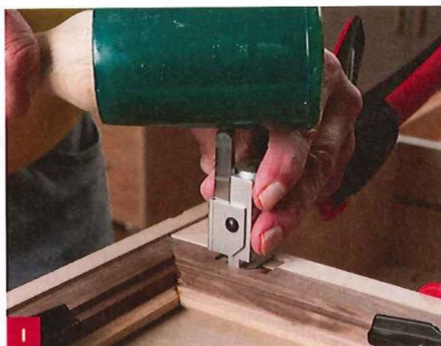
I Fit the corner chisel into a mortised corner, and then smack its spring-loaded cutter pin for a crisp, square result.
