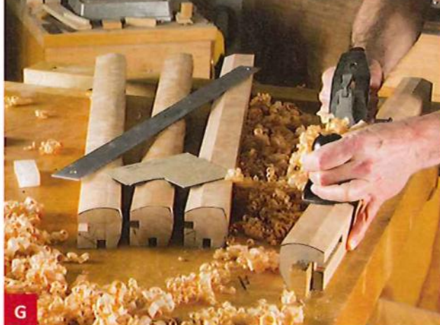
G Extending a finger against one edge of the leg helps maintain the angle of the plane throughout its stroke.
