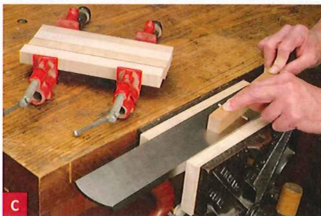
C Clamping the plane in a bench vise creates a muscle-powered jointer of sorts. Skew the stock for a smoother cut.
