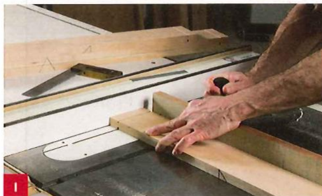
I Saw the wide tenon shoulders, feeding the apron with a miter gauge and using the fence as a stop.
