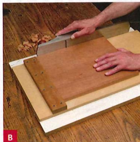
B Running a plane against a shooting board eliminates any tendency for the plane to tip.
