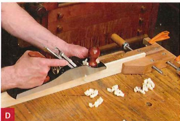
D Positioning an auxiliary stop behind your handscrew clamp can prevent a plane-to-clamp collision when working with narrow stock.
