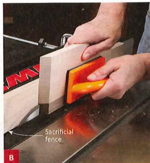
B Raise the blade to the walnut/sycamore seam, slide a sacrificial fence against it, and safely cut the rabbet.
