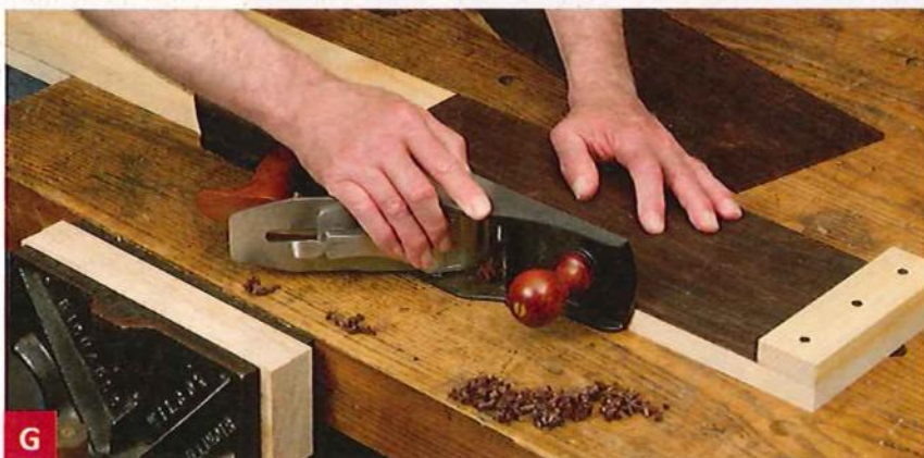
Flip the fixture over to joint edges of thin stock. The plane's side uses the bench as a reference surface to ensure a square cut.
