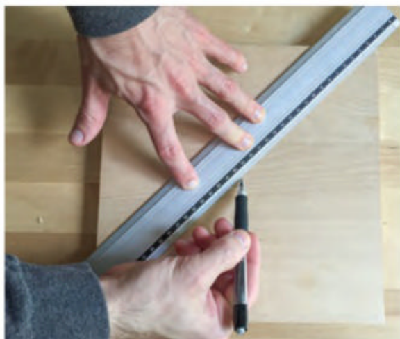
Use a straightedge to locate the center of your stock.
