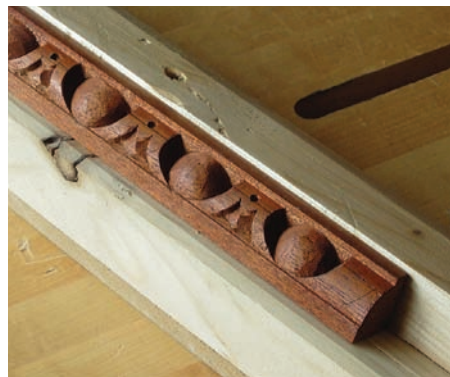
Moulding held in a jig and secured with double-sided tape.
