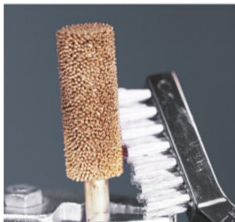
Burn the clogged bit head with a propane torch. Then brush the residual ash out with a stiff wire or bristle brush.
