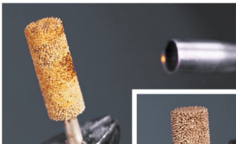
Burn the clogged bit head with a propane torch. Then brush the residual ash out with a stiff wire or bristle brush.
