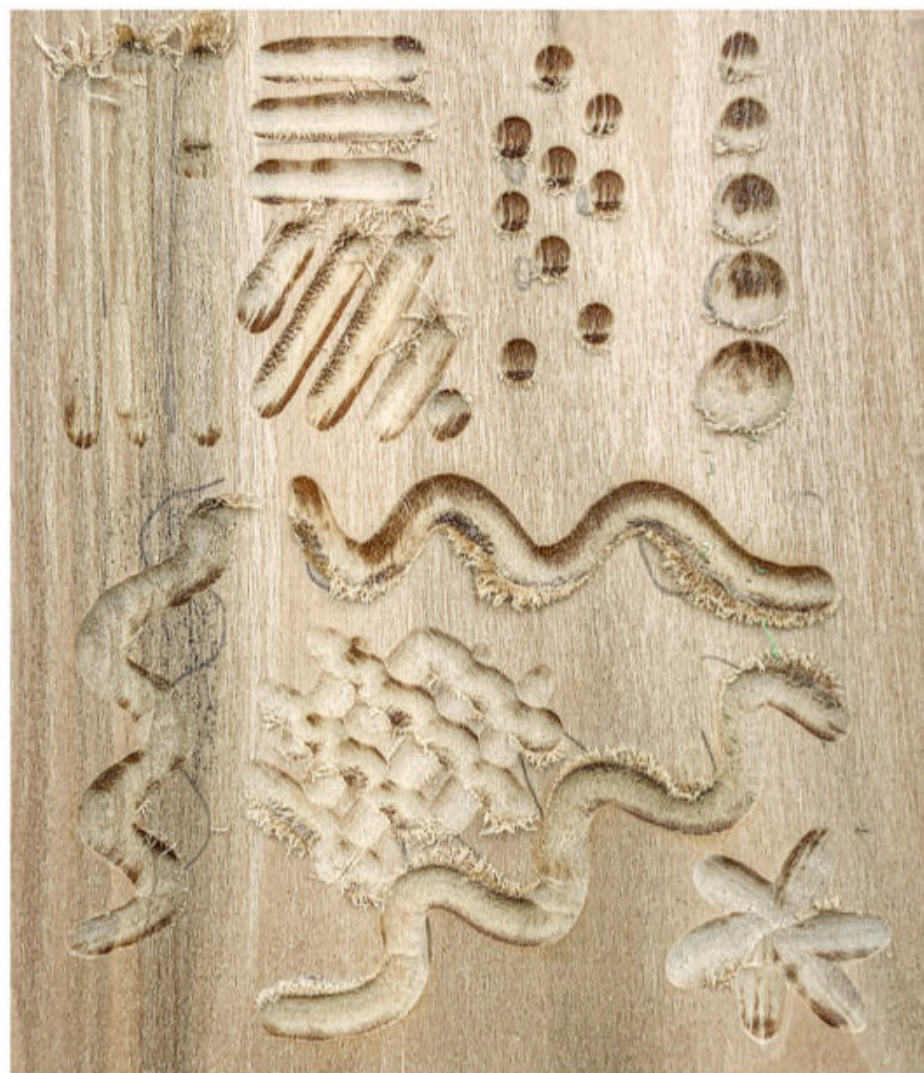
Carving with and across the woodgrain (grain runs top to bottom in photo) will help you understand how grain affects your cut. Note the "fur" raised by the carving on this piece of poplar. Different woods create more or less fur. The fur is easily removed with a few swipes with fine-grit sandpaper.
