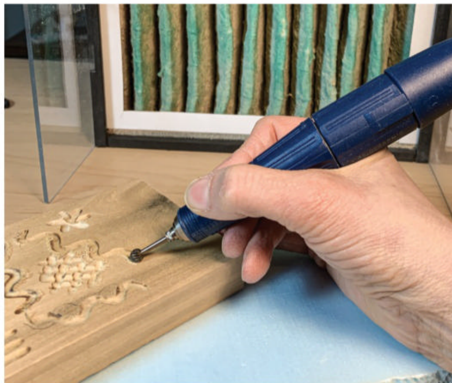
Most burrs cut best when held at an angle similar to that shown here.
