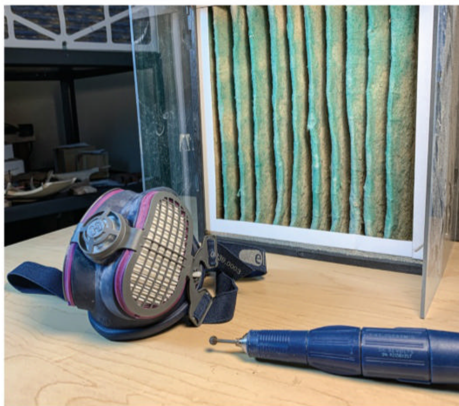
Lung protection: half-face respirator, 10" (25.4cm)-square desktop dust collector and ambient dust collector in background to filter and recirculate workspace air.
