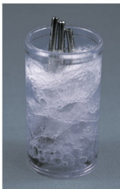
Soak bits in a hot water and cleaner/degreaser solution.
