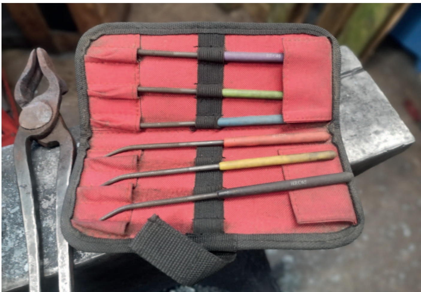
Hardness testing file set – I only use the 65, 55 but mostly the yellow 60
