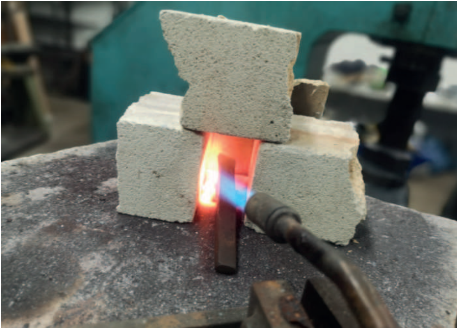
Simple heat treat set-up
