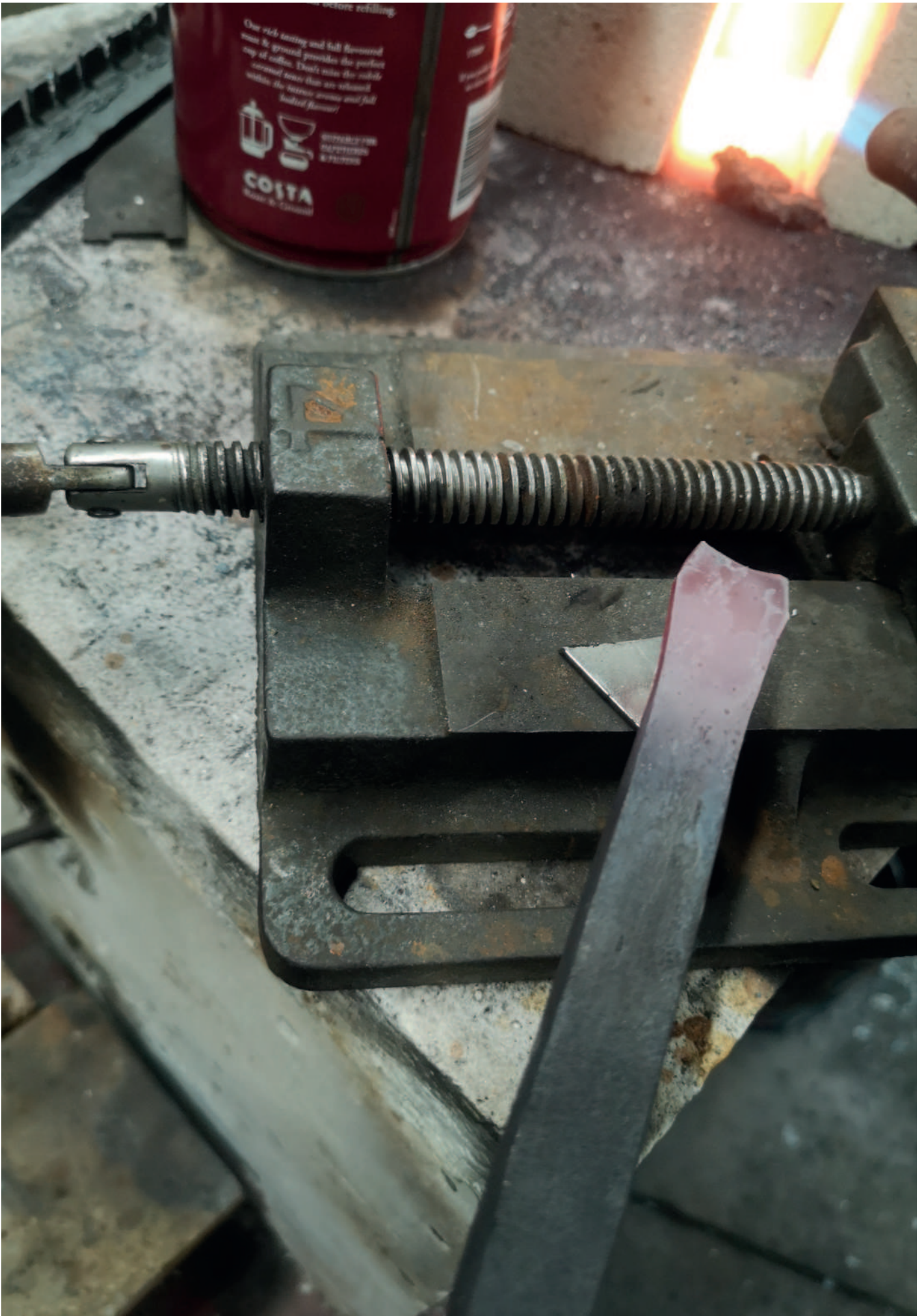
Using an old magnet to test the temperature
