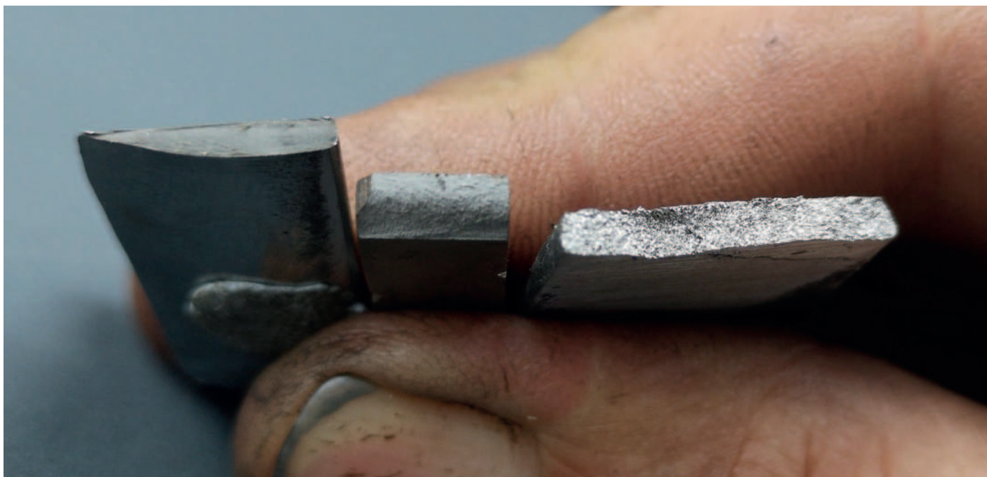
Grain size in different steels, finer is better
