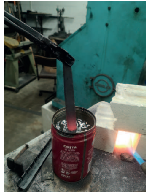
Quenching in water, not full depth
