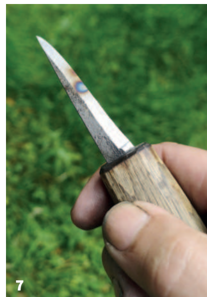
4 The notch 5 Top view of the off-centre V 6 Jointed edge showing the difference in thickness of the wings 7 Blueed, overheated and ruined edge 8 A jig that sets the edge angle regardless of the previous bevel form
