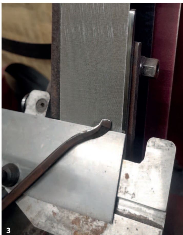
1 Spoon bent gouge as I received it 2 Cleaning up the inside with a custom-made tool, both bevel angle and diameter matched the gouge 3 Grinding the outside bevels, very poorly. Notice the limited contact between the tool and table
