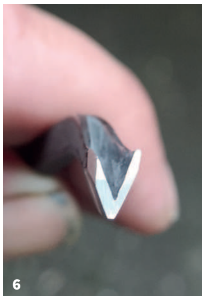
4 The notch 5 Top view of the off-centre V 6 Jointed edge showing the difference in thickness of the wings 7 Blueed, overheated and ruined edge 8 A jig that sets the edge angle regardless of the previous bevel form
