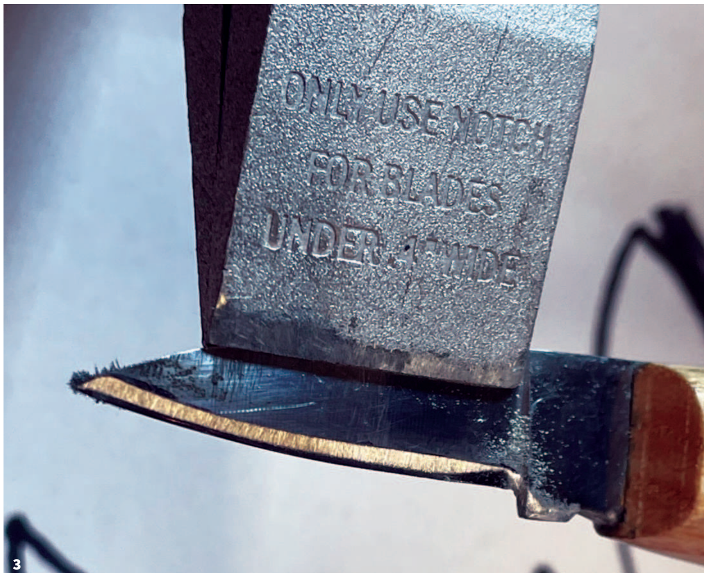
1 Stubai in need of attention 2 Blade held in place and stone offered up to the edge 3 Nearly there – all the black marker needs to be removed, and a burr felt
