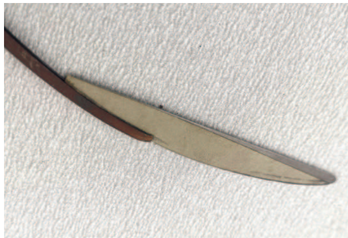
Sharpening tool in use, note they cut one wing at a time so two passes are needed on each grit
