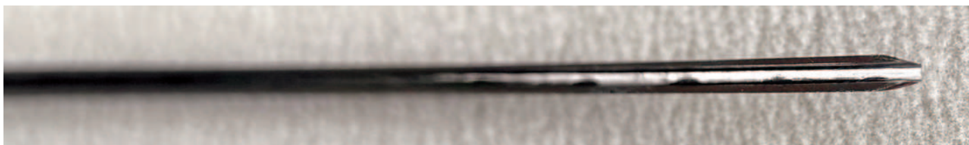
Cleaned up inside bevels
