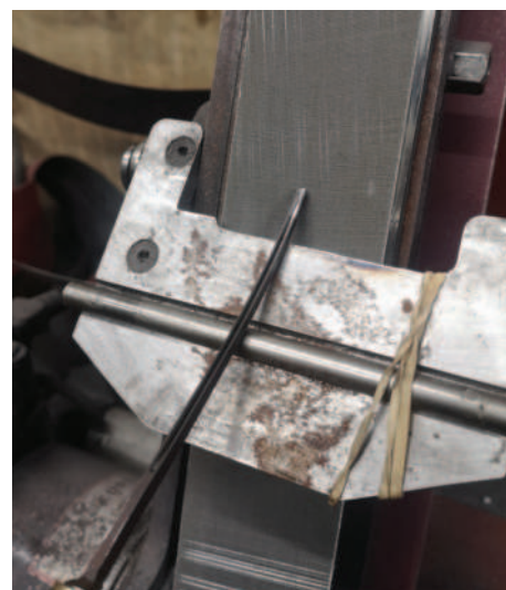
Grinding the bottom of the tool- note steel rod in place, also as this section is thicker this bevel will be longer
