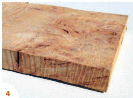
4 Knotted areas often go deep into the wood and are honeycombed with splits, hollows, bark inclusions and soft wood
