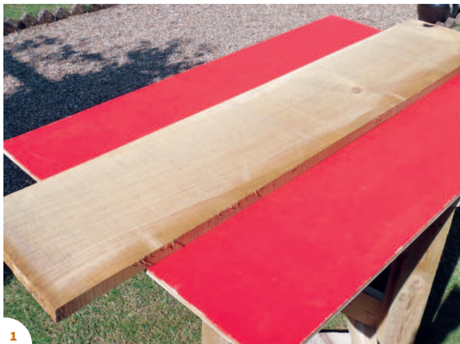
1 This is a good flat 'green oak' board from an estate sawmill with fairly straight grain and only one small knot
