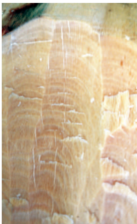
Often a test cut will show up edge dependencies that are not easily seen on the tool itself
