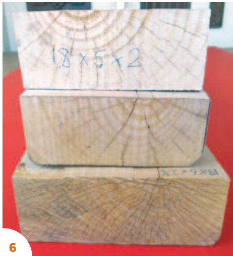
Thicker timbers will usually show shrinkage shakes at the ends, even when sealed, so cut off and discard the ends before use
