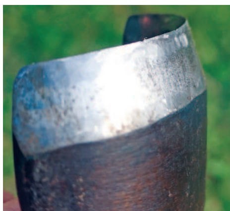
Nicks in the edge—in this case the edge damage was plain to see
