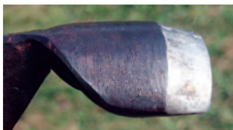
Ridge formed by the back of the bevel that needs to be removed
