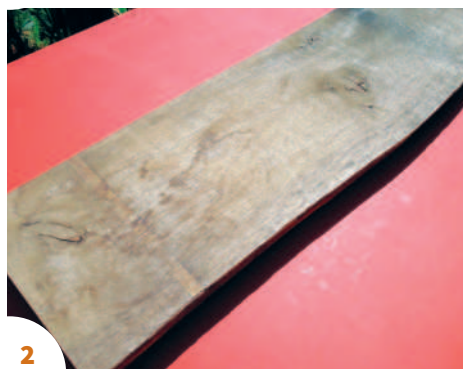
2 This oak board has noticeable knots and shakes in several places and only one-third of it is usable for carving
