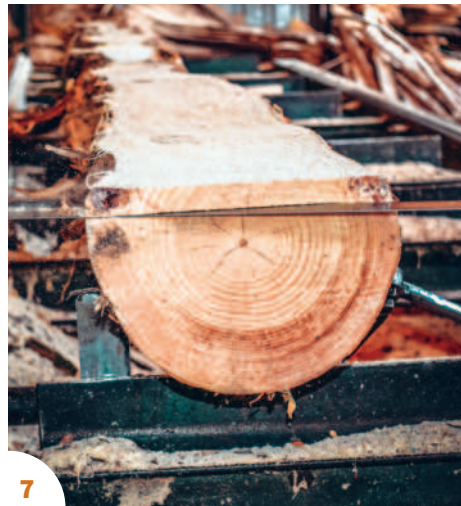
Most boards are cut straight from the circular trunk, working from top to bottom, so the radial grain varies in each board
