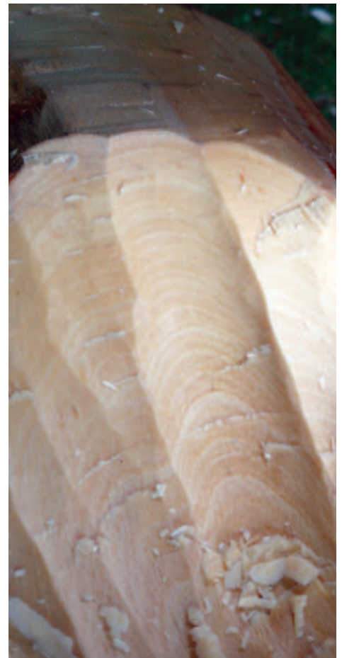
A marked improvement in the cut after sharpening!
