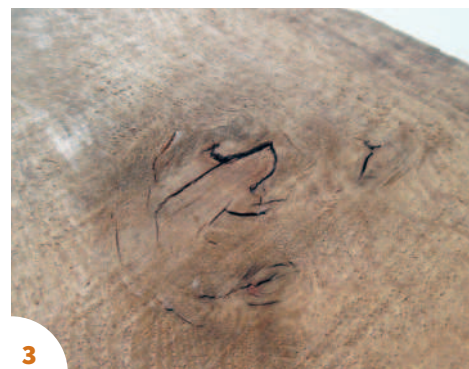
3 Knots tend to have deep splits and very distorted grain, which would disfigure a carving
