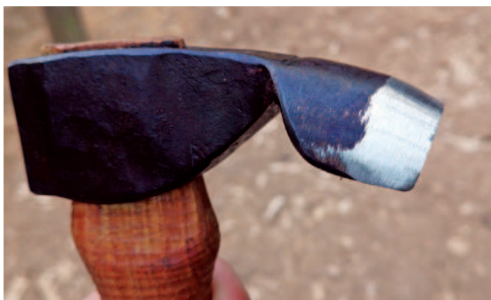
Back of the bevel blended in without altering the edge angle
