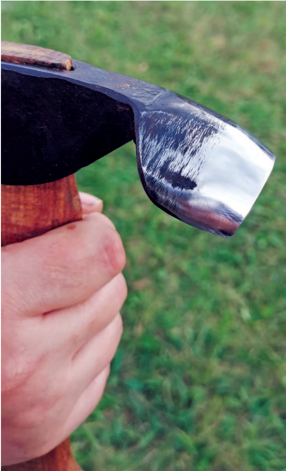
The polish is nice but incidental really, the smoothed outline helps the adze to hollow efficiently
