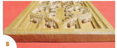
The radial grain on this board is mainly at right-angles to the surface, minimising distortion on this flat Gothic panel
