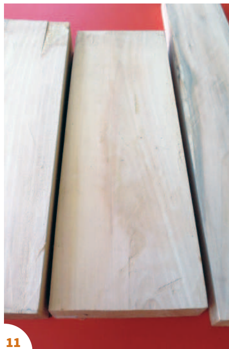
Many pieces of wood differ in colour, even from the same tree, as in these lime wood sections
