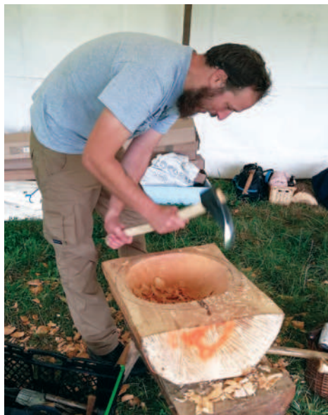
Even a perfectly set up adze won't feel good if the bench is the wrong height for you
