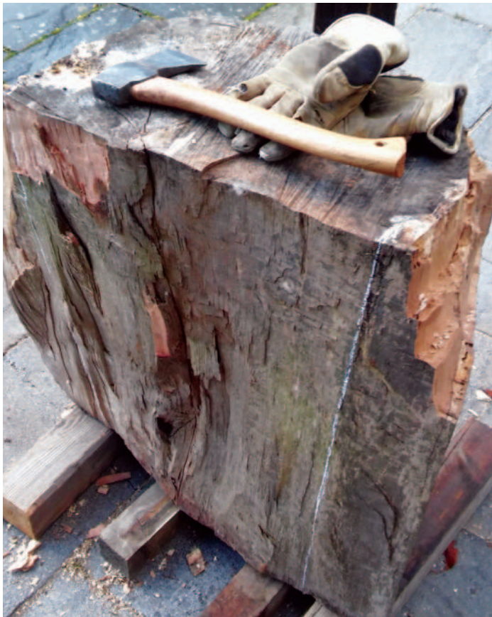
Roughing-out with an axe
