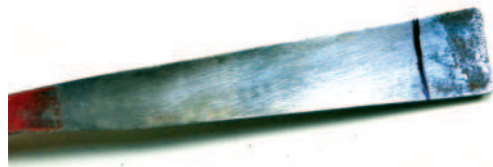
The end is useless but can be cut at line to form good tool
