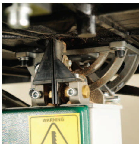
The guides under the table are hidden by safety guards which make access to the guides rather restricted. Note the lockable table tilt trunnions behind
