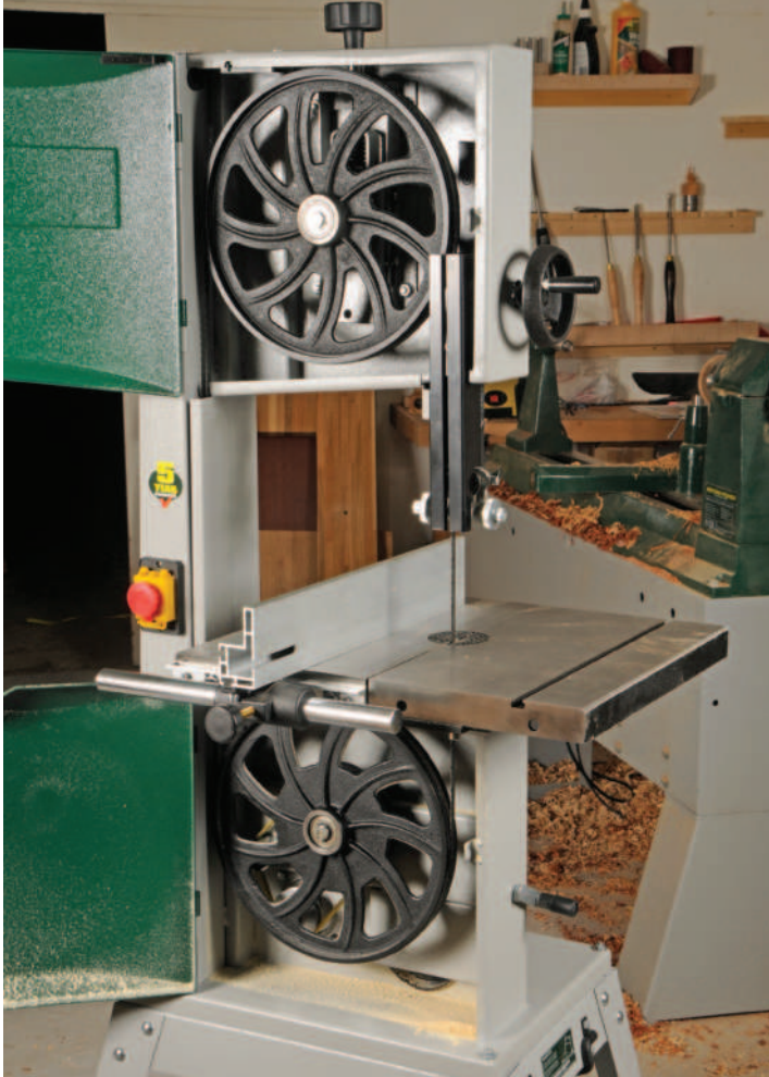
Typical bandsaw case interior design. The drive belt for the bottom wheel has a tensioning handle to ensure it is always running correctly. There are safety microswitches on both doors
