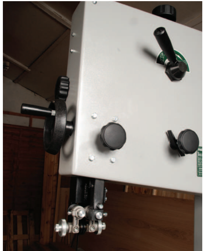
The rear of the case has the tilt and lock for blade tracking and a lock knob for the rise and fall blade guard. In addition there is a quick release lever for detensioning the blade
