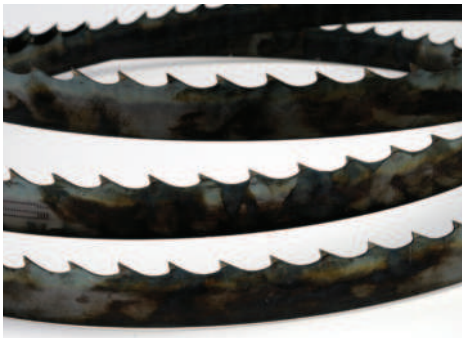
Blades come as standard tooth, skip-tooth with a gap between teeth as seen here or coarse cutting raker teeth. Skip-tooth is the standard type for all except for thin ply or very deep cutting; more on this in the next issue
