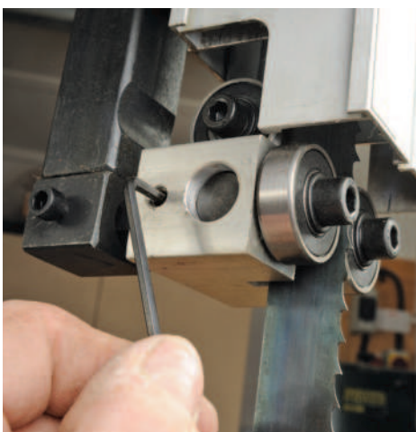
This more expensive machine uses roller bearing guides; some cheaper machines just use solid hardened blocks, although these may be substituted with replaceable hardwood blocks instead
