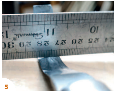
Bevel completed but not flattened
