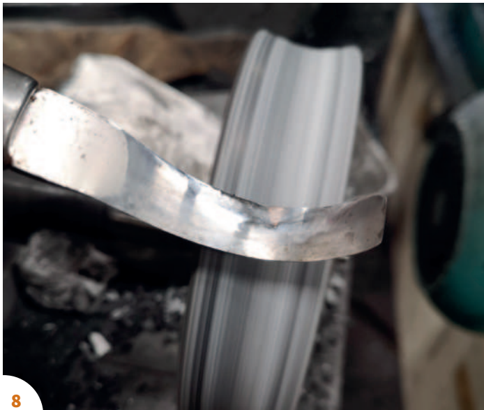
Polishing the outside on a bench grinder
