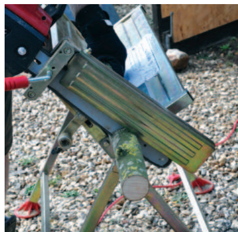
This system has the chainsaw bar securely clamped and guarded until cutting through timber. If the left hand is kept within the trestle area it cannot contact the chain
