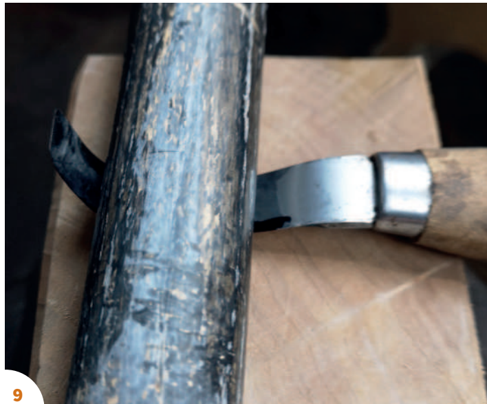
Polishing the inside – using a marker pen to show me when I had reached the edge
