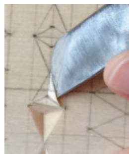
Remove the second chip with another angled cut
