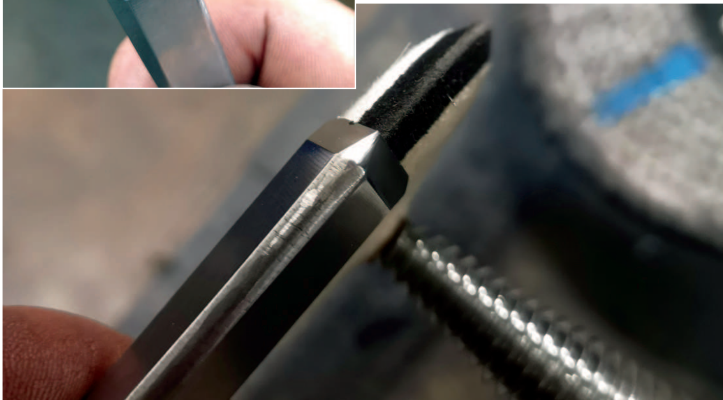
Stropping with shaped felt
