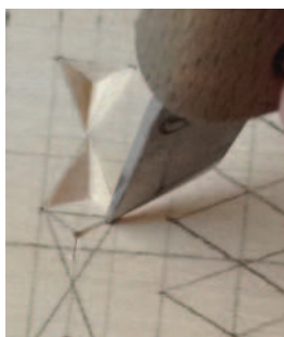
Now complete the two shorter stop cuts
