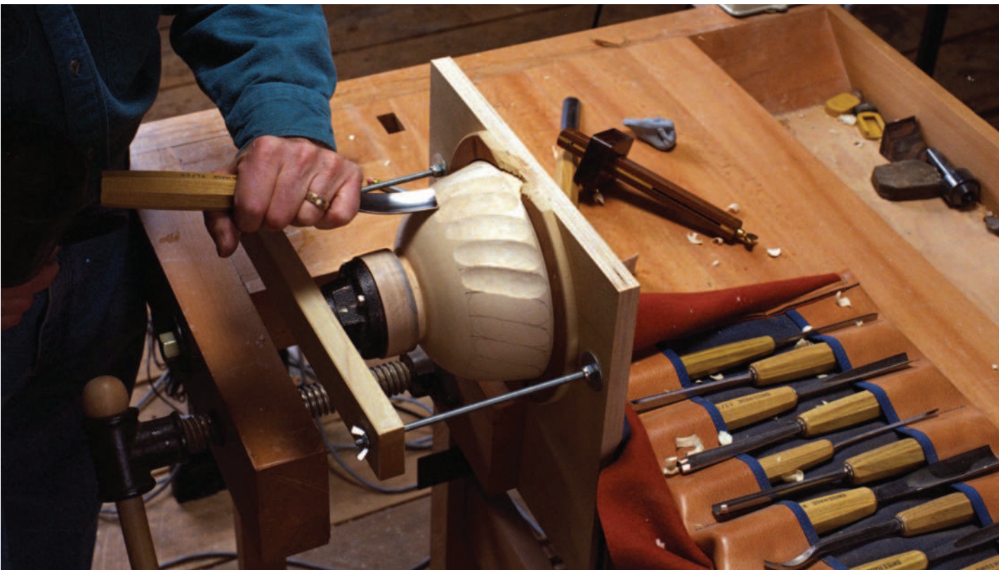
While you can build a fancy vice you can usually make an available woodworking vice work in conjunction with a homemade bowl-holding clamp
