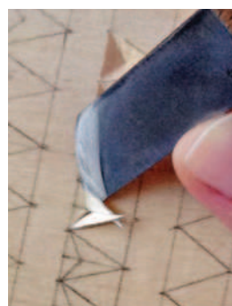
Rotate the board and undercut the second chip
