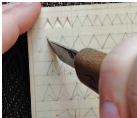
...then lower the heel of the blade along the pencil line to the base of the triangle
