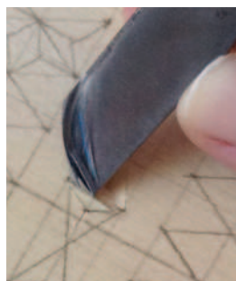
Remove the chip at the base with an angled cut of 45°
