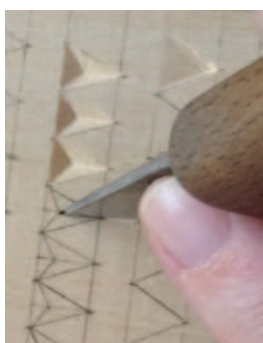
Put the heel of the blade at the centre of the triangle and lower it along the line to the top of the chip
