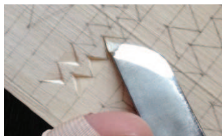
Place the knife at the edge of the triangle at 45° to undercut the first chip
