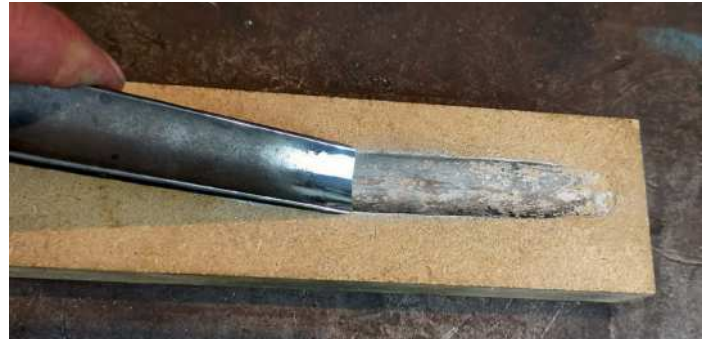
MDF strop for a gouge. The white compound has been quickly blackened by the metal it has removed
