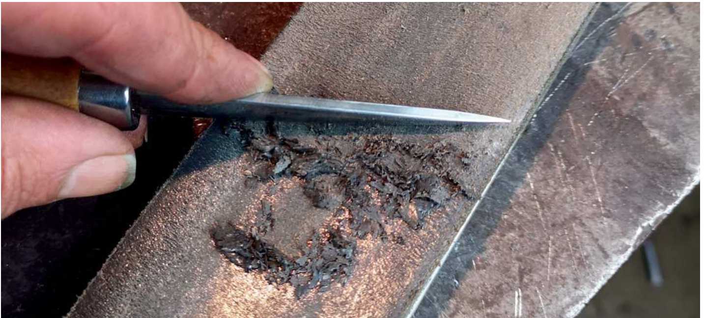
Cleaning a glazed strop. I use an old knife, but a paint scraper is also very effective
