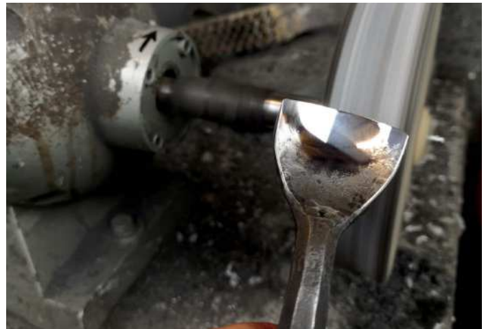
Buffing the outer bevel on a gouge. This is slightly convex so a larger wheel is used. With pressure this will deform slightly to follow the bevel
