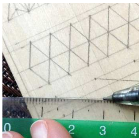
Diagonally connecting all the dots and then (INSET) finding the deepest point of the triangles
