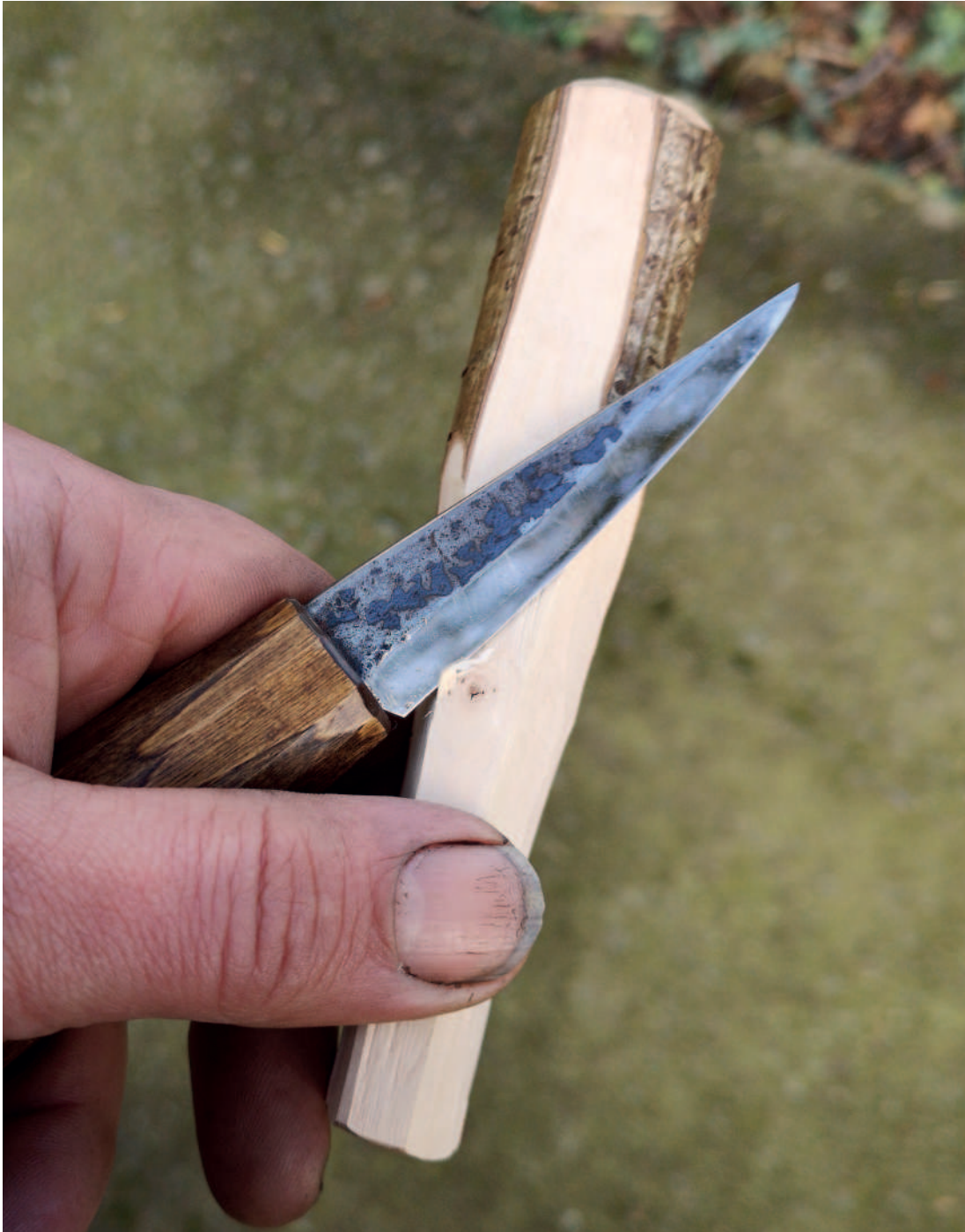
A skewed cut and a gentle touch may allow you to get past tricky areas without damaging your edge
