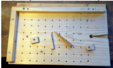
A more advanced bench-top carving station. This consists of a lower board with a second one on top secured by a single wood screw in the centre to allow it to swivel. A series of holes, wedges and pegs hold the work and it can be swivelled for carving or to use the fretsaw peg
