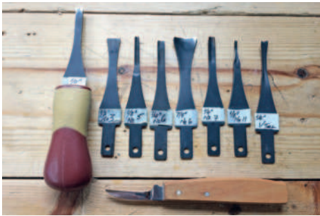
A suggested starter kit. These tools are by Flexcut and are readily available. The blades just push into the handle and so can be stored in a small roll or toolbox. The knife is a general carving knife
