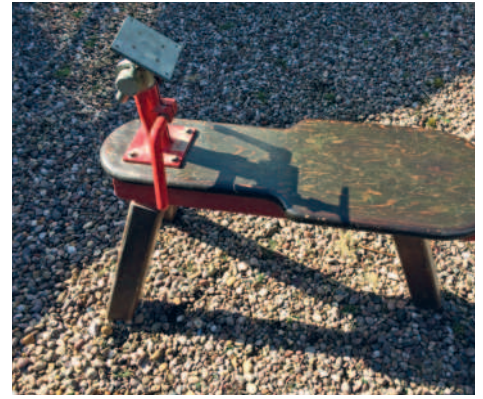
Another solution is a sit-on carving bench, this is a professional one by the Austrian company Stubai. I have seen many homemade versions of these benches, including some that fold up for storage and carrying
