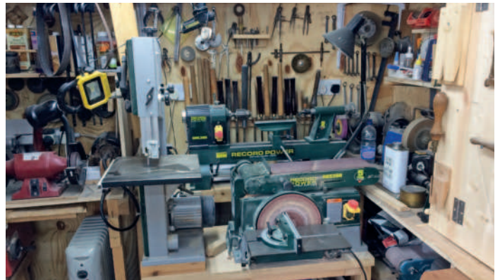
The bandsaw and sander on a moveable base with locking castors. I have to move this to get to the lathe
