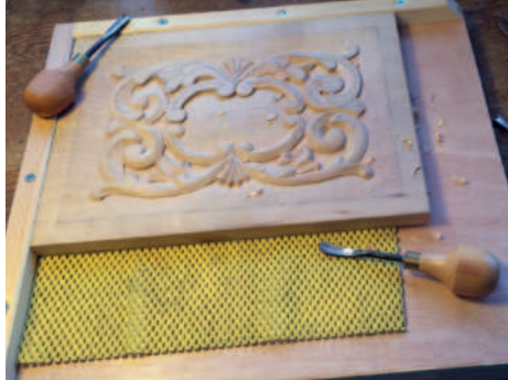
Simple bench hook with added side bar to stop work sliding. We usually start beginners with one of these in our carving club
