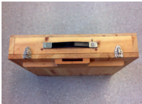
Another version of a work station. This one is a completely closed carrying case. Note the bar underneath, which acts like a bench hook, and the slot for the fretsaw peg
