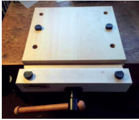
This is an interesting bit of kit that I found recently. It is produced by the famous Swedish maker Sjöbergs. It can be clamped on to any table or desk and can either hold work in the vice or between the dogs
