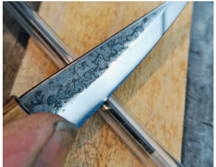
By pressing down firmly and rotating the edge into the Biro you should be able to see the edge deflect
