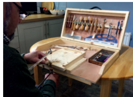
The carving block turned to allow the fretsaw to be used on the V-peg. You don't actually need a scrollsaw
