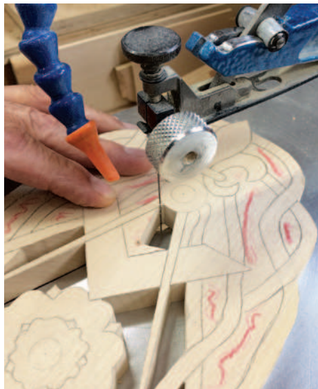
Removing the marked areas on the scroll saw
