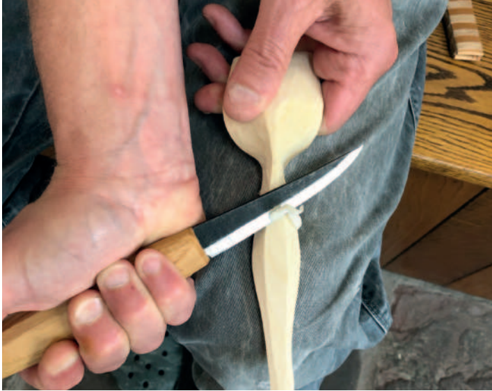
Using the reverse forehand grip to create a smooth, planed finish on the back of the handle
