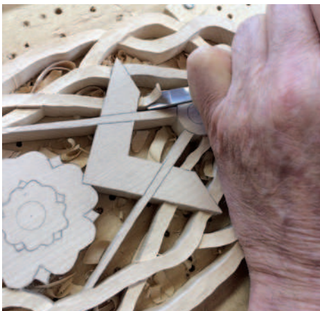
Carving down the levels between the geometric elements of the design
