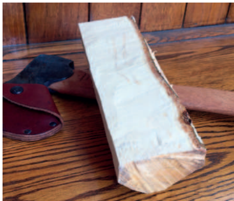
The cleft section is cleaned up and rough-shaped to a 'billet'
