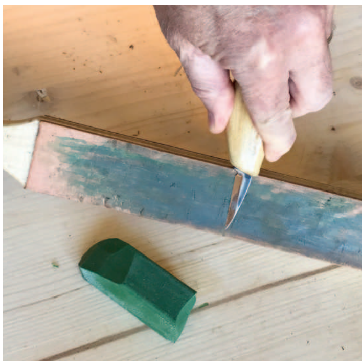
Make several passes on a leather strop charged with a honing compound. Hone both sides of the knife equally
