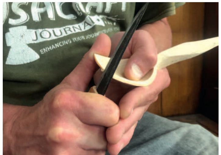
The reinforced thumb joint grip to carefully trim the end grain profile at the leading edge of the bowl
