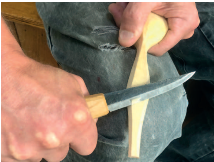
Using the off the knee grip to remove excess material from a handle end that is too thick
