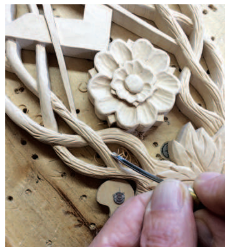
Creating the barked effect on the branches using a curved V-tool
