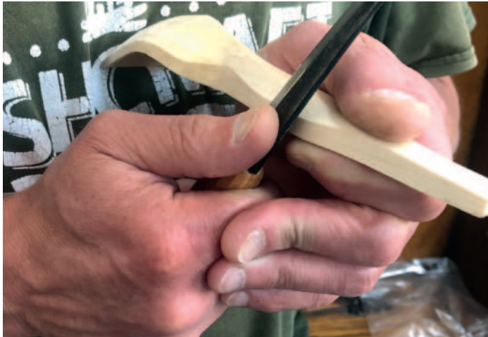
The reinforced pull stroke is useful for working the sides of the handle down towards the back of the bowl
