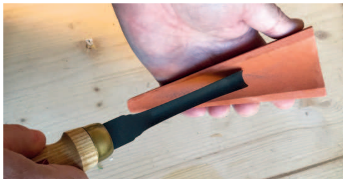
A curved slipstone can help sharpen the edge of a gouge
