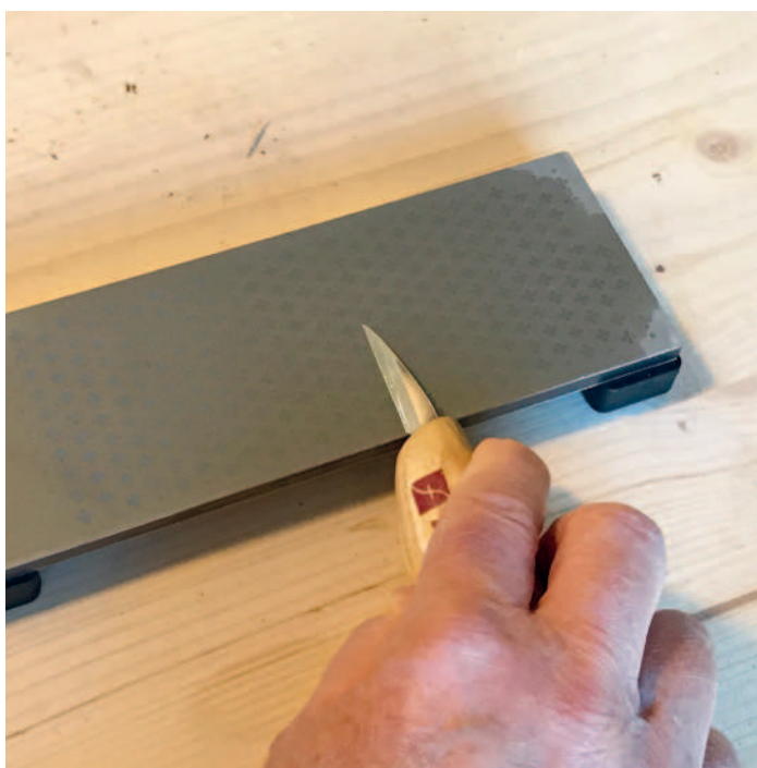
Try to match the knife's original bevel angle and push or pull the blade away from the cutting edge
