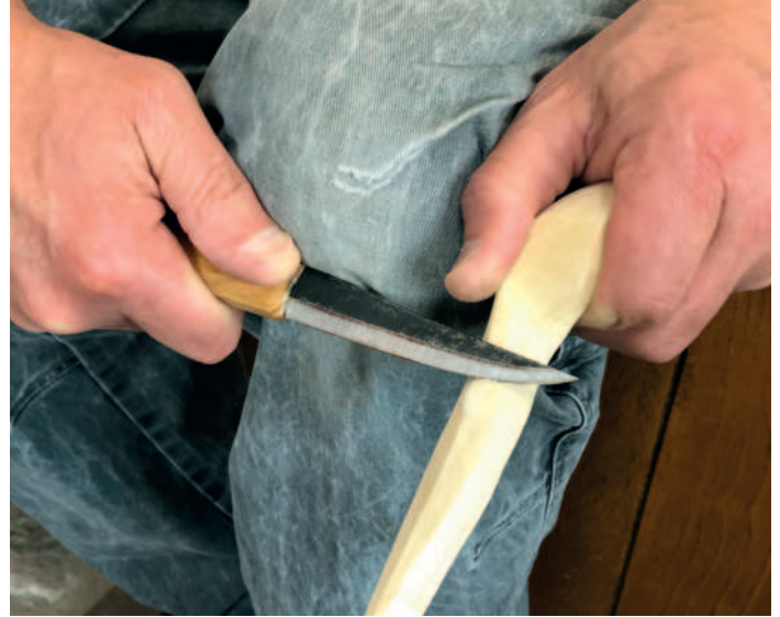
I like to use the knee brace grip to create smooth facets that make up the cross-sectional profile of my handles
