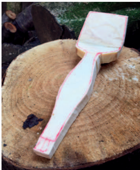
The spoon blank roughed to shape with the axe, working as close to the profile as your skills allow
