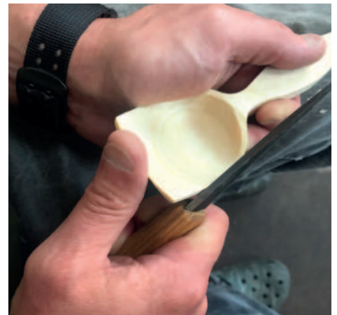
The results of using the thumb joint grip effectively
