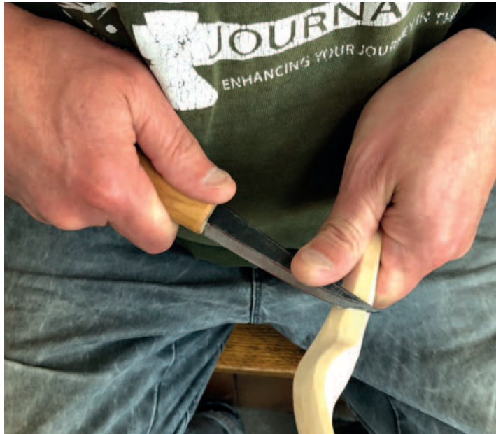
The thumb push excels at dealing with changes in the direction of the grain and is especially useful for this area in the 'neck' of a spoon
