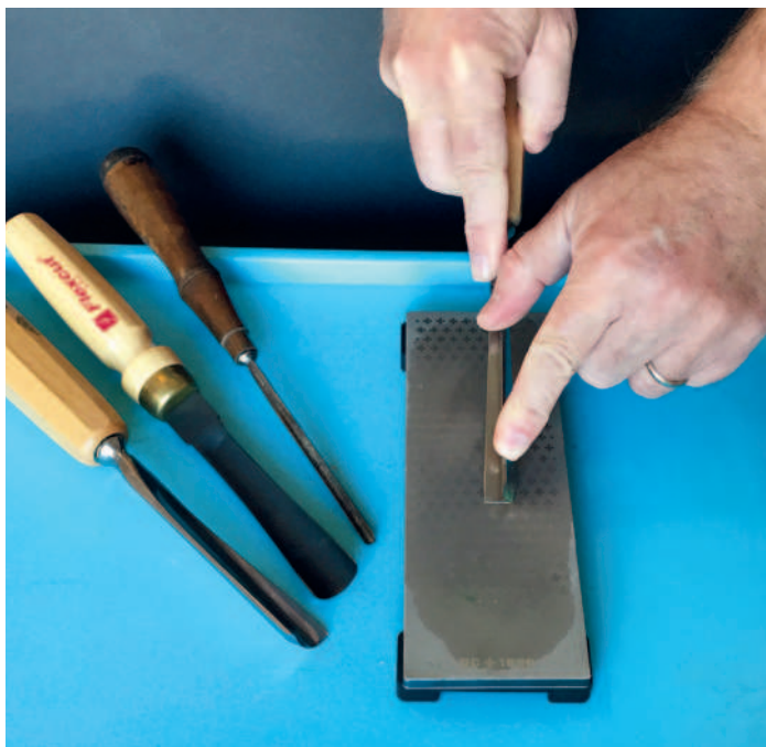
Lay the bevel of the V-tool flat on the stone and draw it towards you, making several strokes
