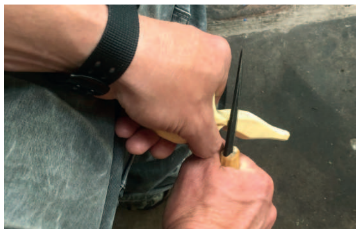
The drop-shoulder forehand grip is more powerful and removes material quicker but with less control
