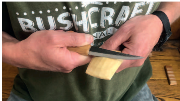
The chest lever grip works well for both the front of the bowl and the back of the handle, always carving downhill
