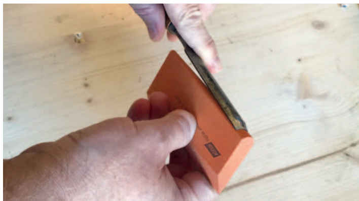
A slipstone with a convex edge can remove the burr on out-cannel gouges or hone the bevel on an in-cannel gouge
