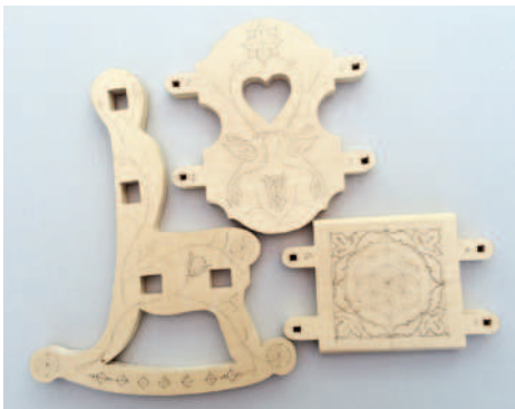
The components cut out on a scroll saw and the chip carving design drawn on
