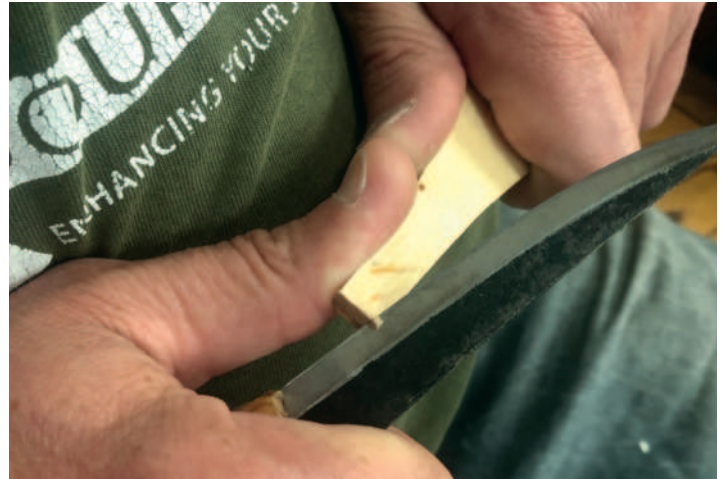
The draw grip makes short work of trimming across the end grain at the end of the handle
