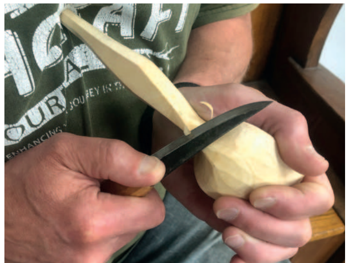
The simple pull stroke (the un-reinforced version) for working a clean cut from the deepest part of the back of the bowl down the entire length of the handle
