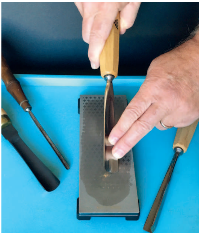
As you pull the gouge towards you, start to roll the cutting edge to the opposite side while maintaining the same bevel angle
