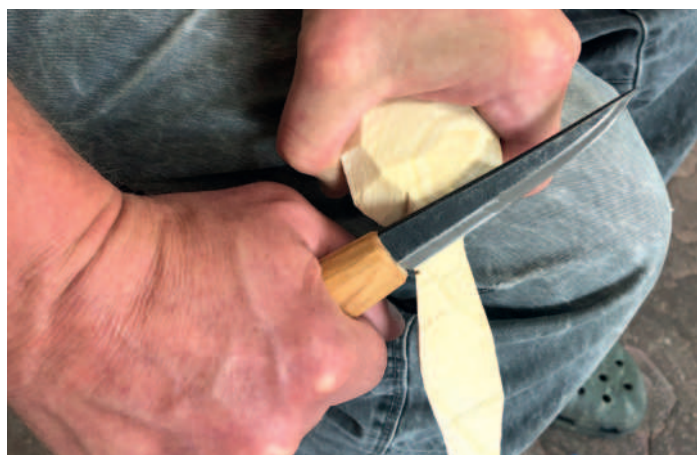
Using a skewed forehand grip to effectively remove material from the back of the handle
