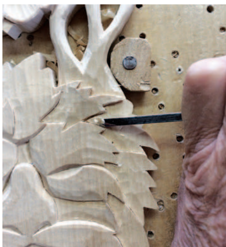
Carving the face required very fine skew chisels
