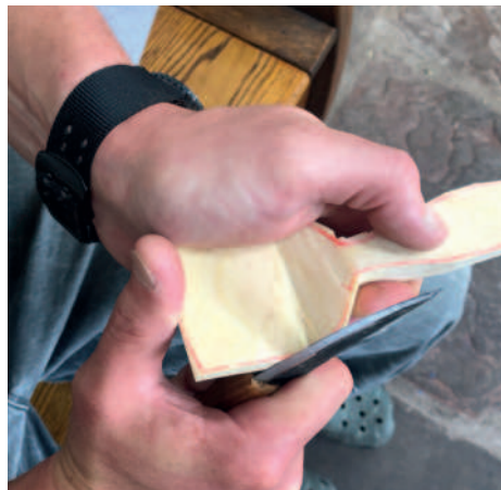
Using the thumb joint grip to take the edges of the bowl to a finished smooth profile
