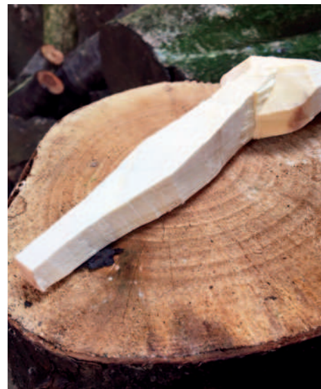
The back of the blank is also roughed out to profile with the axe
