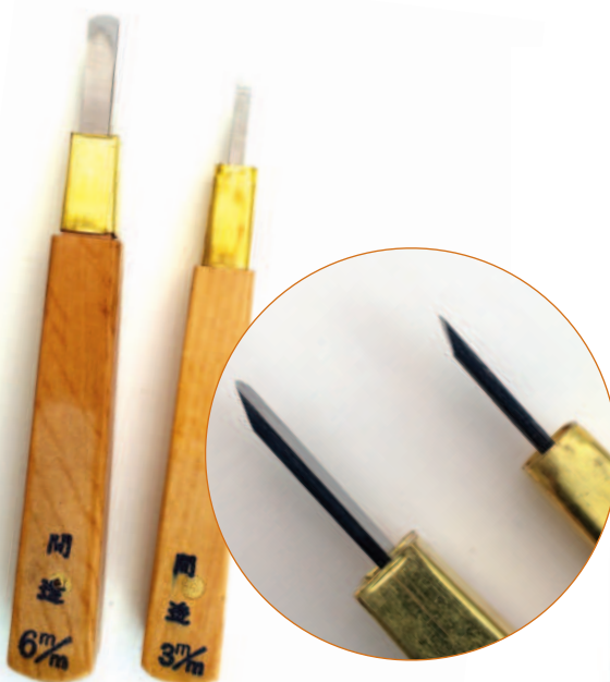
The aisuki. This tool has the profile of the flat chisel but ground with a curved end. The aisuki is used for very shallow carving and has the advantage of the corners not digging into the work
