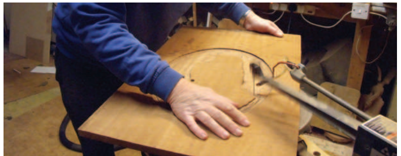
Using a scrollsaw to cut out the internal waste section
