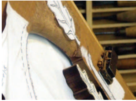
Rounding over the inner edge and progress on the relief-carved tree
