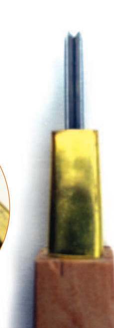
The sankaku-toh, a V-tool which also has an extending blade
