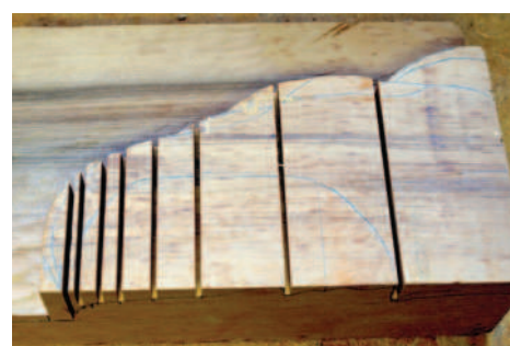
Extend the depth cuts across the width of the section to be cut
