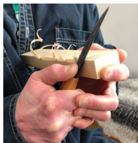
Reinforced pull stroke – observer's view
