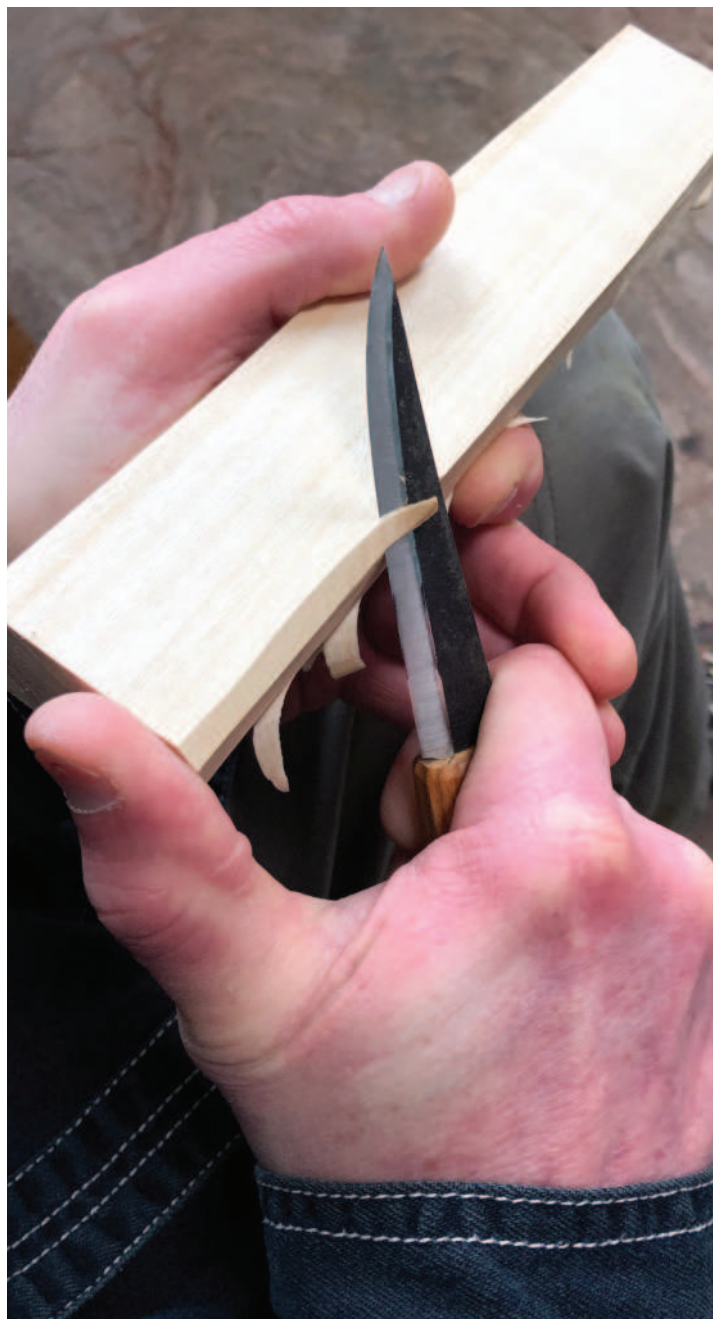
Reinforced thumb joint grip – carver's view
