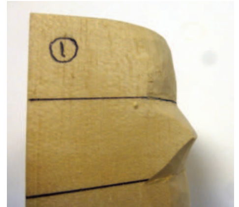
Cut back to the middle line to create nose slope, angle down to next section. Round off the corner as shown
