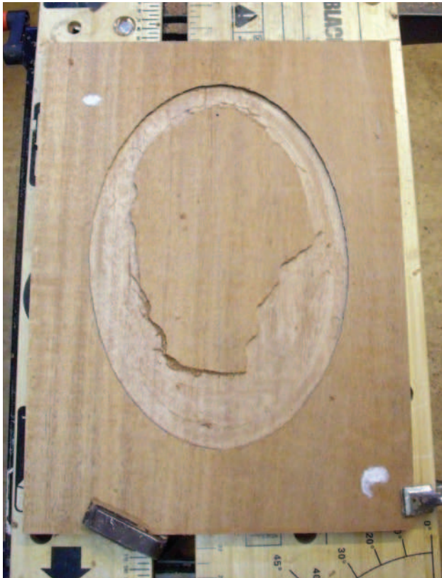
The back of the mirror routed out to take a 4mm thick mirror
