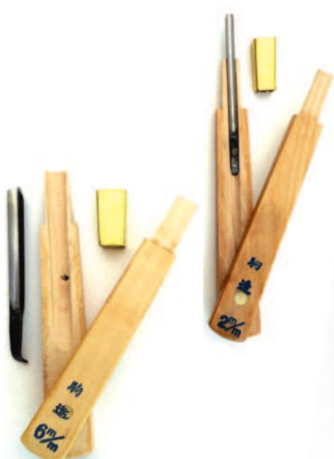
The komasuki opened to show its component parts
