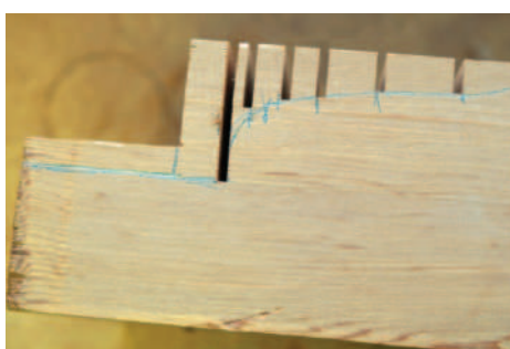
Cut to depth on the edge
