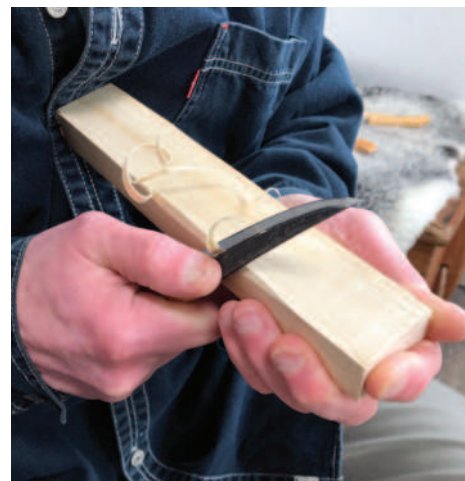
Simple pull stroke – observer's view
