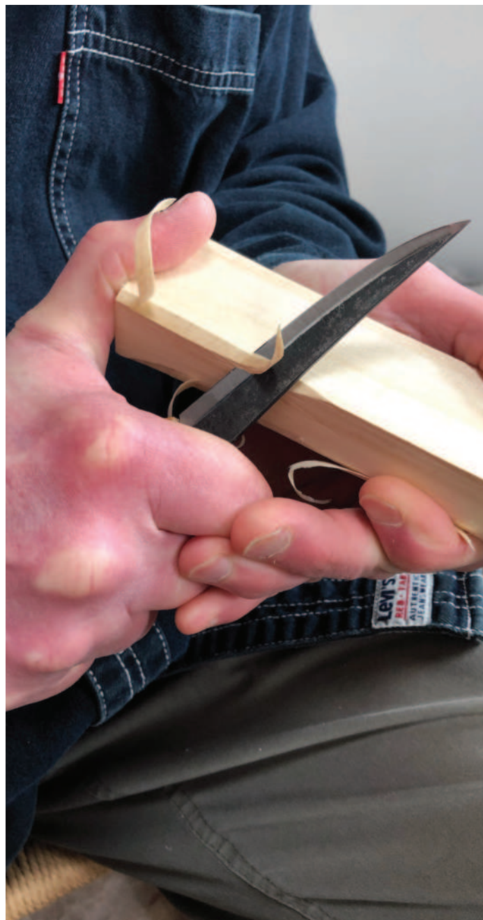
Reinforced thumb joint grip – observer's view
