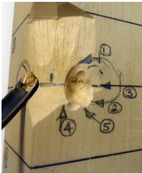
Direction of the five cuts to be made with your gouge
