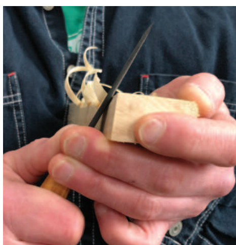
Reinforced pull stroke – on spine of knife
