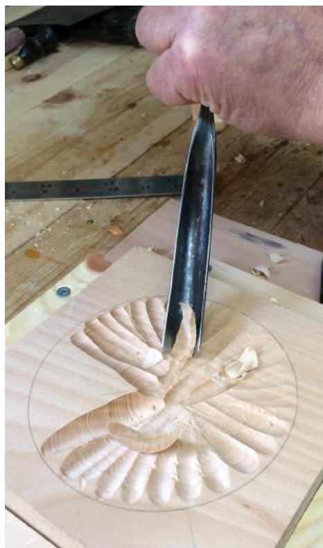
Carving out the bowl in a simple jig made from the scrap box
