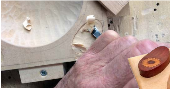
Removing the bulk of the recess with a shallow gouge
