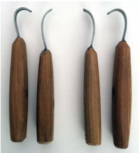
Four knives by Ben Orford, two right-hand and two left-hand, or push and pull as I prefer to call them
