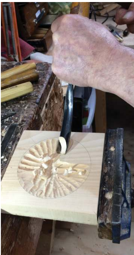
Roughing out the bowl with the old No.11 gouge that I didn't know I needed
