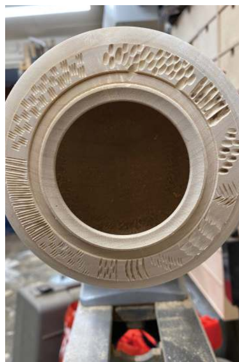
Creating various textured detail with the small cutters
