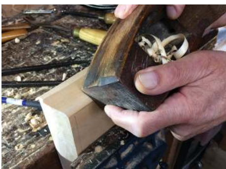
Shaping the side of the bowl using an old wooden smoothing plane bought at a car boot sale
