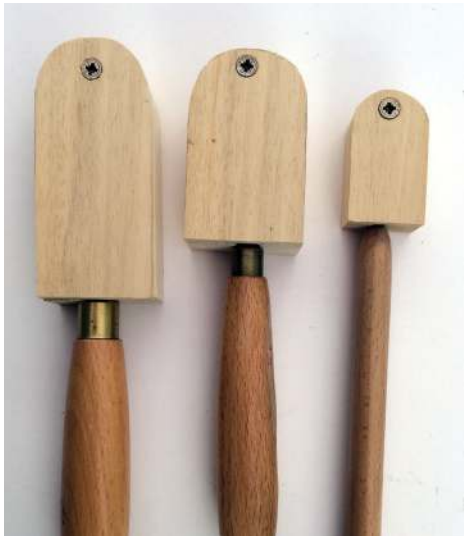
The protective covers in the closed position
