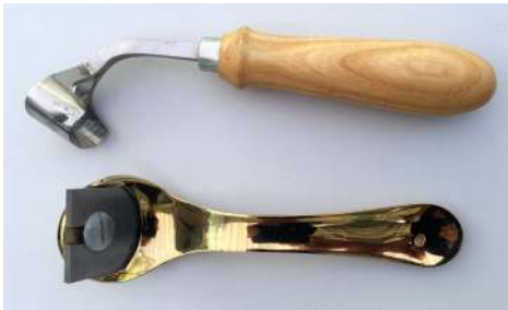
The scorp (above) and the pull plane (below)
