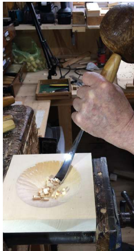
Refining the deep gouge marks with a No.6 bent gouge
