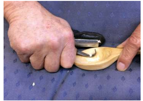
A spoon bowl being carved using the homemade protective stall and resting on a cushion
