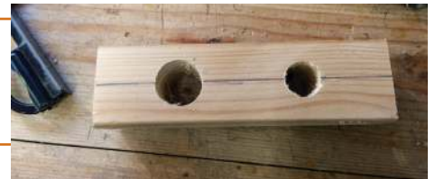
The drilled timber ready for splitting to make a simple swage block
