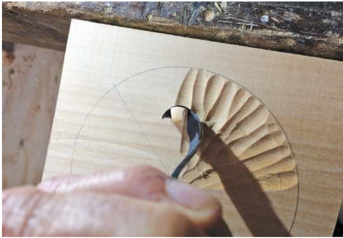
Starting the bowl with a deep curve knife
