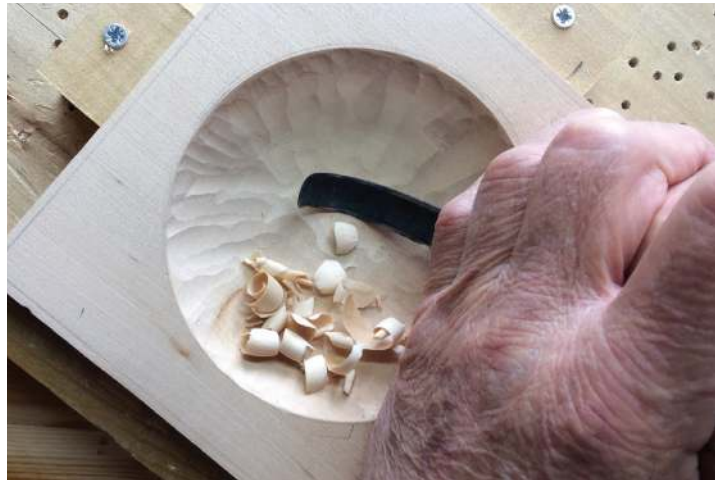
Using a shallower curved blade to smooth out the bowl
