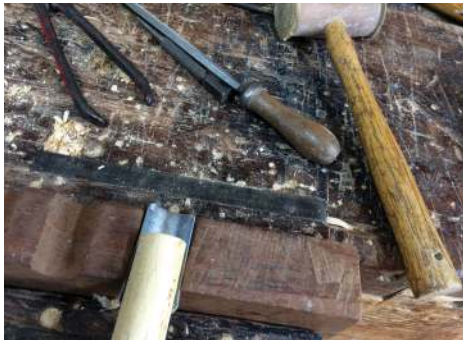
Curving the aluminium sheet in a swage block made from wood
