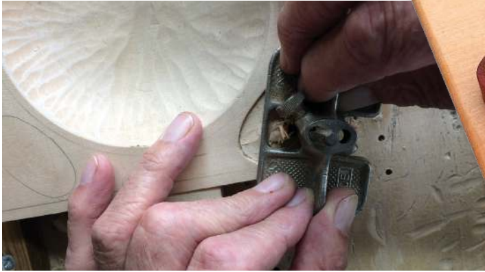
Using a small hand router known as an 'old woman's tooth' to level the base of the recess
