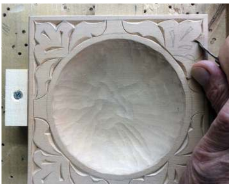
Chip carving the corners of the bowl
