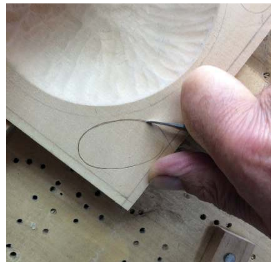
Setting in the recess with a knife
