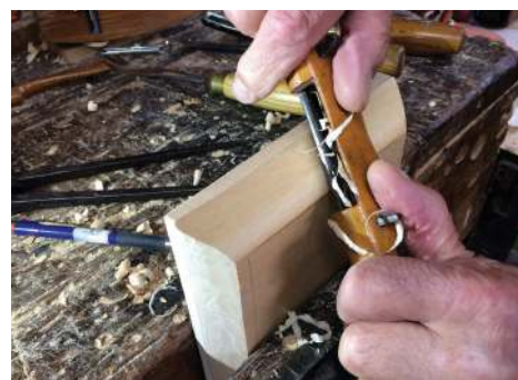
Rounding off the edges using an old wooden spokeshave
