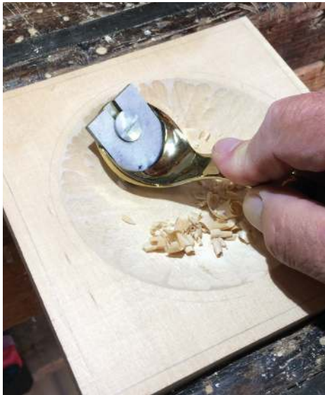
Smoothing the bowl with a curved blade pull plane
