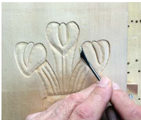
Modelling below the surface with a Gonzales hook
