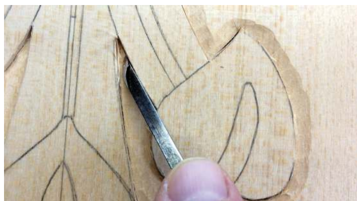
Getting into a tight corner with a small skew chisel made from an old needle file
