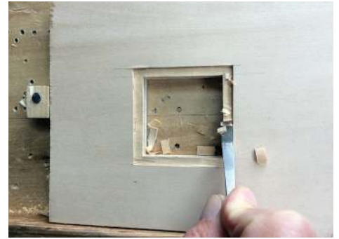
Carving down the rebate using a dog-leg chisel
