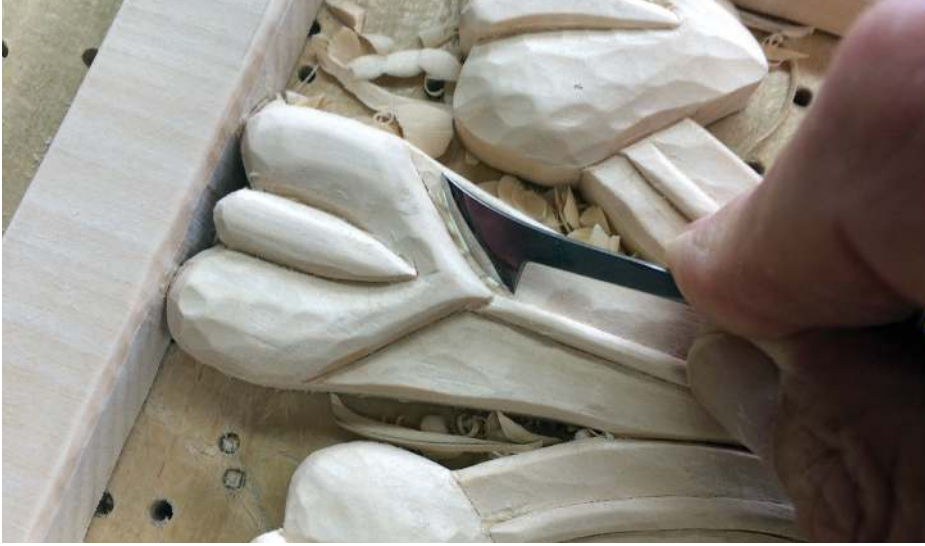
Cutting in with a hook knife – it is ideally suited to this task RIGHT: The pierced panel
