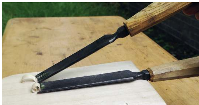
Angle of attack for in and out cancell gouges. Note out cancell gouge is so flat that the handle will foul the work
