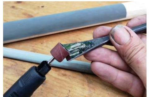
Various ways to set the inside bevel – slips, abrasive paper on dowel, multitool or flexidrive mounted sanding wheel
