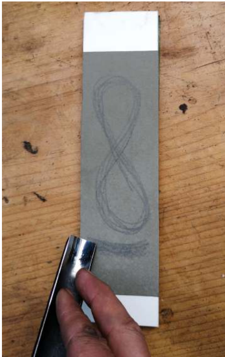
Setting the outside bevel, figure of 8 or rocking motion (shown)
