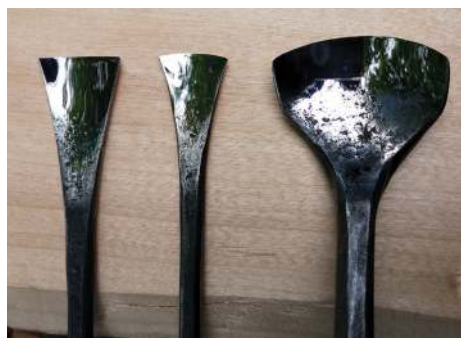
Three plan forms of gouge. L-R straight, bull nose and softened corners
