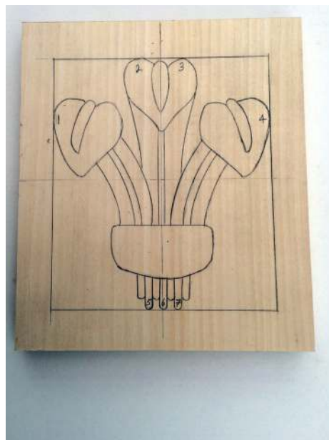
The pierced panel set out showing the seven contact points
