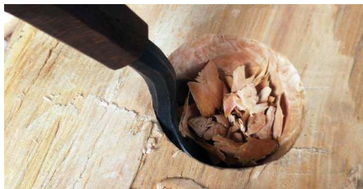
A steep AOA allows for deep forms to be hollowed
