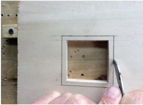
The pierced aperture with the rebate marked on the reverse side. Setting in with a knife
