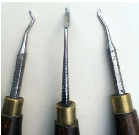
Small tools made from dental probes. They are left, right and straight cutters
