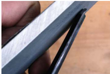
Setting the outside bevel, alternate method
