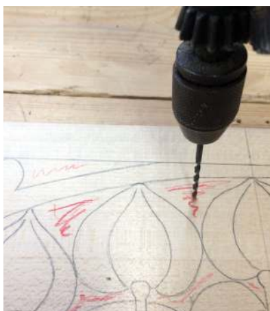
Drilling a hole for piercing
