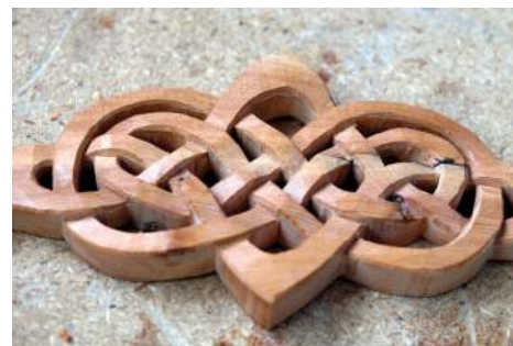
Here are the completed chamfers
