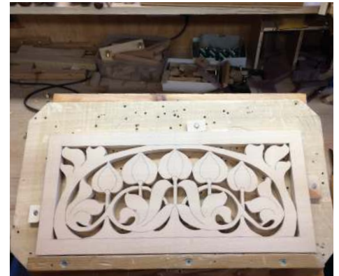
The pierced panel held and ready to work on
