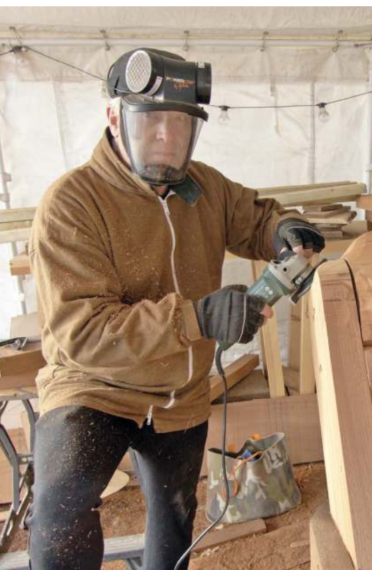
Working on bigger projects often means working with power tools using Arbortech and Saburr cutters and full safety gear
