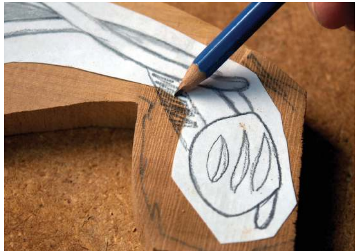
If required, mark in the sections needed for additional strength
