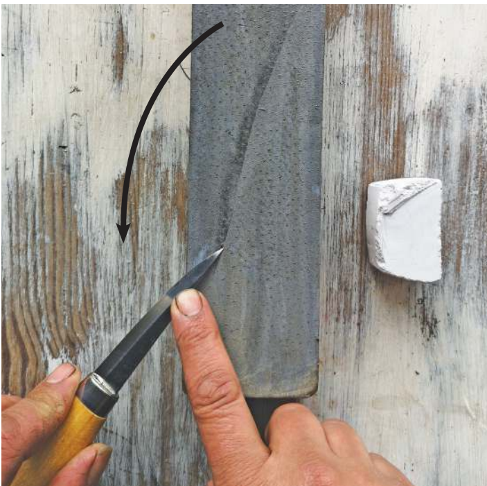
White polishing compound on suede, the black streaks are the steel it has cut from the blade
