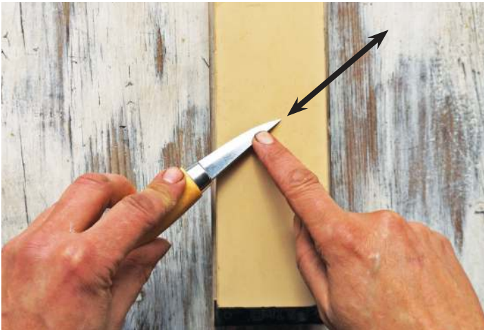
Stab sharpening. This can be an easier way to keep the bevels at the tip flat
