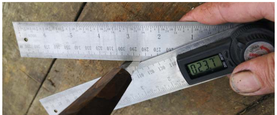
Measuring bevel angle with a digital angle finder
