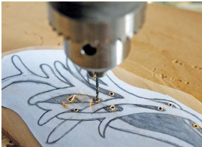
Drill out the inner sections with a fine drill bit ready for cutting with a scrollsaw
