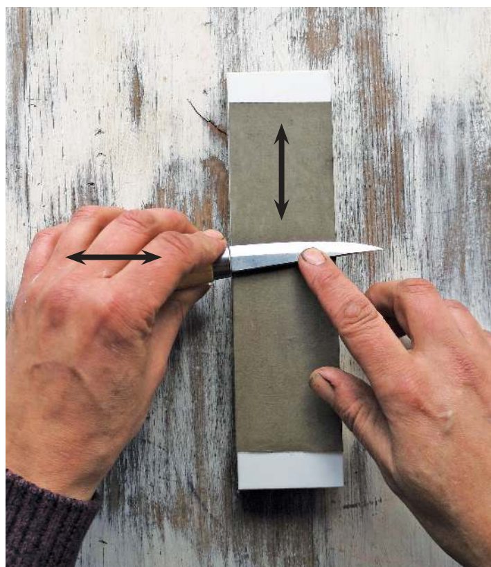
Concentrate on keeping the bevel flat and work the blade up and down the stone, while also moving the blade laterally so the full length all the way to the tip is worked on
