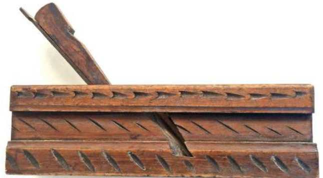
A moulding plane with chip-carved decoration found in a bric-a-brac shop in Zurich, for which I paid the princely sum of £4
