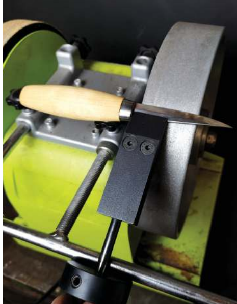
Hollow grinding a knife, using a Hewn & Hone sloyd jig
