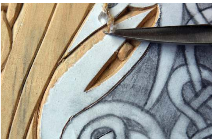
Use a knife to round over the detailed areas as required
