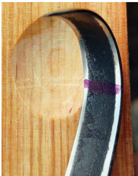
It was hard to spot the edge damage on this blade but it showed up easily in soft timber
