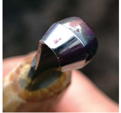
This flat ground blade is prone to chattering (making contact only on the edge and back of the bevel)
