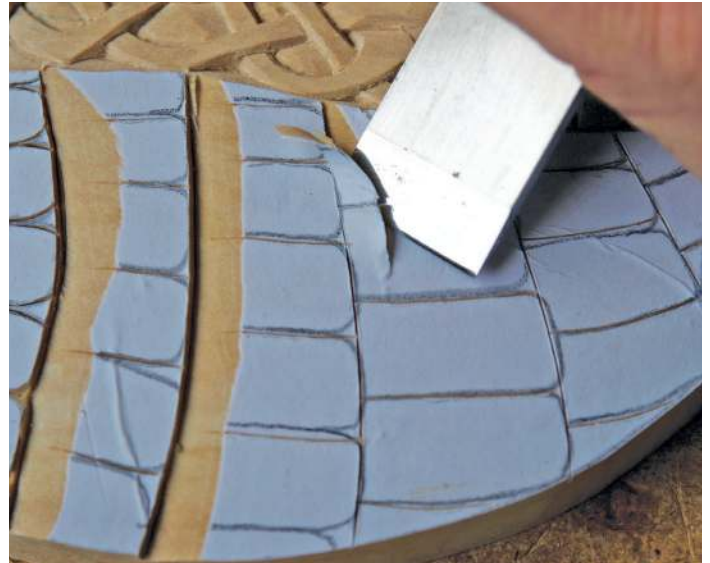
Use a number 1 straight gouge or chisel to create the angled layers
