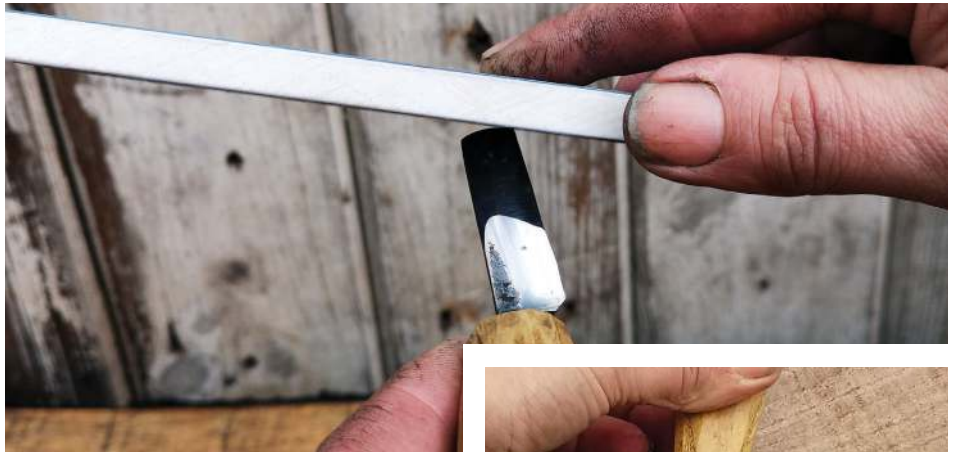
My preferred method as you can actually see the angle you are presenting the blade to the abrasive, and in this case it is focusing too much on the edge
