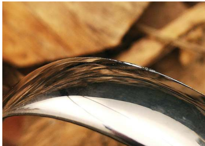
A shiny burr raised from working on the inside bevel. In my production work I use a sequence of 1200 grit, 3000 and then finish with either 7000 grit or a fine compound, rubbed directly on to a dowel
