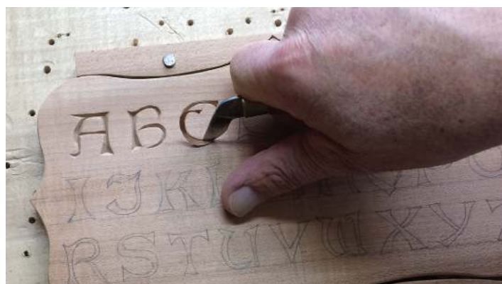
Carving the sampler using a continental-style knife. You could, of course, use a standard chip-carving knife
