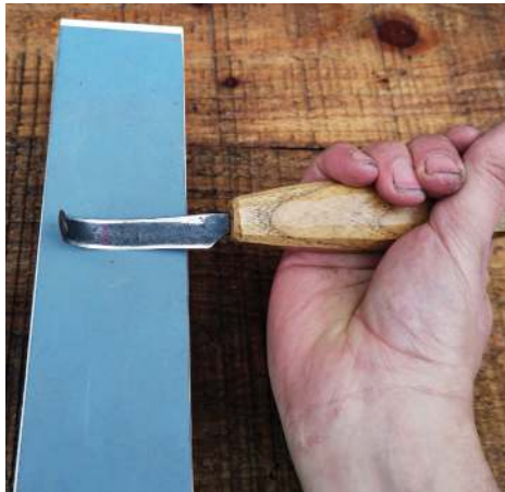
Working away from the edge with the palm up. Lifting your hand will allow you to work from tang to tip in a single, smooth motion, or the other way
