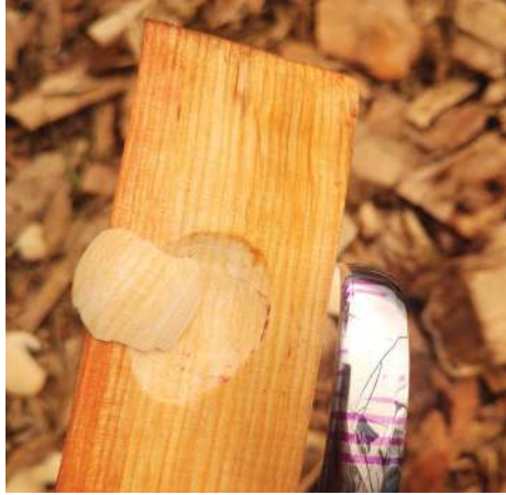
This blade profile suits this form well. There is contact along nearly the full width of the blade. Remember, you only have to do this once, if at all – some blades have very good geometry straight from the box
