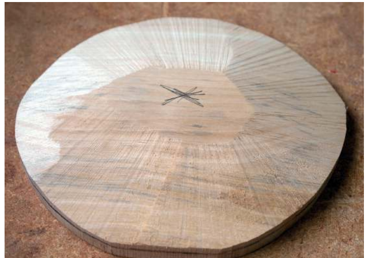
The medallion has a slightly domed face, so work this down in stages
