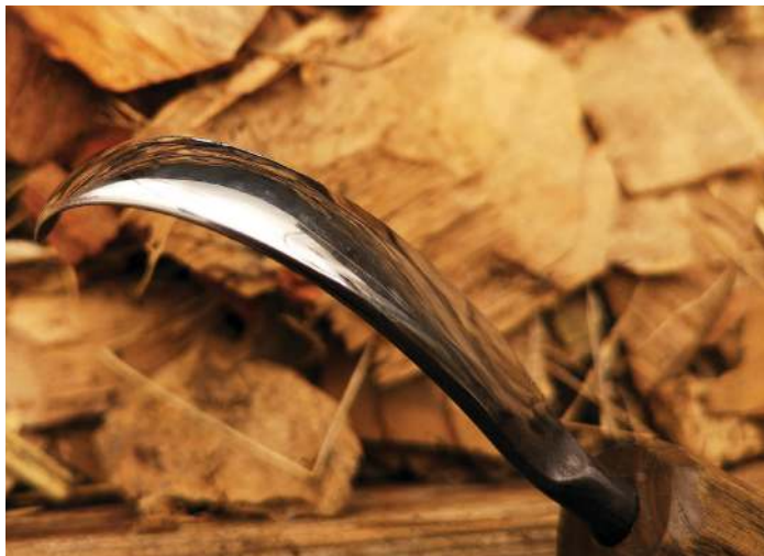
A shiny burr raised from working on the inside bevel. In my production work I use a sequence of 1200 grit, 3000 and then finish with either 7000 grit or a fine compound, rubbed directly on to a dowel
