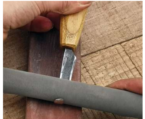
Using wet or dry on a dowel to refine the inside. Work the paper away from the edge to avoid cutting into it
