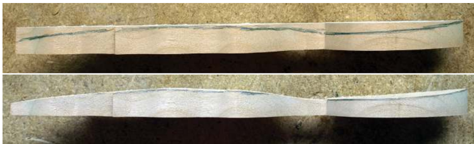
Roughly marked top face of the bowl and spoon curvature
