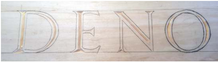
The first V-cuts on the longer sections
