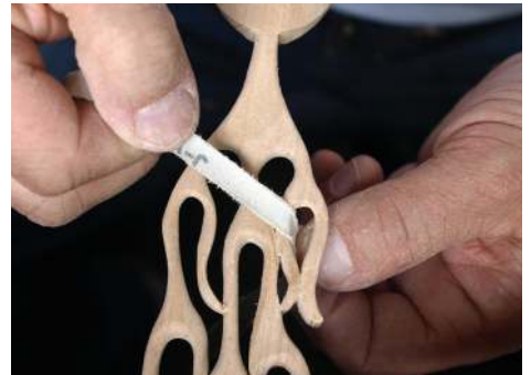
Carefully sand the flames using minimal pressure
