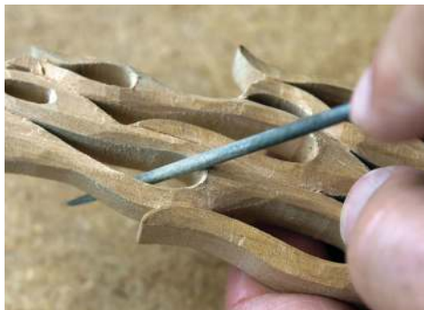
Refine the curved areas with a rasp or abrasive
