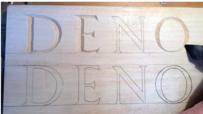
Carving the letter 'O' with the mill knife
