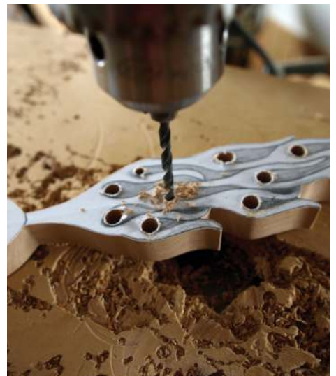
Drilling holes ready for cutting
