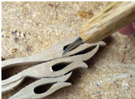
Use a knife to clearly define each flame section
