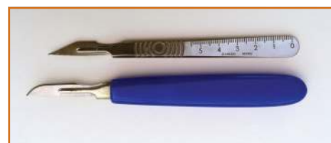
Two styles of scalpel handle with different shaped blades
