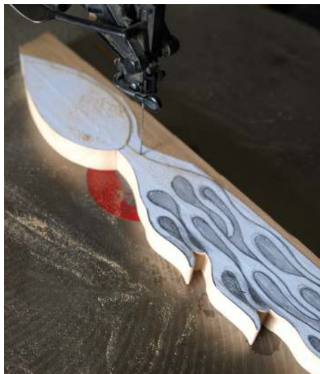
Cutting out on a scrollsaw
