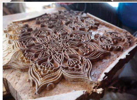
Blockwood carving for fabric printing in Jaipur, India
