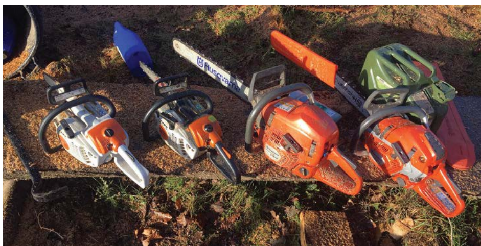
Ella’s kit equipped with both carving and conventional chains and bars
