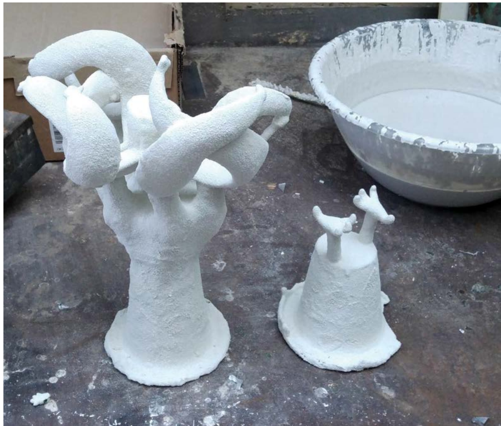
Wax tail and legs coated in a ceramic shell
