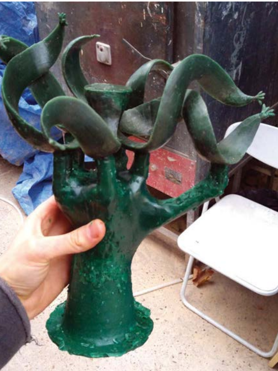
Wax mould of the tail feathers attached to wax runners and cup
