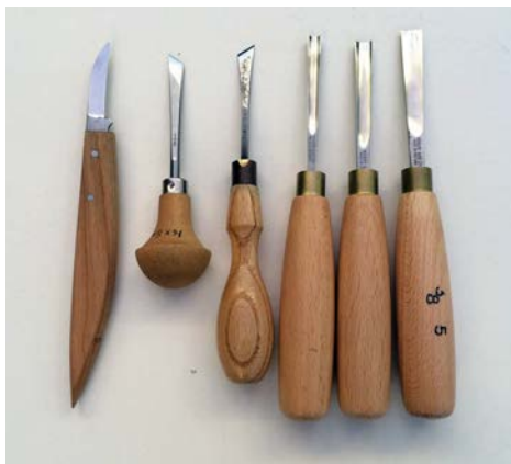
Some possible additions to your toolkit. From left to right: a straight-bladed chip-carving knife, two skew chisels, and three gouges, a No.7, 6 and 9mm and a No.5, 10mm
