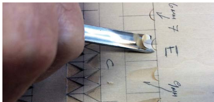
Making the slicing cut with the No.7, 9mm
