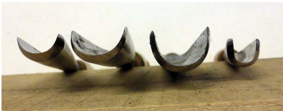
These tools, from the left, are a No.9, a No.10 and a No.11 (note the subtle difference in the sweep). The one on the right is a special with longer extensions to the sides to cut even deeper into the wood
