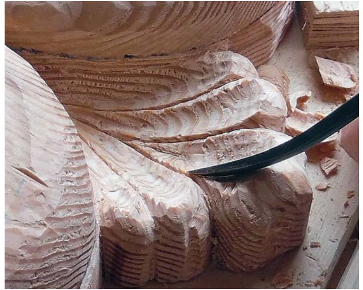
When cutting across the grain, the hard latewood crushes the soft earlywood causing tearout
