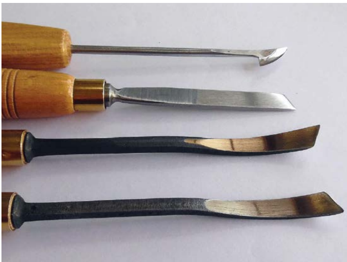
Skew chisels and gouges can slice through the grain at an angle. Top to bottom: hooked skew chisel, straight skew chisel, right and left curved skew gouges
