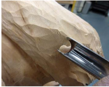
A no. 9 removing only a little wood creating a shallow cut
