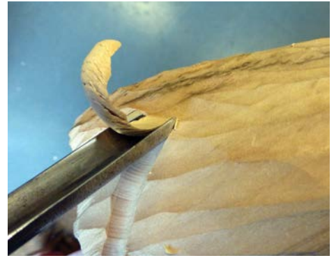
The same tool producing a very deep roughing out cut
